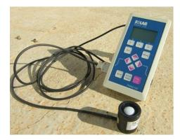
Figure 3.16. Portable UV-A radiometer.
