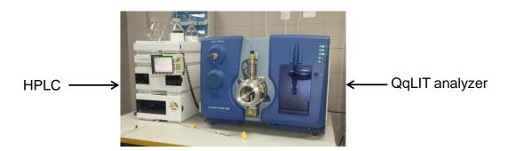
Figure 3.9. Photograph of HPLC-QqLIT-MS/MS equipment.
