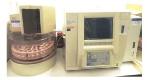
Figure 3.19. Photograph of TOC-analyzer.
