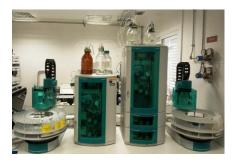
Figure 3.18. Photograph of ion chromatographs.
