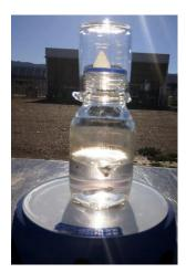
Figure 3.12. 200 mL-solar reactor exposed to natural sunlight.
