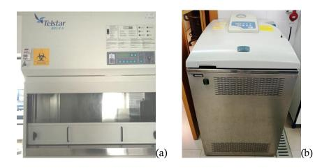
Figure 3.1. Laminar flow cabinet (a); and autoclave (b).
