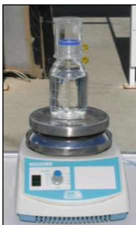
Figure 3.8. 200 mL-Batch reactor exposed to natural sunlight.
