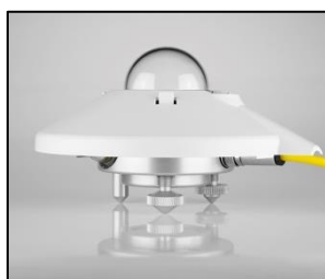
Figure 3.11. UV radiometer Model CUV4, Kipp & Zonen located in PSA facilities.
