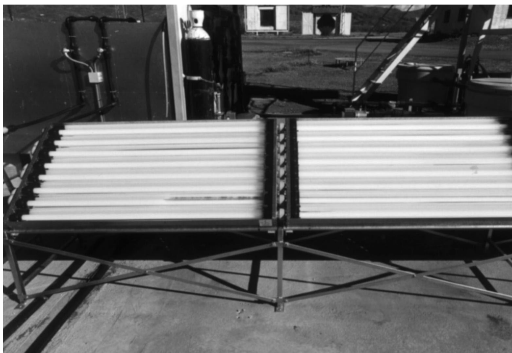
Fig. 9. Photograph of two CPCs of one prototype module (3 m 2 ) for photocatalytic experiments at PSA (Almería, Spain).
