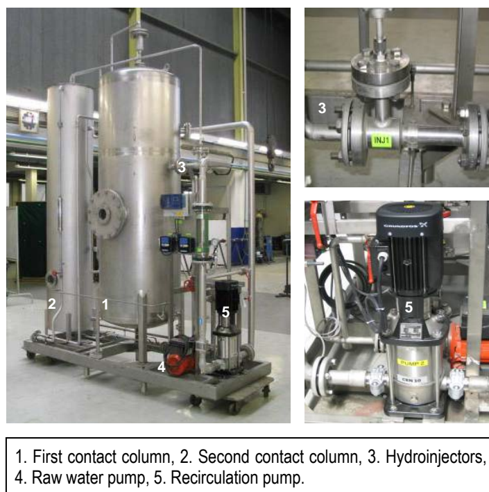
Figure 6.25. Images of the ozone unit designed by Trailigaz for the CADOX demonstration plant.
