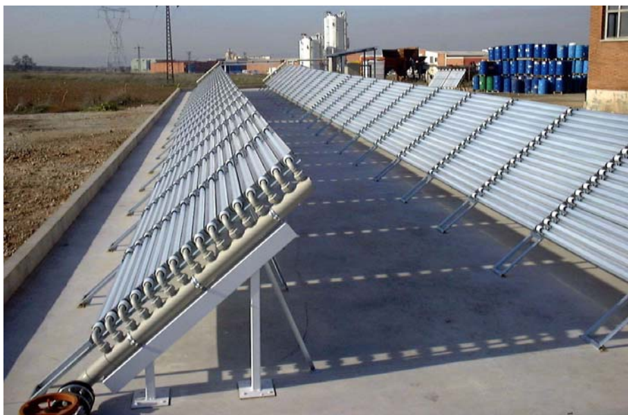
Figure 8 Partial view of the demonstration plant based on CPCs [Malato et al. , 2002 a]
