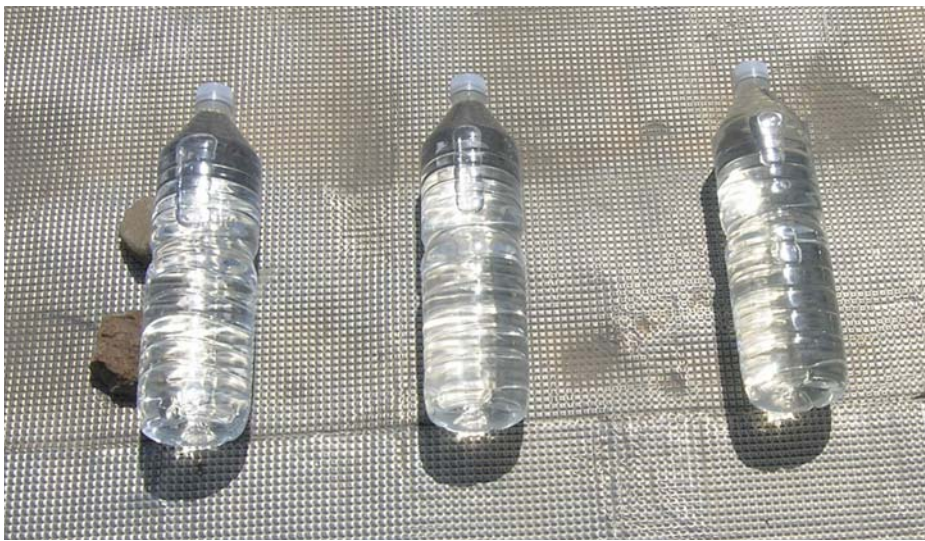
Figure 6 PET bottles filled with contaminated water and exposed to solar irradiation for water disinfection.
