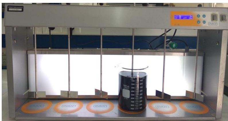
Figura III.23. Sistema “jar-test” JTS60E (OVAN).
