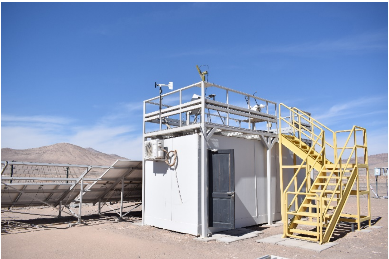
Figure 84. Weather station at the Plataforma Solar del Desierto de Atacama (PSDA) in Antofagasta (Chile). It is equipped with a large variety of instruments ranging from atmospheric parameter measurements to solar resource measurements.
