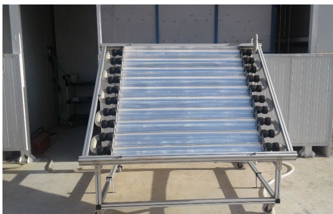
Figure 42. View of 2 m 2 -CPC coupled to Electro-Fenton pilot plant (ELECTROX).
