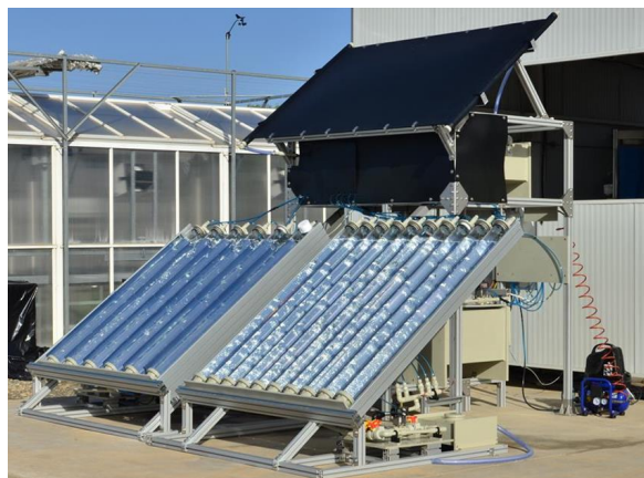
Figure 43. View of new CPC and U-type photoreactors (NOVA 75 V 1.0).
