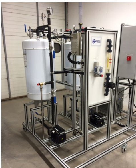
Figure 37. Bench-scale unit for testing membranes on isobaric MD.
