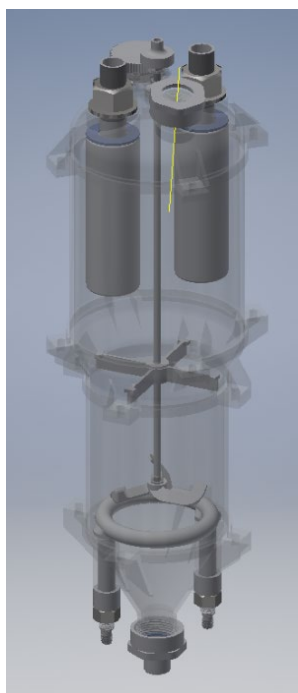
Figure 91. CAD model of the lunar test reactor.
