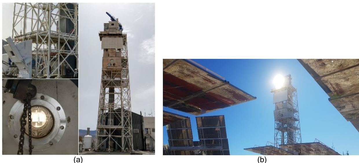
Figure 82. Erection of the testing equipment of the CAPTURE project in the CRS solar tower facility at PSA (left) and first commissioning tests (left).
