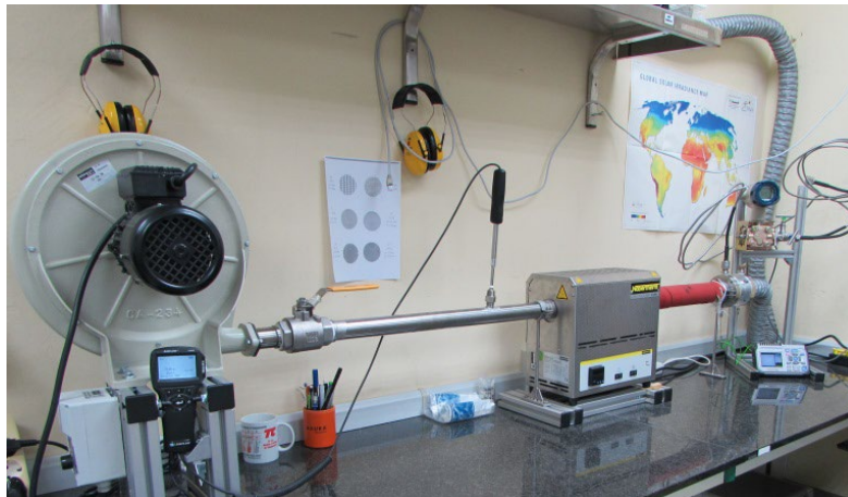
Figure 66. Test bench for pressure difference measurement with configuration up to 300°C.
