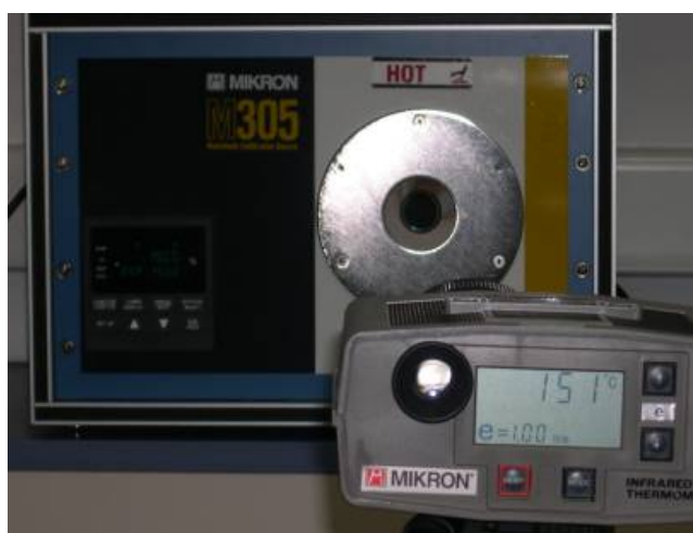
Figure 59. IR sensor calibration using a black body.
