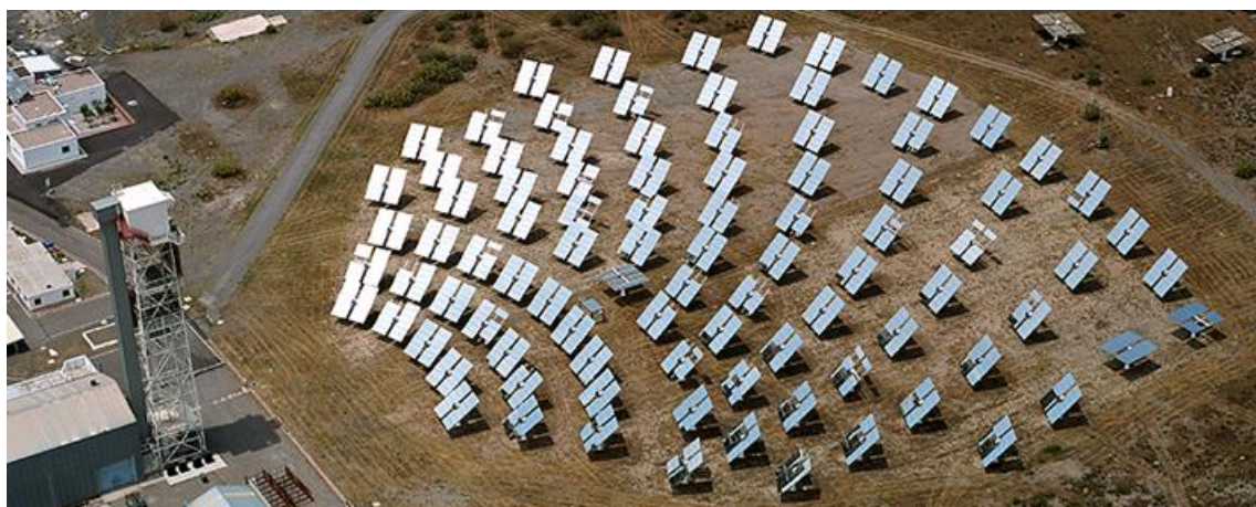
Figure 18. Aerial view of the experimental SSPS-CRS facility.
