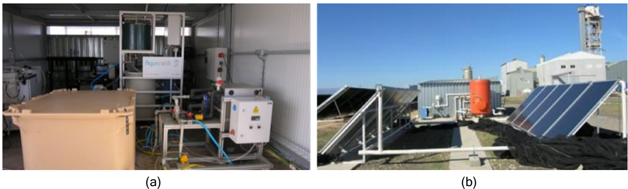
Figure 36. Internal (a) and external (b) views of the Membrane Distillation experimental test bed within the PSA low-temperature solar thermal desalination facility.
