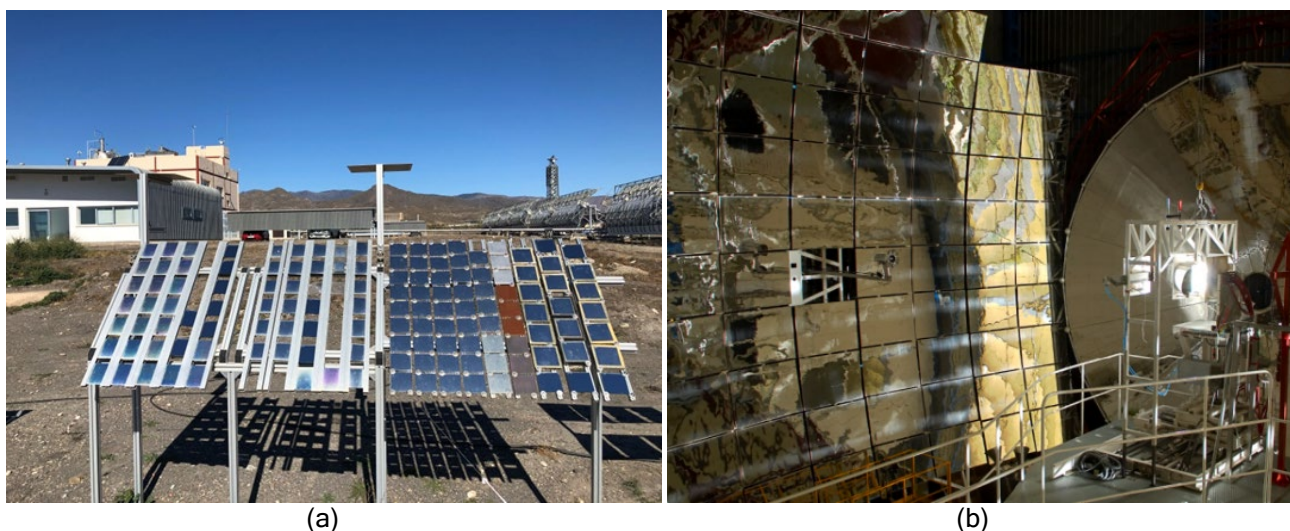
Figure 75. Test bench exposed outdoor at the PSA (a) and real operating test for secondary mirrors at the PSA solar furnace (b).
