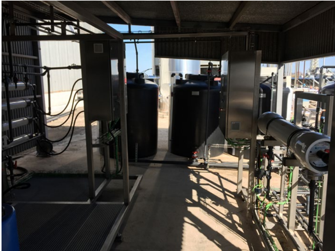
Figure 40. Test bed for FO-RO combination research.
