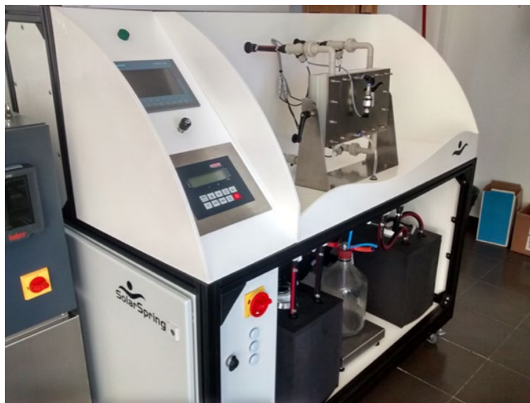
Figure 38. Bench-scale unit for testing MD with flat-sheet membranes.
