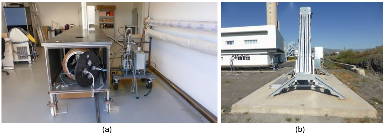
Figure 62. View of the HEATREC test chamber to measure heat losses in solar receiver tubes (a) and RESOL test bench to measure receiver's optical efficiency (b).
