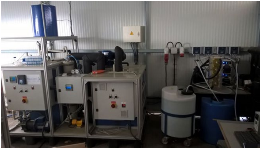
Figure 94. Pilot-plant for assessment of combined reverse electrodialysis and membrane distillation.
