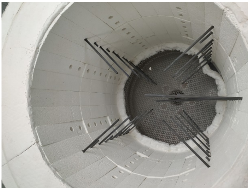
Figure 69. Picture taken from the upper part of the tank, showing its internal room and thermocouples at different lengths and radial positions.
