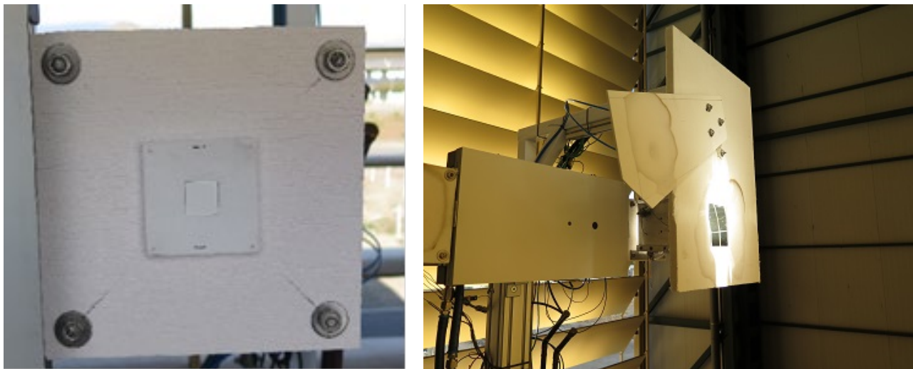
Figure 90. Sample under solar exposure at the SF40 facility.
