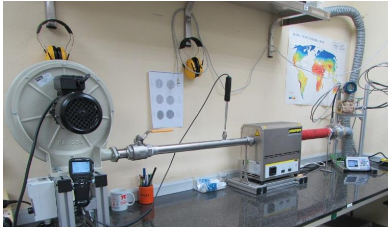
Figure 61. Test bench for pressure difference measurement with configuration up to 300°C.
