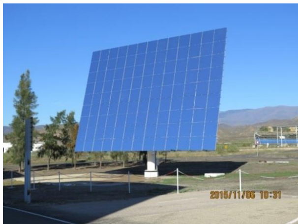
Figure 22. HT120 heliostat with new PSA facets.
