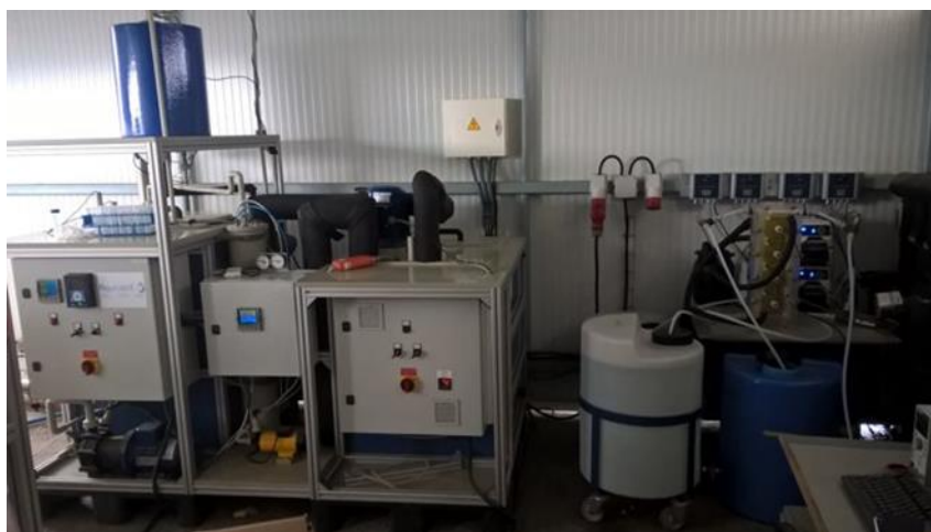
Figure 99. Pilot-plant for assessment of combined reverse electrodialysis and membrane distillation
