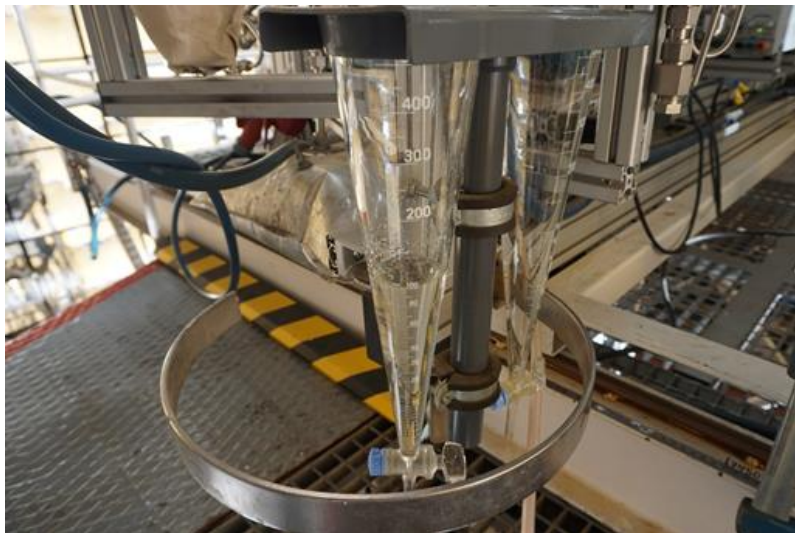
Figure 97. Production of 100g of water from hydrogen reduction of ilmenite demonstrated with the Oresol experiment in PSA's Solar Furnace SF60.
