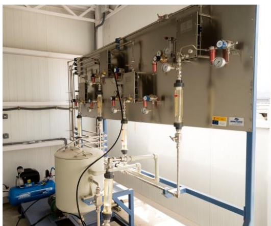
Figure 39. Electro-Fenton pilot plant coupled with a 2 m 2 CPC (ELECTROX).
