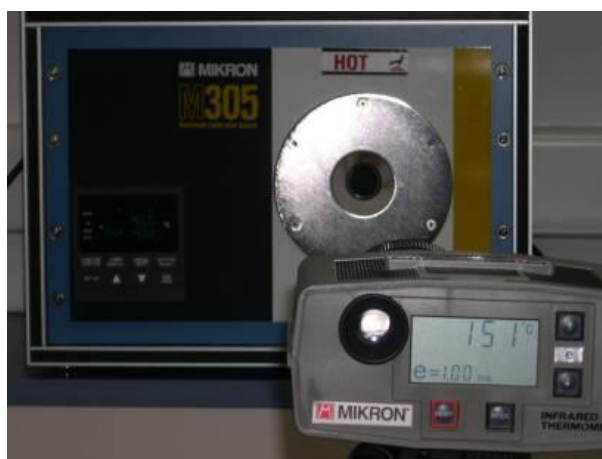
Figure 54. IR sensor calibration using a black body.
