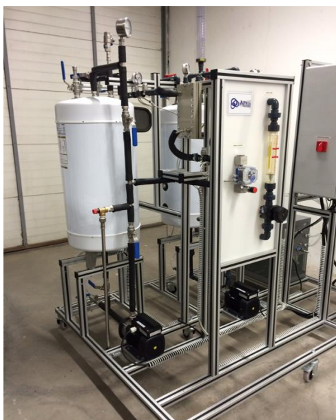
Figure 34. Bench-scale unit for testing membranes on isobaric MD.
