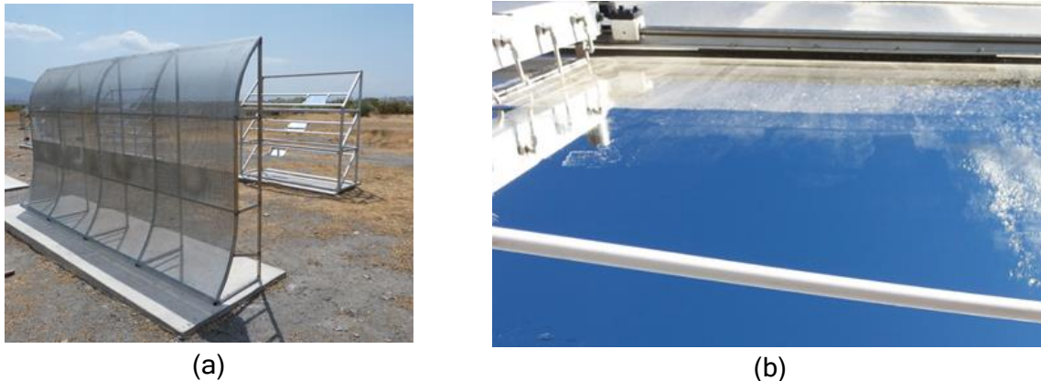
Figure 79. Dust barrier test bench (a) and ultrasonic cleaning system (b).
