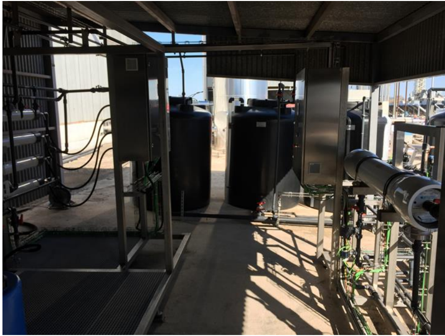
Figure 37. Test bed for FO-RO combination research.
