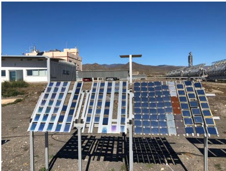
Figure 77. Test bench exposed outdoor for reflector samples at the PSA (RAISELIFE project).
