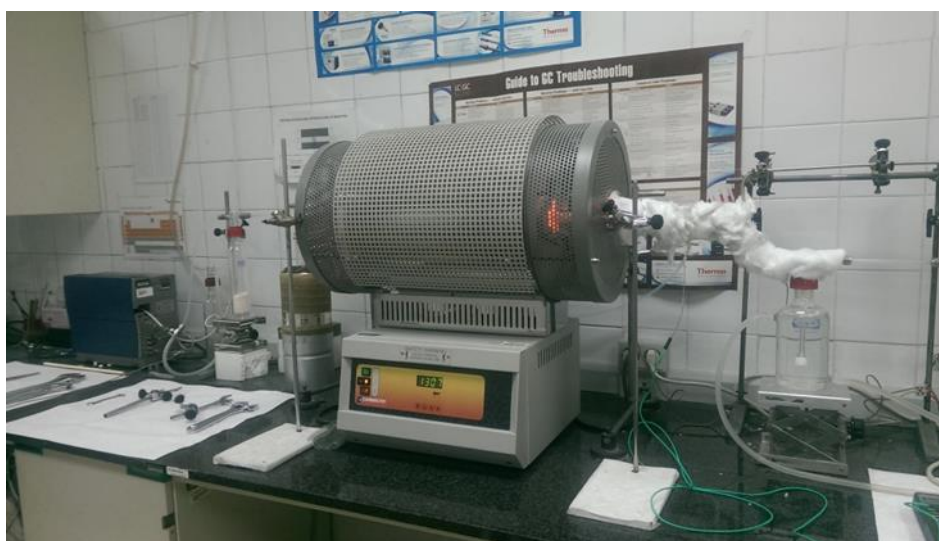
Figure 66. Indoor Solar Simulation Loop for evaluation of materials for thermochemical cycles.
