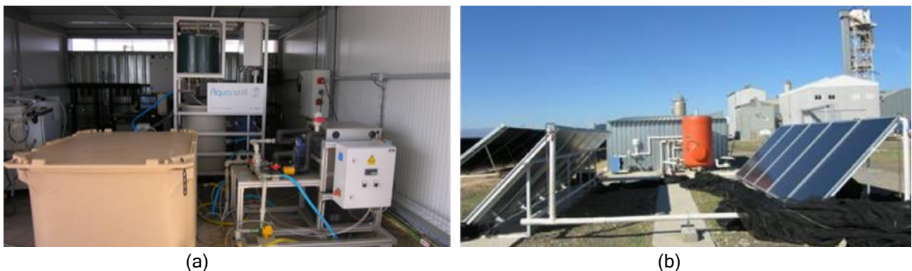
Figure 33. Internal (a) and external (b) views of the Membrane Distillation experimental test bed within the PSA low-temperature solar thermal desalination facility.
