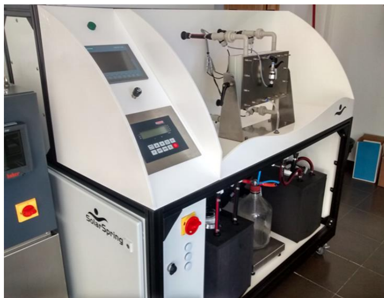
Figure 35. Bench-scale unit for testing MD with flat-sheet membranes.
