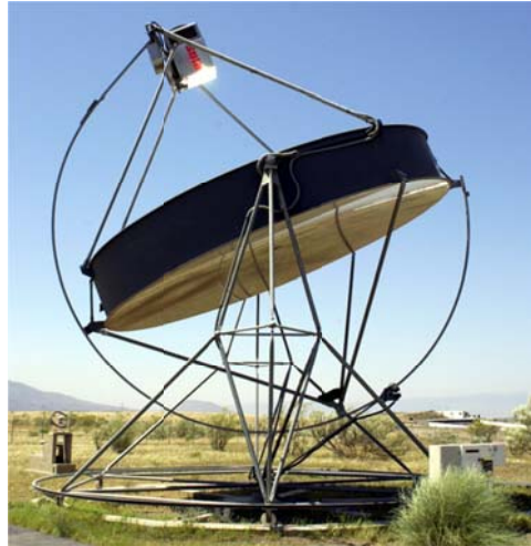
Figure 20. View of a parabolic-dish DISTAL- II.
