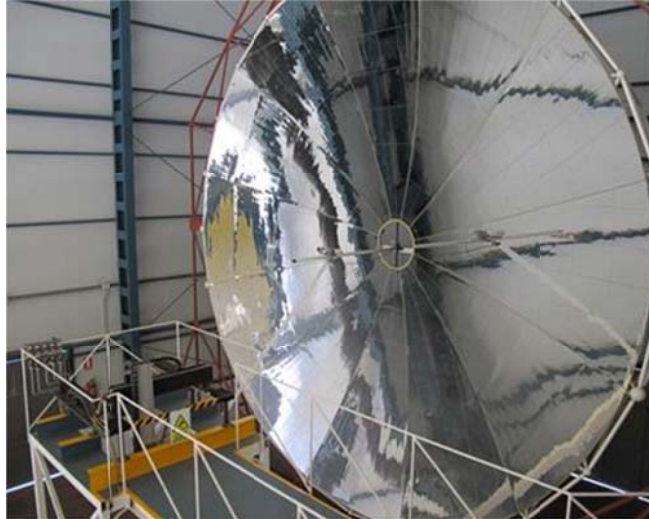
Figure 26. Interior of the SF-40 solar furnace, showing the parabolic concentrator.
