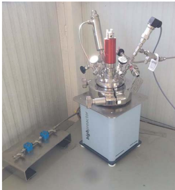
Figure 66. Wet Air Oxidation Pilot plant.
