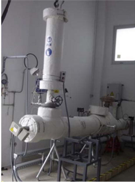
Figure 54. Test bench BES-I for evaluation of molten salt components.
