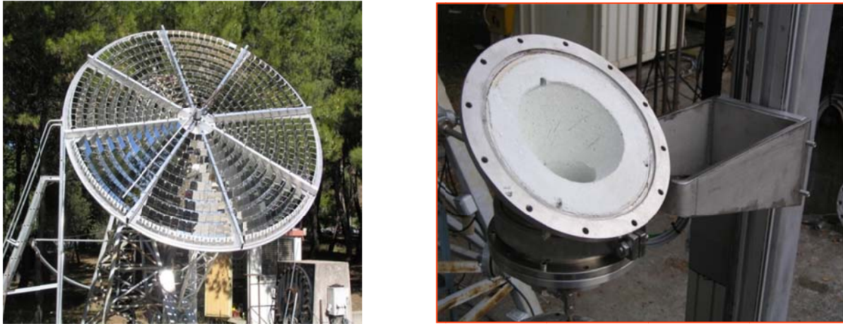
Figure 50. Outdoor Solar Double Reflection disc and a fluidised bed reactor on the focus
