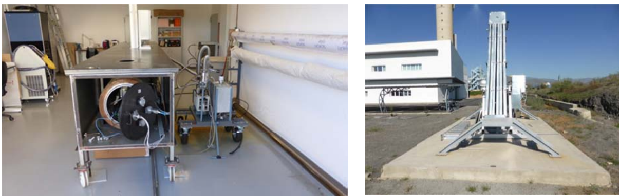
Figure 43. View of the HEATREC test chamber to measure heat losses in solar receiver tubes (left) and RESOL test bench to measure receiver's optical efficiency (right).
