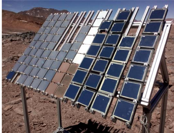
Figure 78. Test bench with mirror segments exposed outdoor in Chile.
