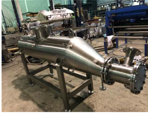
Figure 109. Steam generator already purchased at PSA facilities
