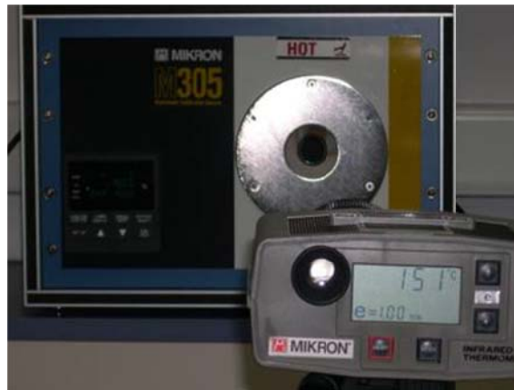
Figure 53. IR sensor calibration using a black body.
