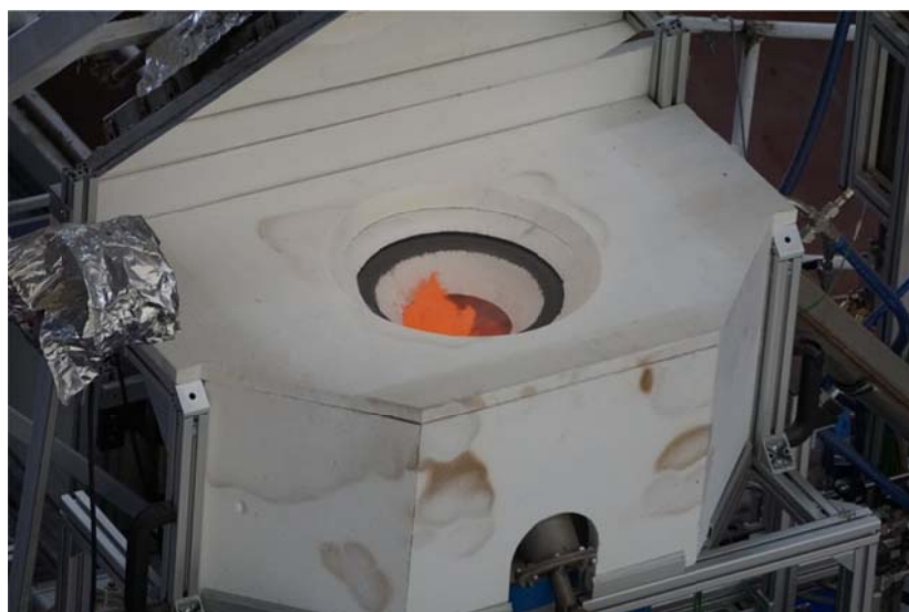
Fig. 91. Oresol experiment with hot particles on the test platform of the Solar Furnace SF60
