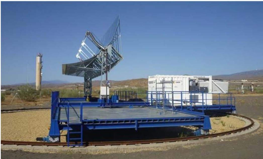
Figure 18. Side view of Kontas test bench and the heating cooling unit.
