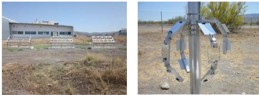
Figure 107. Picture of the test bench for the anti-soiling coating for reflectors (left) and absorber tubes (right)
