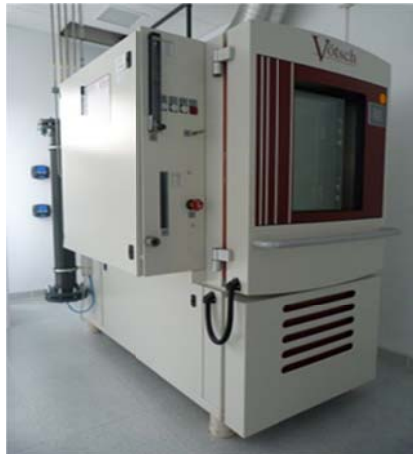
Figure 42. Climate chamber with corrosive gases.
