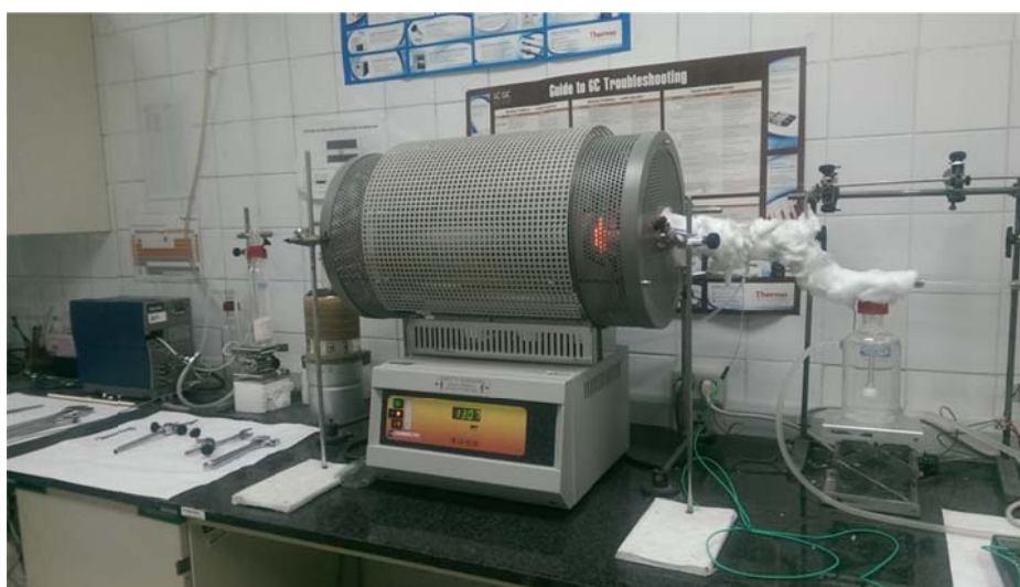
Figure 48. Indoor Solar Simulation Loop for evaluation of materials for thermochemical cycles
