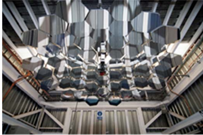
Figure 27. Concentrator of the SF-5 Furnace.
