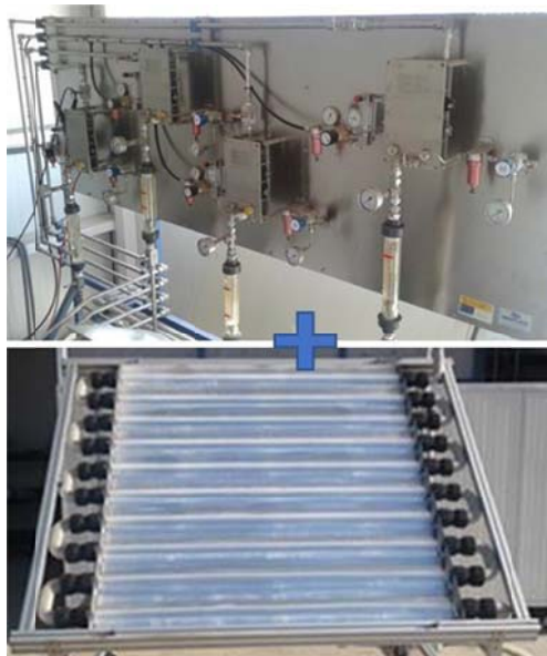
Figure 100. Photo-electro-Fenton pilot plant (4 electro cells combined with a solar CPC) for testing in TRICERATOPS project.
