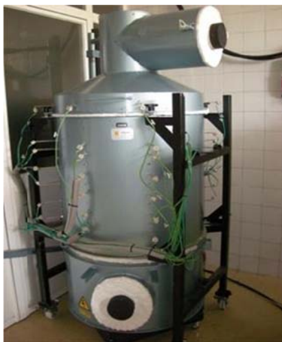
Figure 46. Front view of the lab-scale regenerative storage system in static arrangement.
