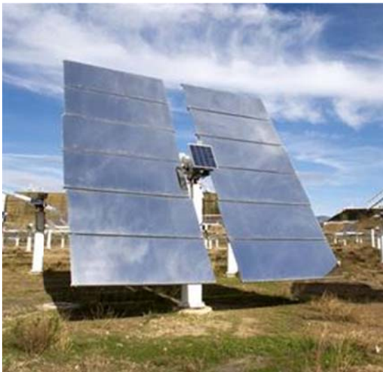
Figure 8. An autonomous heliostat in the CRS field.
