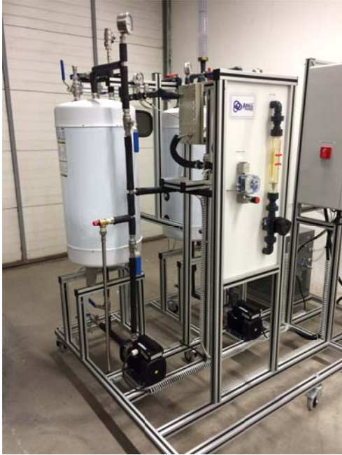
Figure 34. Bench-scale unit for testing membranes on isobaric MD
