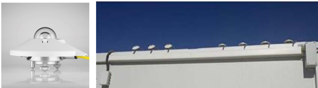
Figure 67. CUV-5 radiometer (left). View of all solar UV radiometers (inclined and horizontal setup) used in the Solar Water Treatment Unit (right).
