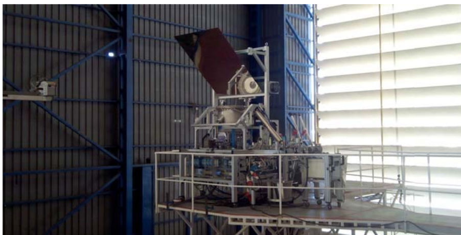
Figure 51. Testing of a ORESOL plant in a solar furnace to produce oxygen form regolite.
