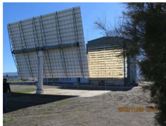
Figure 24. HT120 heliostat in tracking.
