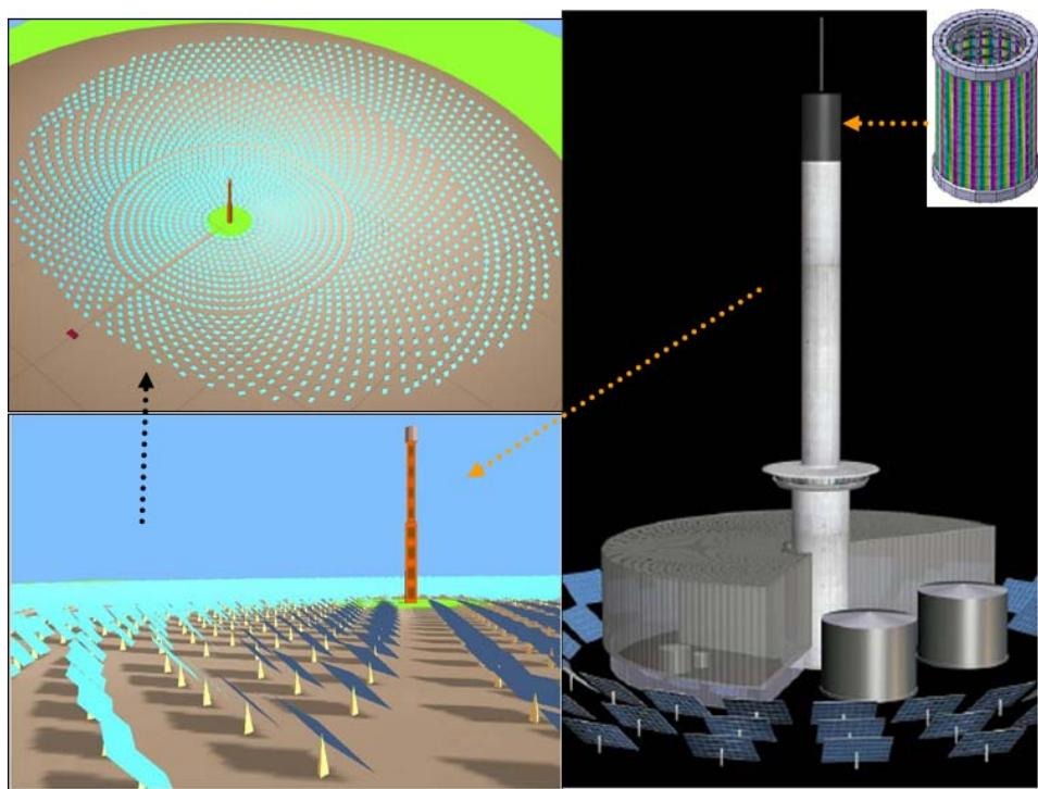
Figure 3.8 Predesign views of the Solar Tres plant
