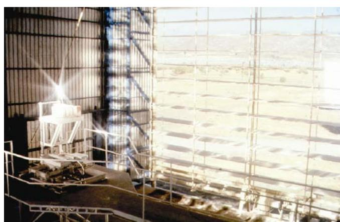
Figure 2.13 The focus and the test table on the left. On the right, the attenuator, completely open, allows the rays from the heliostats outside to enter.
