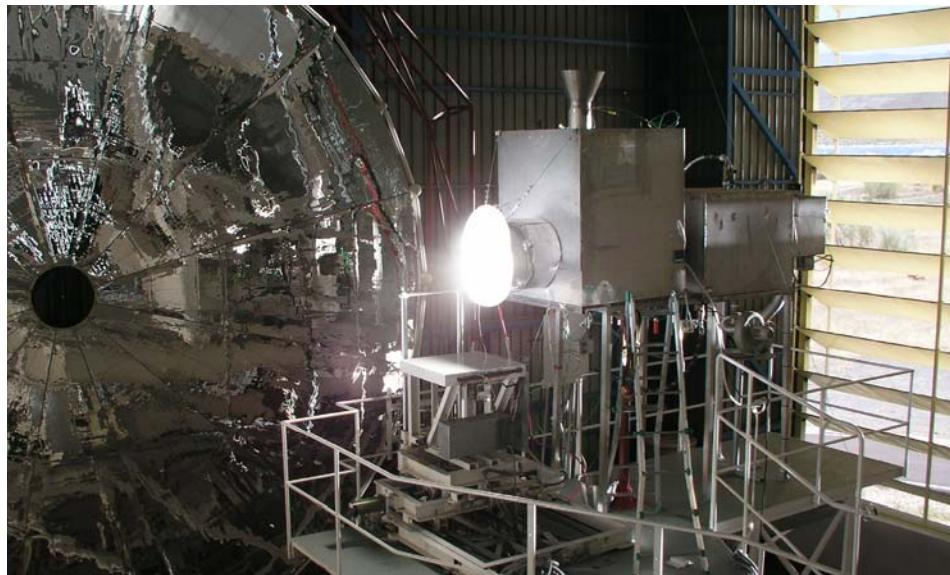
Figure 3.27 Fluidized bed reactor in operation in the PSA Solar Furnace
