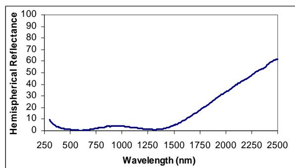
Figure 3.4 Hemispherical reflectance of the high-temperature absorbers
