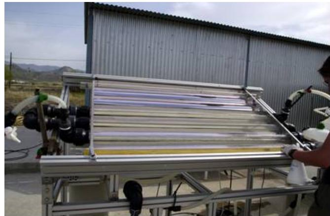
Figure 2.1 Partial view of the solar photochemical facilities. Front of solar CPC collector prototype used for water disinfection.
