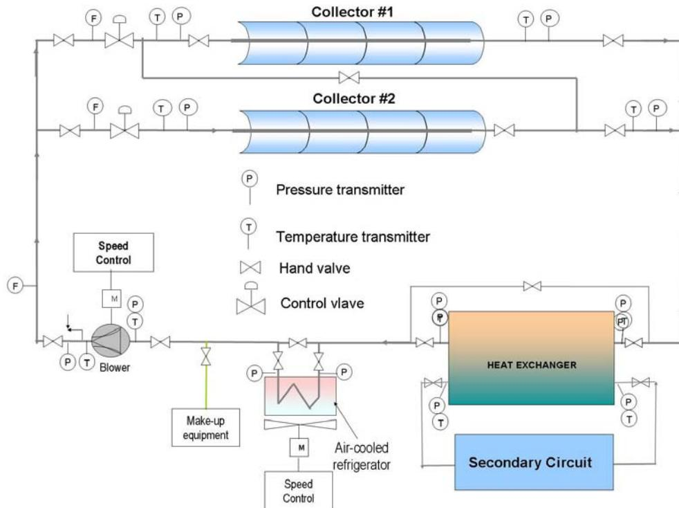
Figure 3.6 Diagram of the innovative fluid test loop
