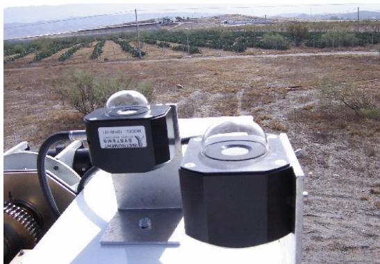
Figure 2.4 Spectroradiometer probes for measuring global and diffuse radiation installed in the solar tracker
