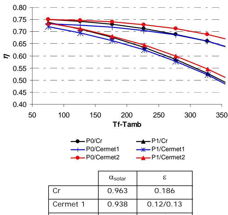
Figure 3.5 Simulation of the influence of absorber optical properties on overall performance of a parabolic-trough collector with a flat anti-reflective glass cover over the reflector and a vacuum ('P0') or atmospheric pressure ('P1') receiver
