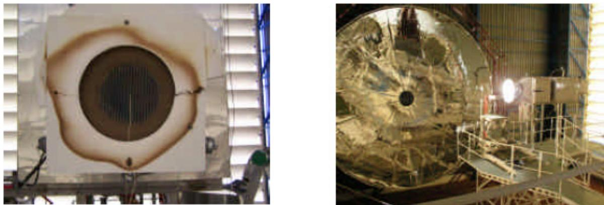
Figure 3.15 SiC volumetric absorber aging test. To analyze microstructural deterioration in this type of material, the concentration on the absorber was raised until small samples of the material started melting at surface temperatures of around 1500°C.
