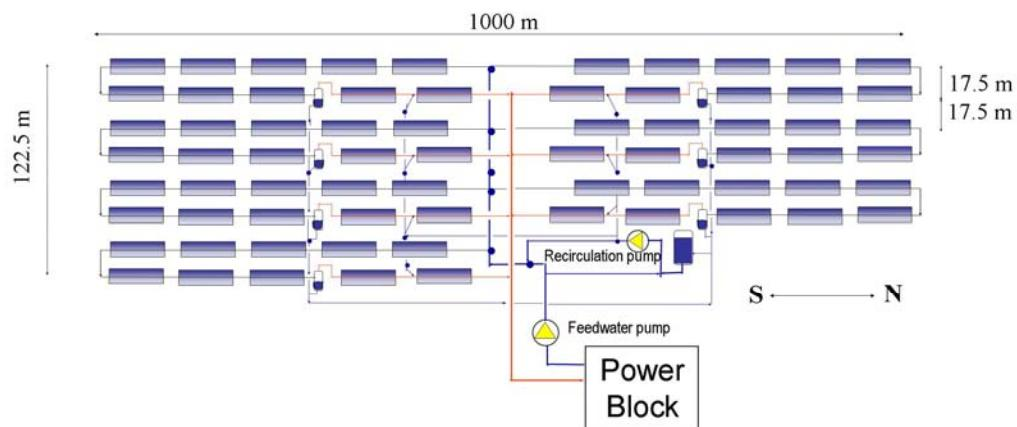
Figure 3.2 Schematic diagram of the 3 MW<sub>e</sub> Almería DSG plant.
