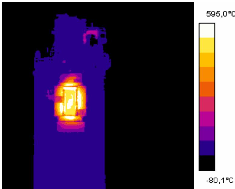
Figure 3.10 Infrared image of first salt receiver panel tests in the CESA-1 tower.
