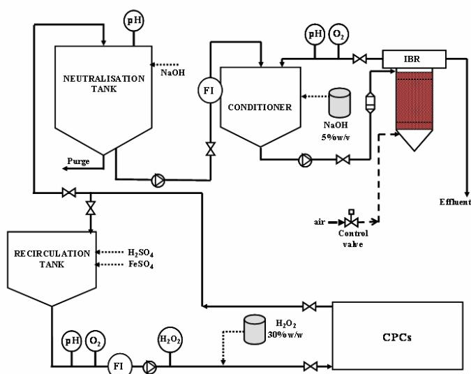
Figure 4.2 Conceptual design of photo-Fenton (solar radiation using CPC-type collectors) treatment of toxic and/or persistent waste water hooked up to biological treatment in a fixed-bed reactor
