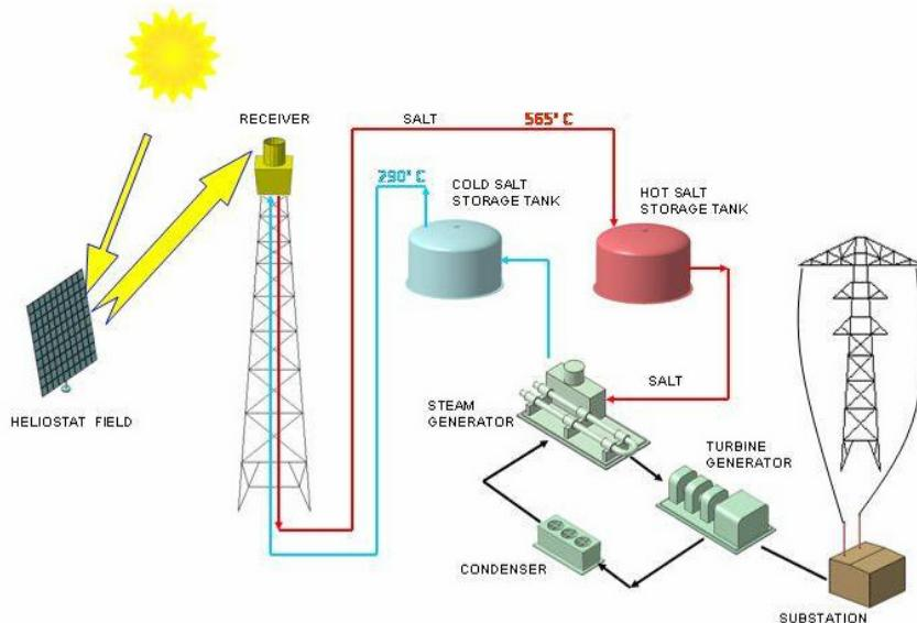
Figure 3.7 Flow diagram of the Solar Tres plant
