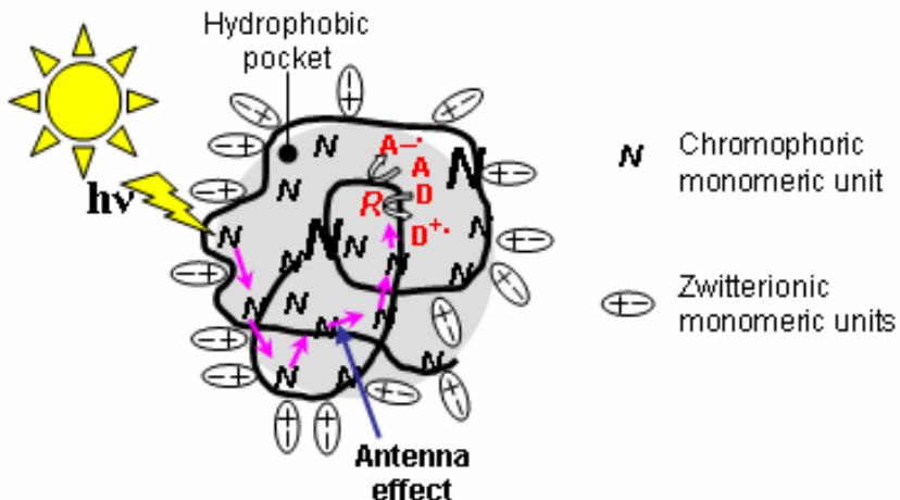
Figure 4.4 Conceptual illustration of light capture and formation of singlet oxygen in photozyme nanomicels (*R* is a unit of anthracene acting as a reactive center)
