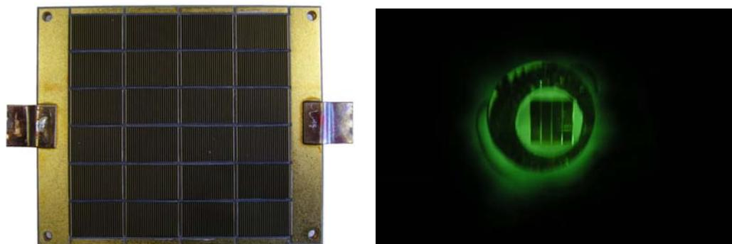
Figure 3.12 CCM Module: 120VDC and 21A and photo during testing at 1 MW/m<sup>2</sup>.
