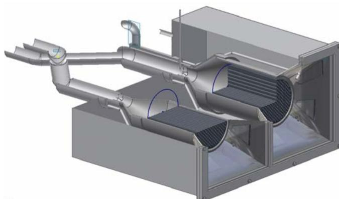
Figure 3.26 Detail of the housing device for the activation and hydrolysis reactors used in Hydrosol-II
