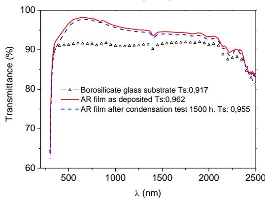
Figure 3.3 Glass transmittance with and without the AR film, before and after 1500 h in weathering chamber
