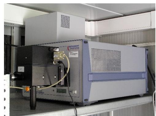
Figure 2.5 Spectroradiometer detector with three-probe connector switch
