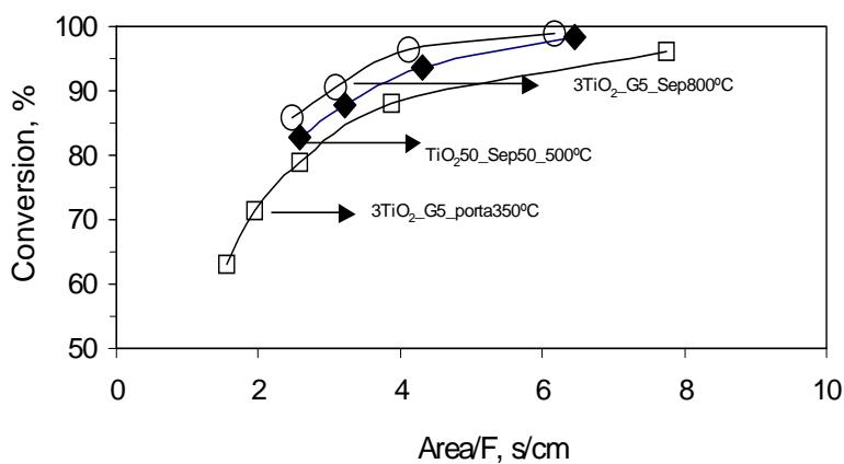
Figure 4.12 Trichloroethylene conversion as a function of the illuminated area to flow ratio (Area/F) for three different photocatalysts:  $\text{TiO}_2$  coating on the silicate, a 50:50 W/w  $\text{TiO}_2$ /silicate mixture and a  $\text{TiO}_2$  layer on a glass plate. Initial pollutant concentration 10 ppmv
