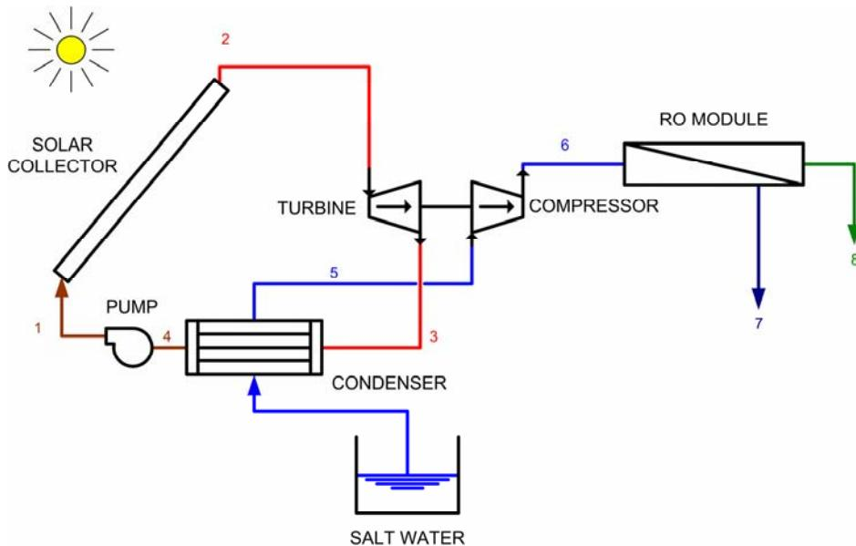
Figure 4.16 Generic reverse osmosis system hooked up to a solar driver
