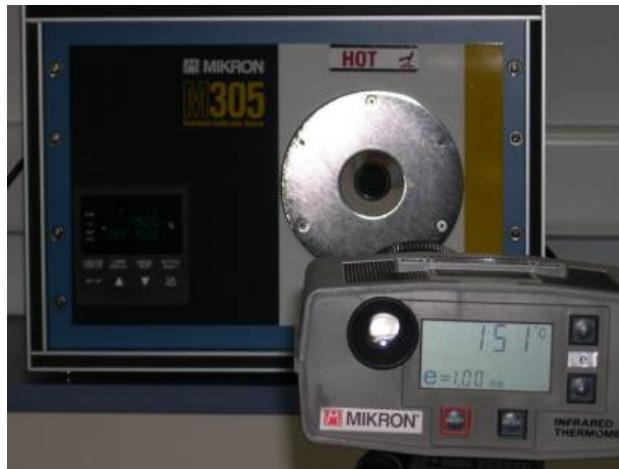
Figure 3.20 Calibration of an IR detector in the laboratory.
