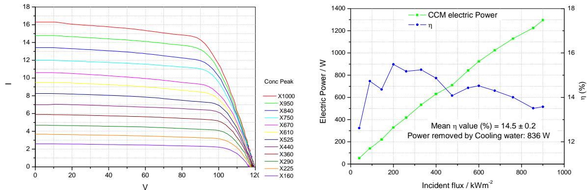
Figure 3.13 IV curves for the CCM tested at different concentrations in the solar furnace; delivered electric potential and efficiency curves.
