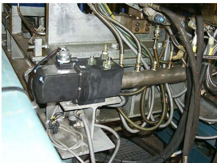
Figure 3.18 The Metering Valve (fuel lines disconnected)
