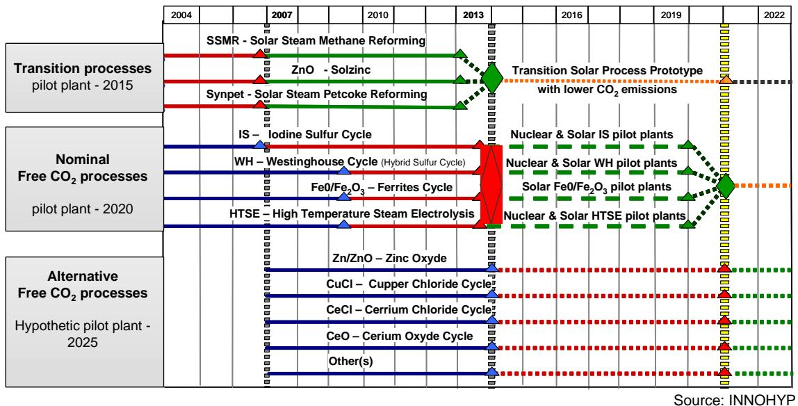
Figure 3.22 Main high-temperature thermal hydrogen production processes retained for development for a future hydrogen economy .
