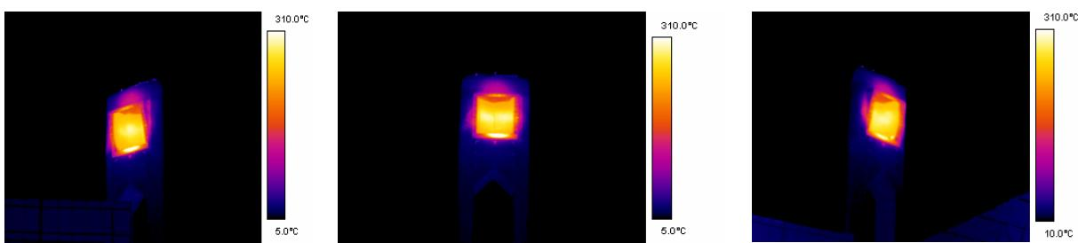
Figure 3.11 Infrared measurement of the PS10 receiver during commissioning (14/12/06) from three field observation points
