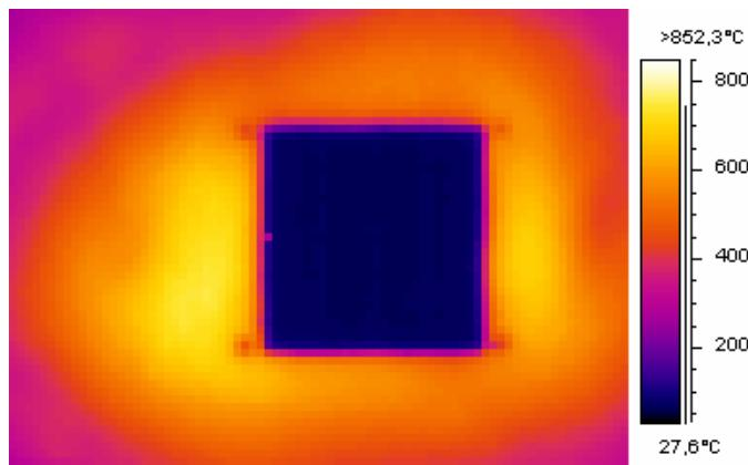
Figure 3.14 Thermogram of CCM surface temperature at 1 MW/m<sup>2</sup> concentration
