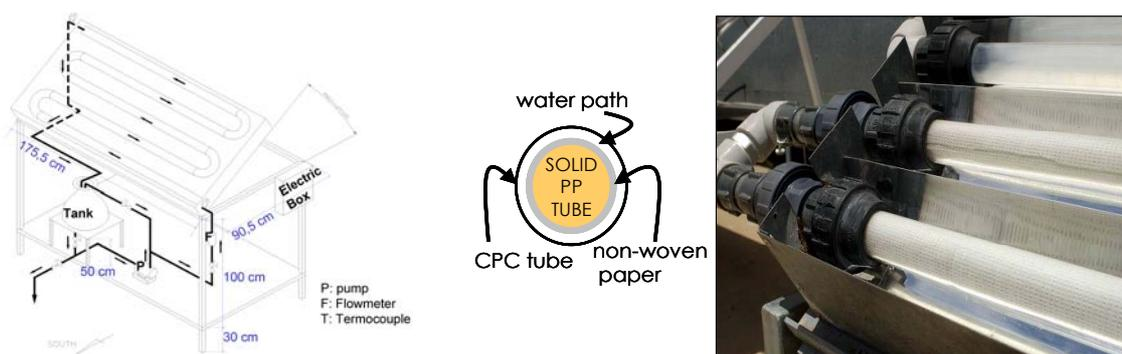
**Figure 67.** Photoreactor for disinfection by photocatalysis (left) and solar concentric arrangement of Ahlstrom paper with TiO<sub>2</sub> (right).
