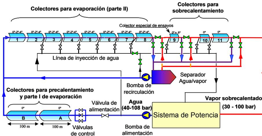
Figure 11. Simplified diagram of the PSA DISS plant
