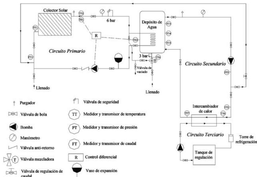
Figure 28. General schematic diagram of the stationary solar collector test bed.
