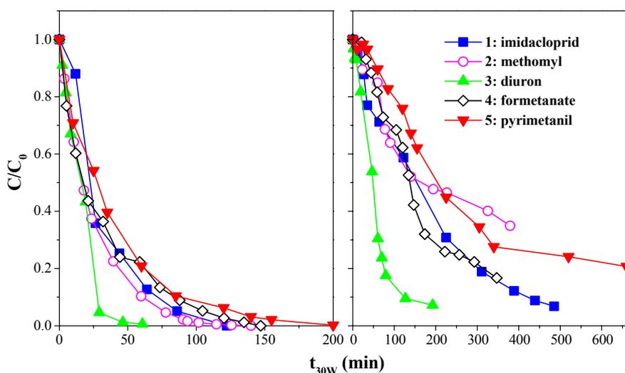
Figure 56. Degradation (left) and mineralization (right) of several pesticides at  $C_0 = 50$  mg/L using TiO<sub>2</sub> (200 mg/L).
