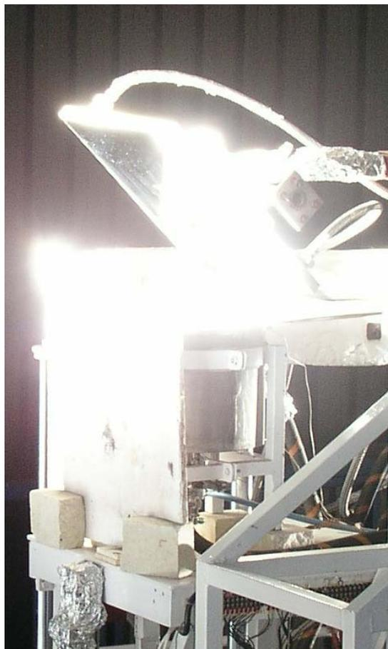
Figure 81. Tilted mirror and MiniVac during testing
