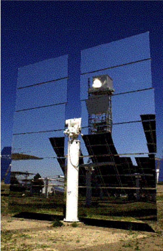
**Figure 8. A CRS field heliostat reflecting the tower**
