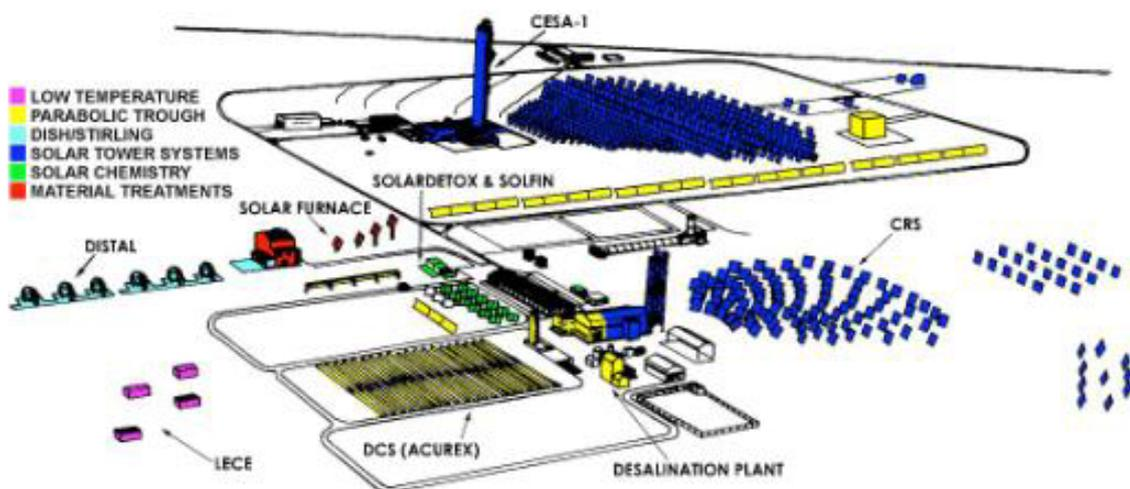
Figure 6. Location of the main PSA test facilities
