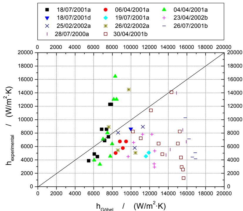
**Figure 55. Comparison of the Goebel (1998) correlation and the surface convective heat transfer coefficient values obtained from the DISS experimental data.**
