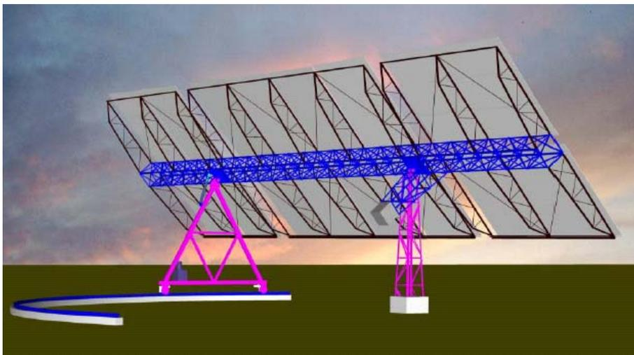
**Figure 36. Artist's view of the 200-m<sup>2</sup> Megahelio heliostat (Design by SOLUCAR)**
