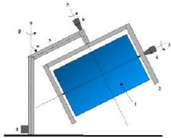
**Figure 37. Confined line-focusing cylindrical heliostat**
