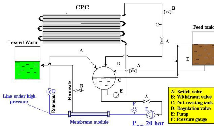
Figure 70. Conceptual diagram of the membrane system coupled to a CPC photoreactor
