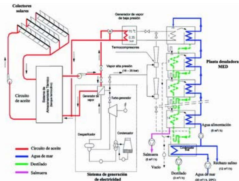
Figure 13. General diagram of the SSPS-DCS plant
