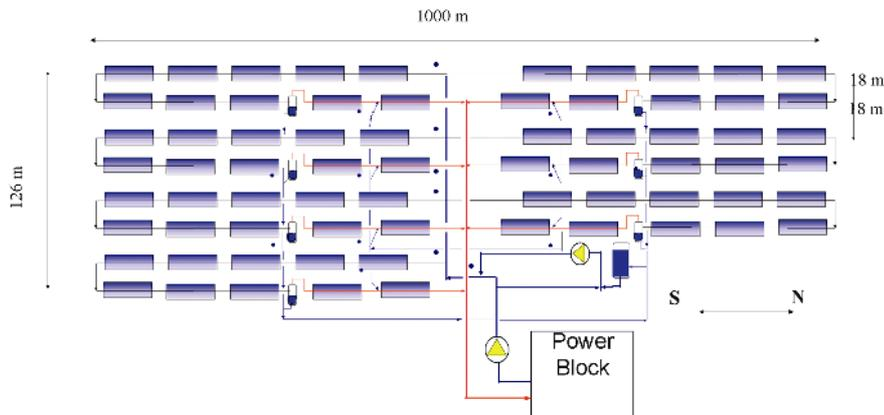
**Figure 47. Simplified diagram of the INDITEP plant solar field designed by CIEMAT.**
