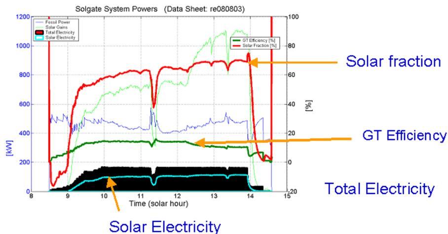
**Figure 42. Results of operating the SOLGATE system on August 8, 2003 (Maximum temperature 960°C)**
