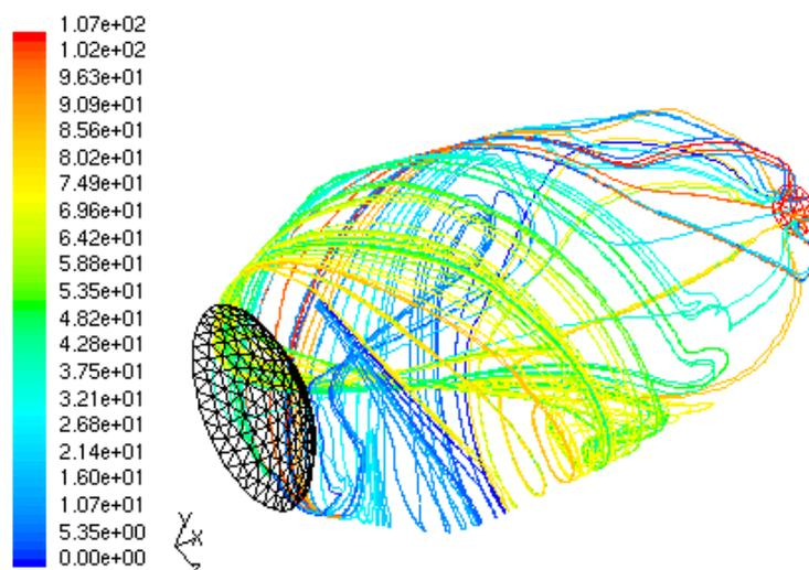
Figure 77. "FLUENT" code modeling of particle flux inside the reactor. Analysis conditions: Flux by injector = 2 Ln/min =  $4.0833 \times 10^{-5}$  kg/s Total flux = 12 Ln/min; Theoretical mean residence time = 4.72 s. Injectors = 1A, 2A,3A,4A,5A,6A; Tangential injection ( $\alpha=0, \beta=90$ )
