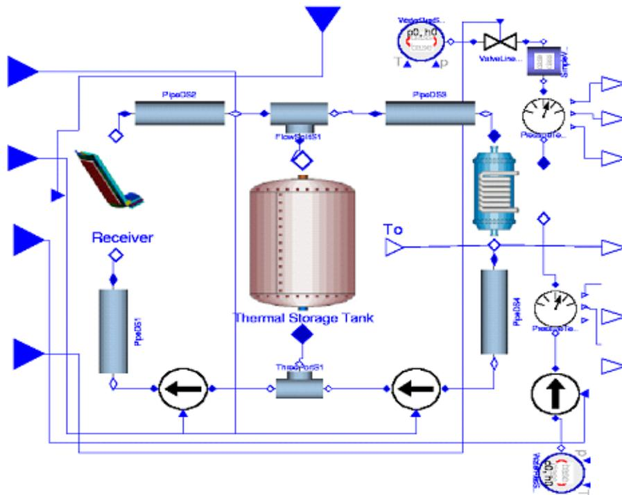
Figure 43. Graphic environment developed in Labview® for the new SOLAIR facility control system (arriba) y Dynamic model of the new SOLAIR facility control system using Dymola/Modelica® (abajo)
