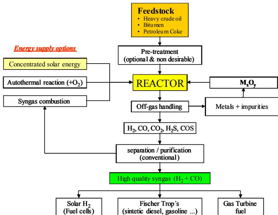
Figure 75. Flow diagram of the process to be technologically developed
