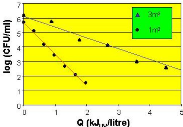
Figure 71. Inactivation of *E.coli* (log(CFU/ml)) as a function of solar UV solar collected in CPCs with 1 and 3 m<sup>2</sup> collector surfaces
