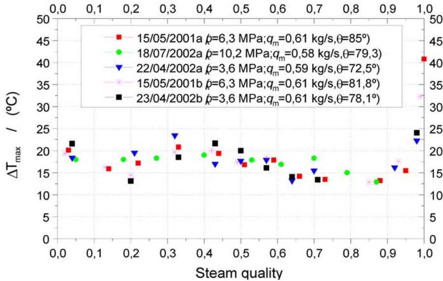
**Figure 53. Measured values of the maximum circumferential temperatures in the absorber tube evaporating zone, depending on the steam quality.**
