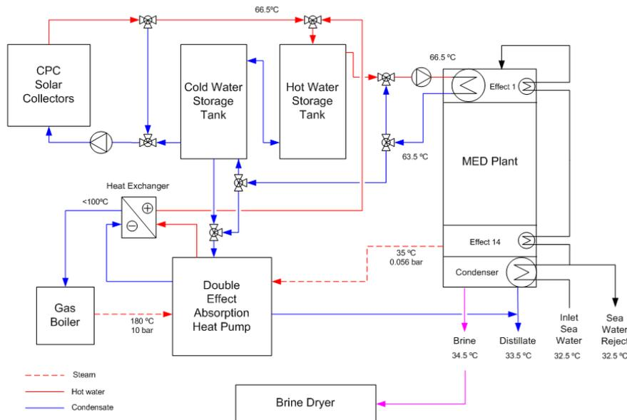
**Figure 68. Final configuration of the desalination system to be erected in the AQUASOL Project.**
