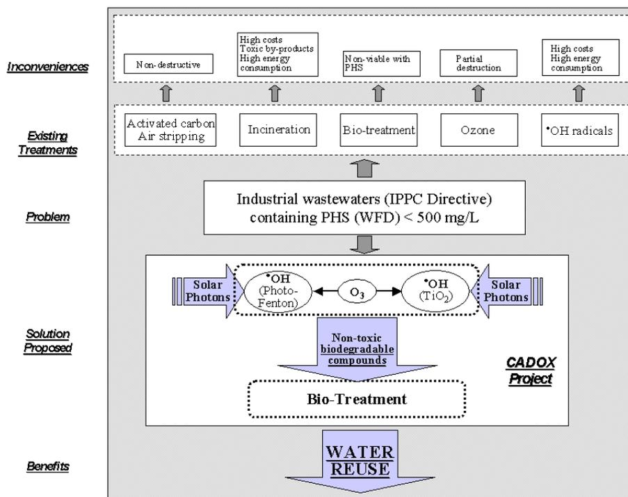
Figure 61. Innovative aspects of the CADOX project and schematic summary of alternative technologies
