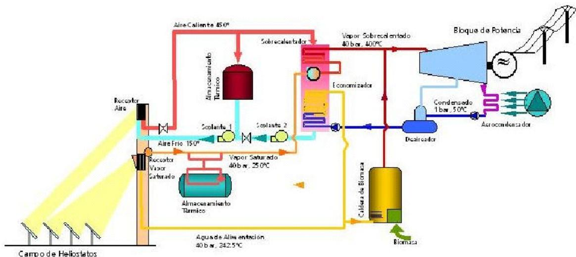
**Figure 45. Schematic diagram of the 1.5-MW SOLPRO plant proposed for the PSA.**
