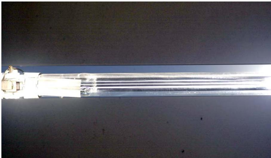
**Figure 54. High flux lines on DISS absorber tubes**
