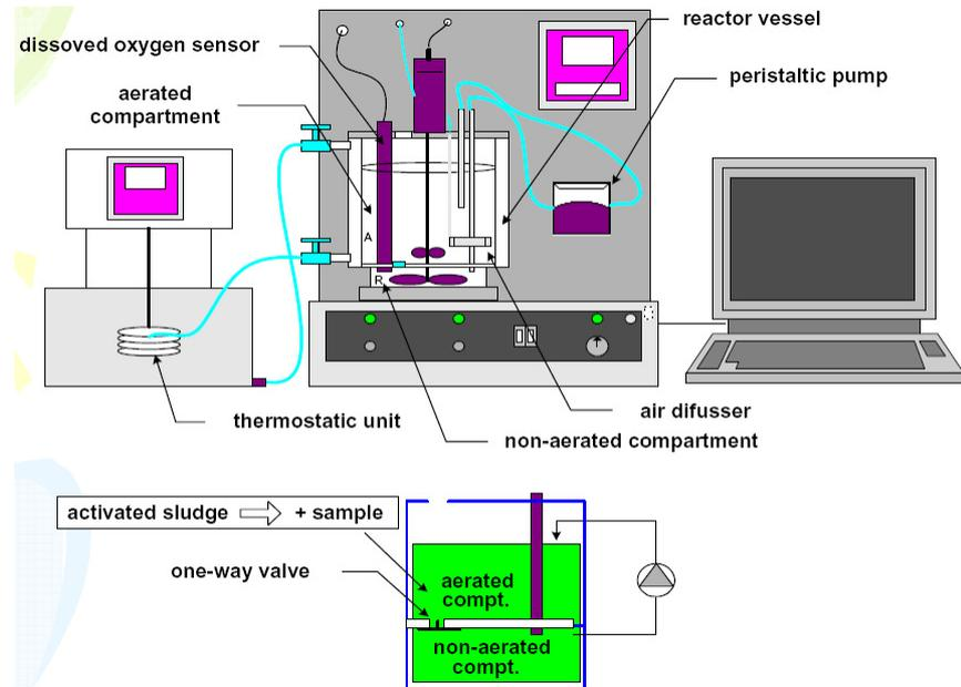
Figure 5 Experimental set-up of the Respirometer
