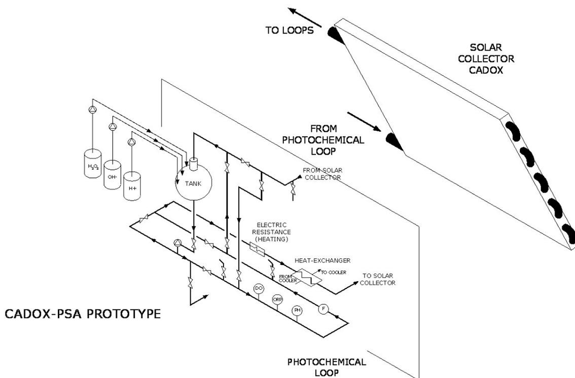
Figure 7 isometric drawing of the CADOX plant at PSA
