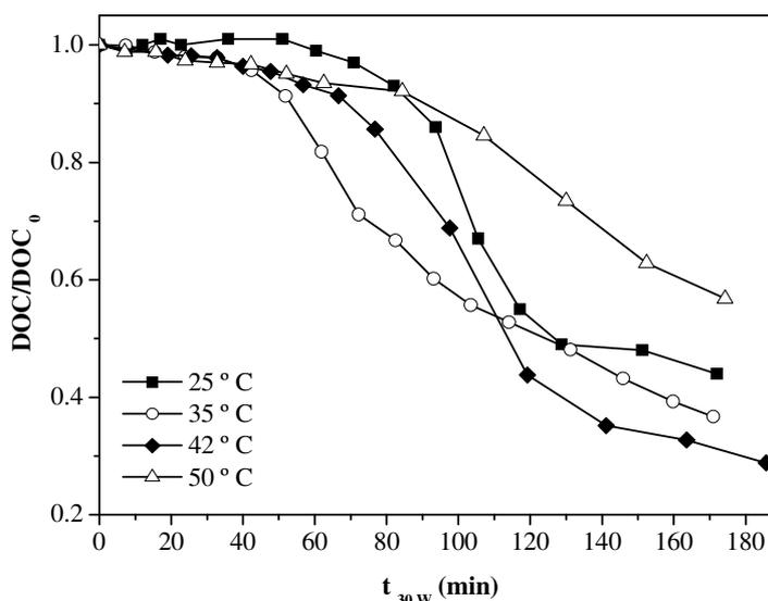
Figure 10 Mineralization depicted on illumination time for all temperatures, DOC 200mg L<sup>-1</sup>
