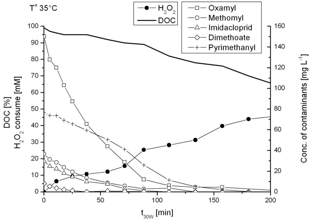
Figure 13 Mineralization,  $\text{H}_2\text{O}_2$  consumption and decomposition of the initial compounds at  $35^\circ\text{C}$ , initial DOC  $500\text{ mg L}^{-1}$  pesticide compounds had been entirely degraded.
