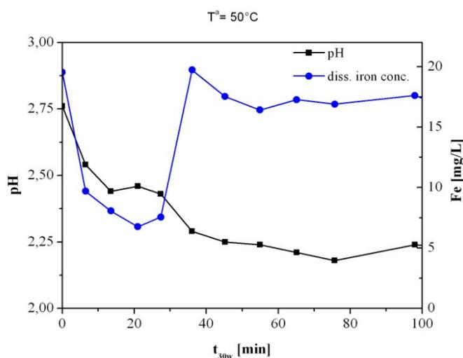
Figure 11 Behavior of the pH and total diss. Iron at 50°C and 200 mg L<sup>-1</sup> DOC
