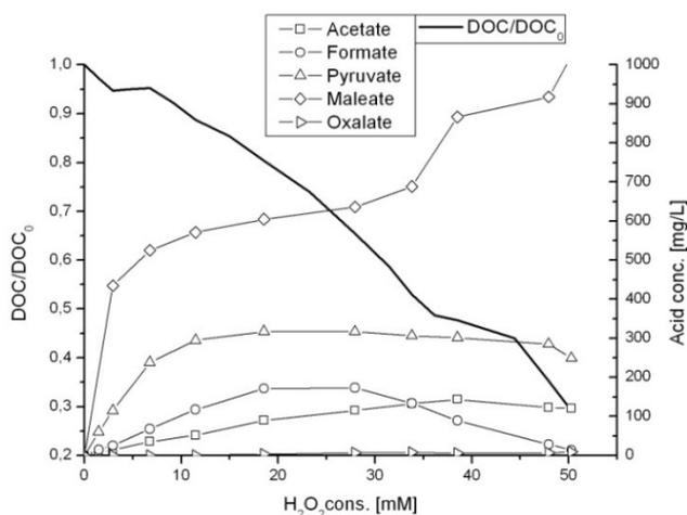
Figure 15 Results of the IC analysis, formation of organic acids and mineralization at 35°C (500 mg L<sup>-1</sup> initial DOC)
