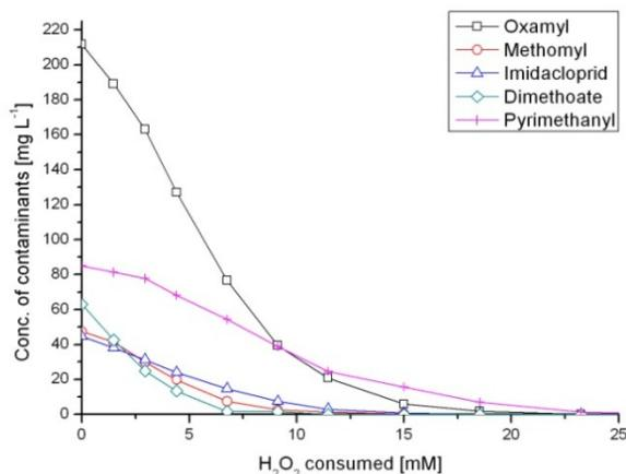
Figure 14 Decomposition of the five pesticides with controlled doses, initial DOC 500 mg L<sup>-1</sup>
