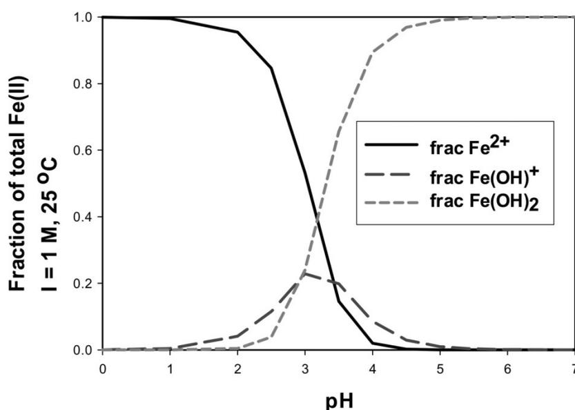
Figure 2 Speciation of Fe (II) in water as a function of pH at 1 M ionic strength [Pignatello J., Oliveros E. et al., 2006]
