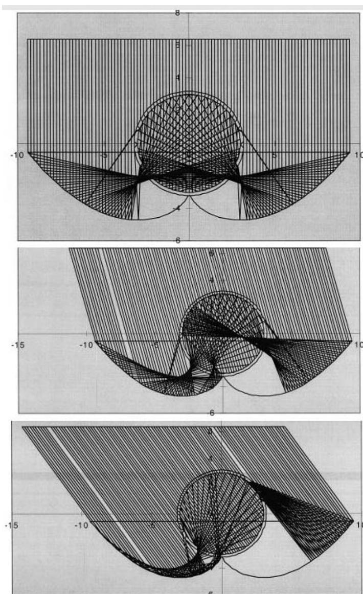
Figure 1 CPC reflector with tube [Malato S., 2004]
