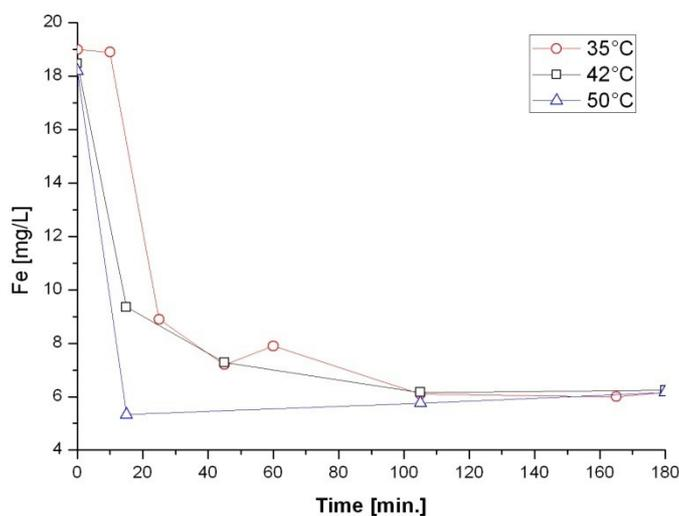
Figure 12 Behavior of dissolved iron in absence of pesticides (blank) at three different temperatures
