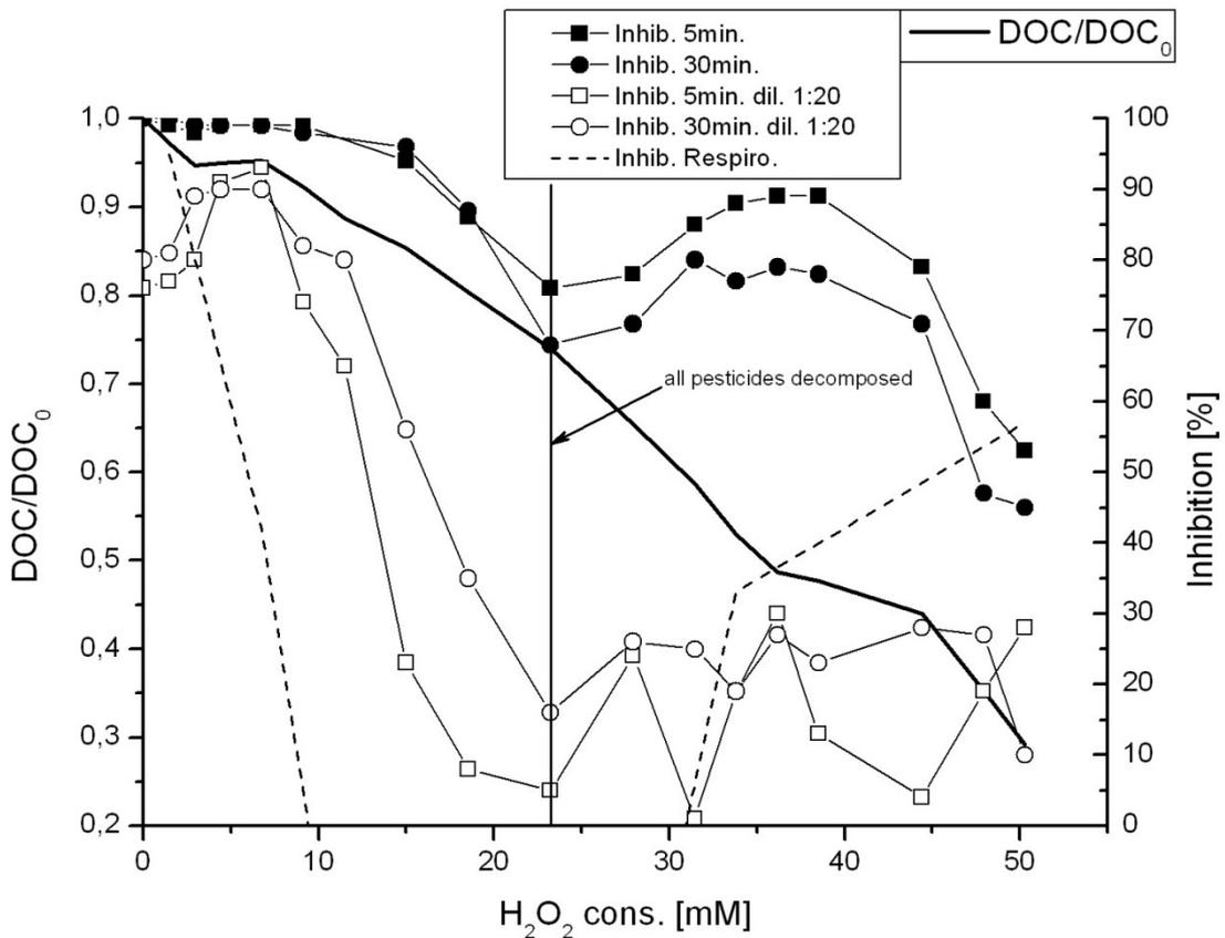
Figure 16 Results for toxicity assays with *Vibrio fischeri* (Inhibition after 5 + 30min., non diluted and with a dilution factor of 1:20) and Respirometry; mineralization depicted on  $H_2O_2$  consumption
