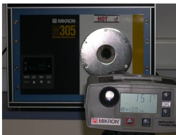
Figure 63. IR sensor calibration using a black body.
