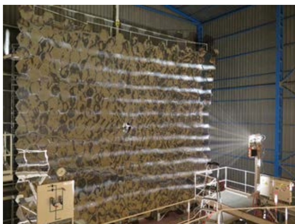
Figure 27. Interior view of the PSA SF-60 Solar Furnace in operation.
