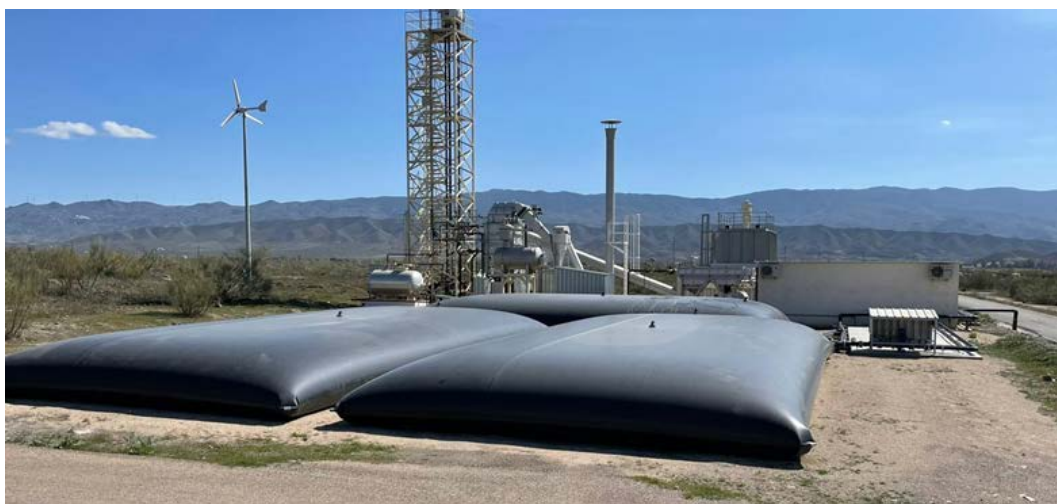
Figure 41. Containers filled with real seawater for desalination tests in closed loop.
