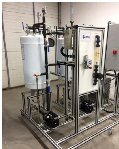
Figure 71. Bench-scale unit for testing membranes on isobaric MD.
