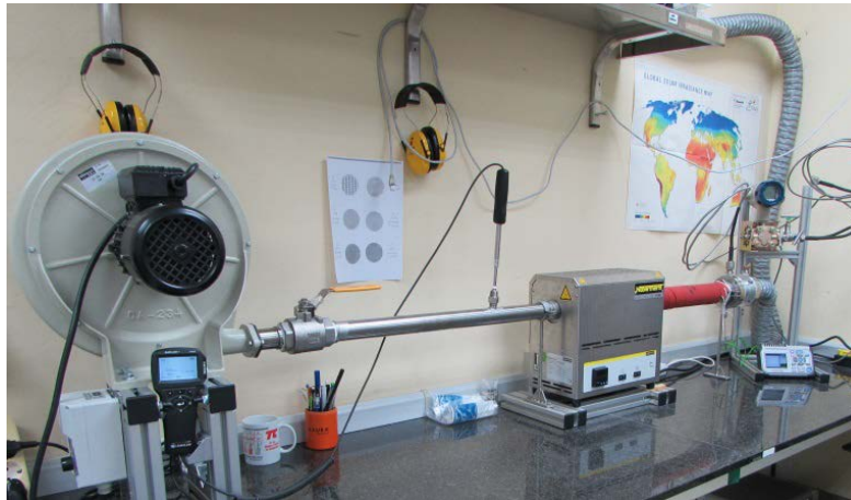
Figure 69. Test bench for pressure difference measurement with configuration up to 300°C.
