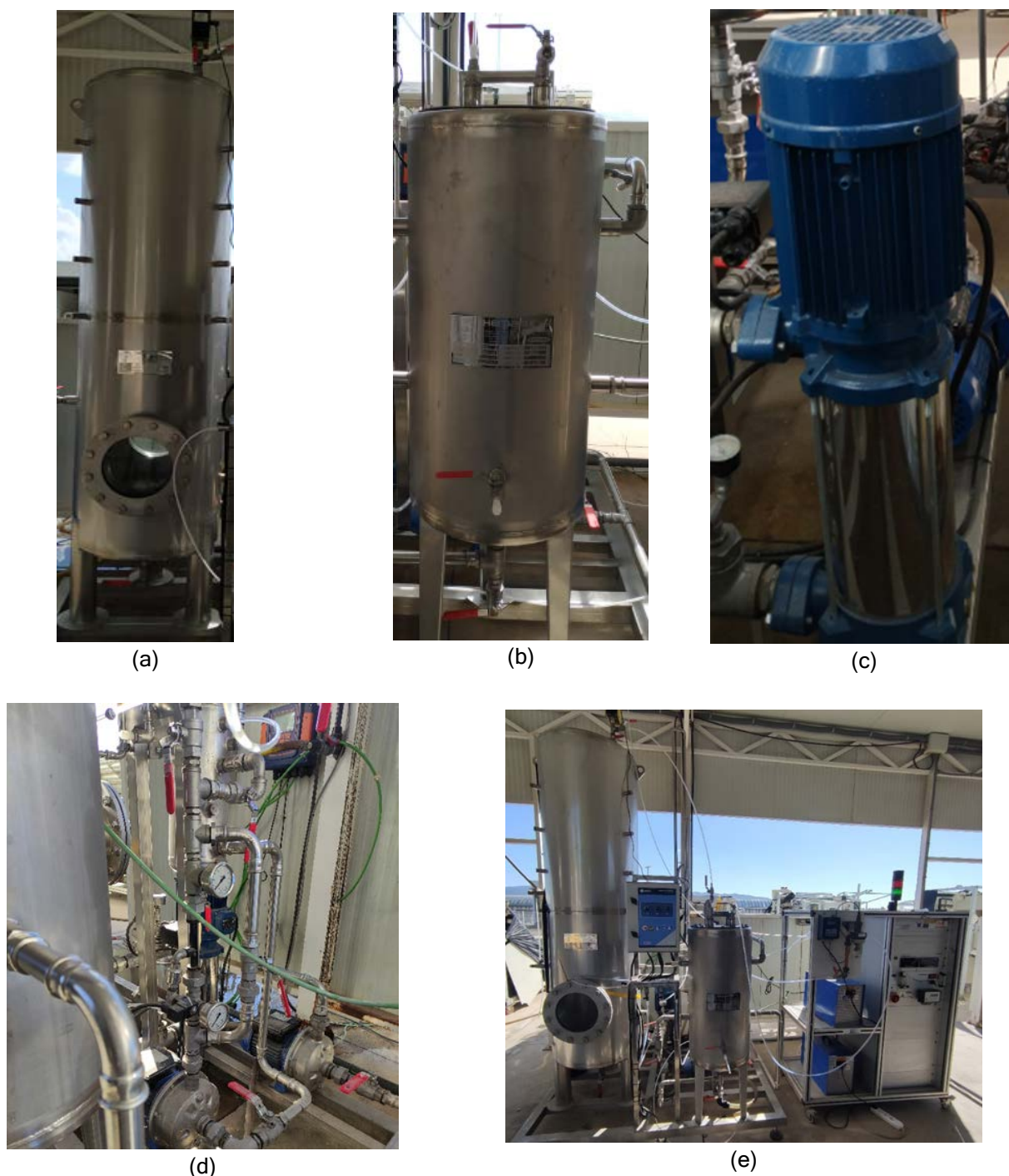
Figure 48. Pictures of the improved parts of the ozonation pilot plant: a) New 580L contact column reactor; b) Pressurized tank; c) HP pump for nano-bubbles generation; d) Venturi for micro-bubbles injection and e) complete view of the new ozonation pilot plant.
