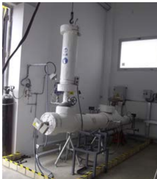
Figure 32. MOSA indoor test bench (BES-II).
