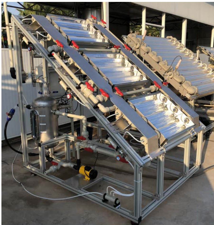
Figure 49. Solar CPC with direct injection of ozone available at PSA facilities.
