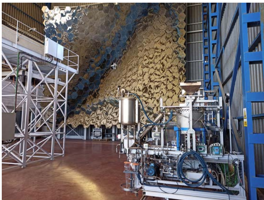
Figure 103. Oresol system in summer 2021 awaiting future testing. In the background the recently replaced, brand-new concentrator of the PSA Solar Furnace.
