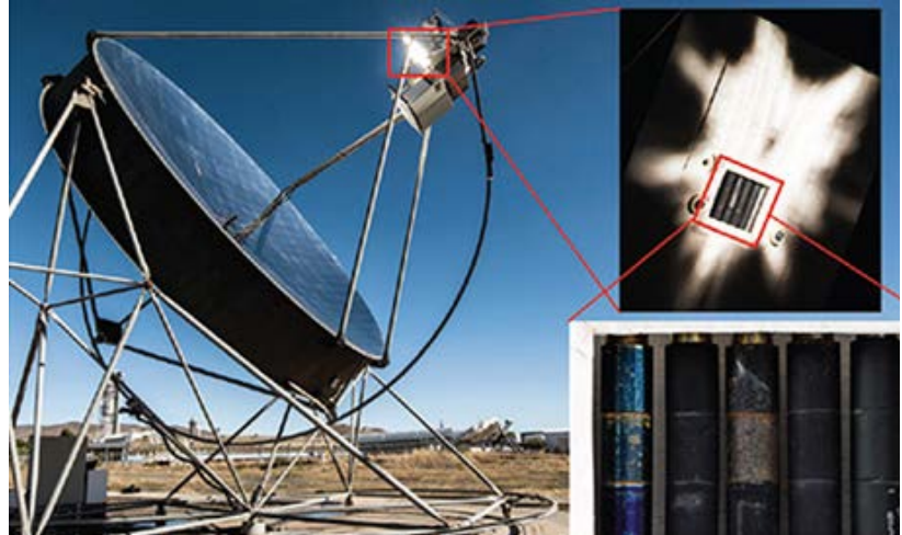
Figure 23. Accelerated aging tests of steel samples at a parabolic-dish DISTAL- II
