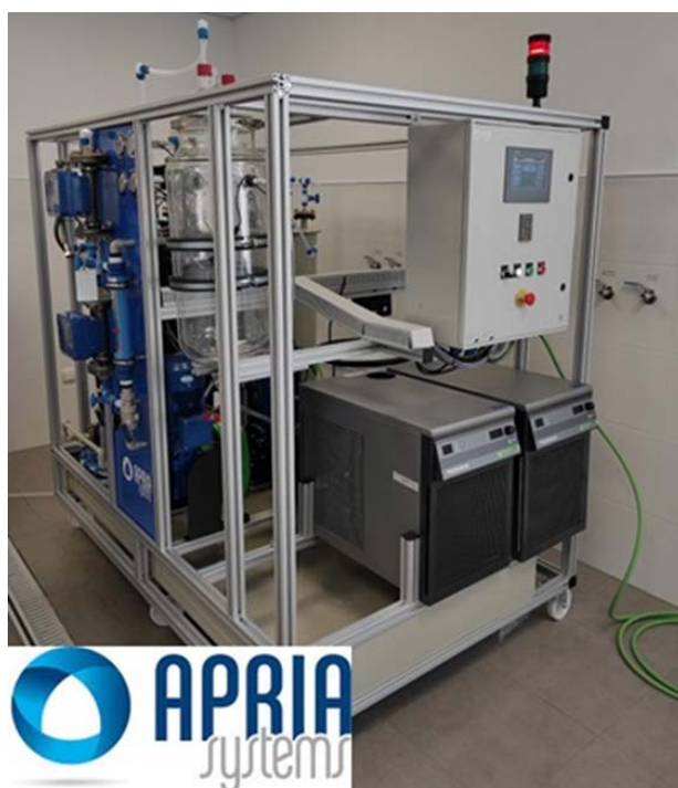
Figure 112. Membrane distillation- crystallization pilot plant installed at CIEMAT facilities.
