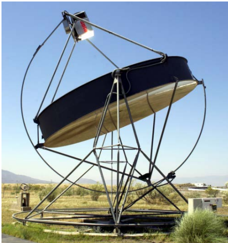
Figure 22. View of a parabolic-dish DISTAL- II with the original Stirling engine.
