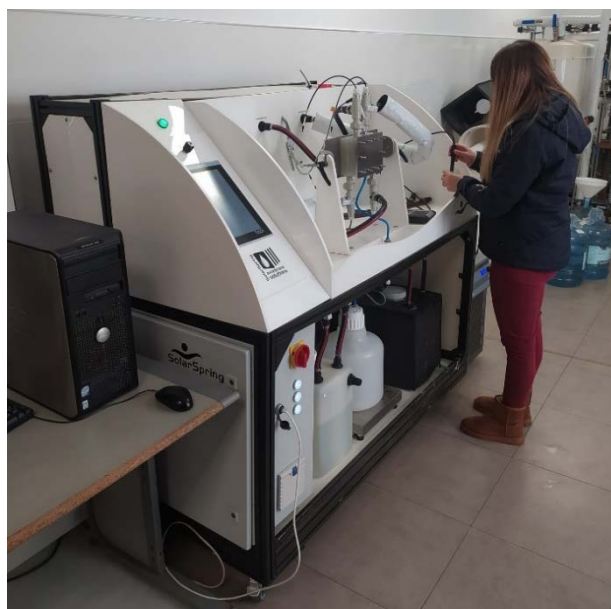
Figure 72. Bench-scale unit for testing MD with flat-sheet membranes.
