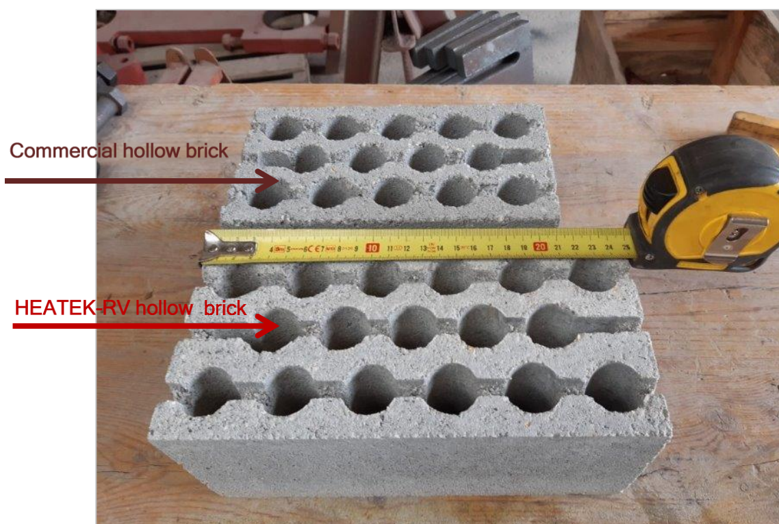
Figure 93. Comparison of geometry between a commercial hollowed brick and one using Heatek-RV®.
