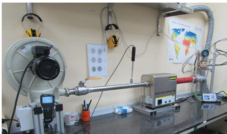
Figure 67. Test bench for pressure difference measurement with configuration up to 300°C.
