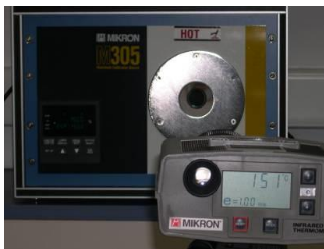
Figure 61. IR sensor calibration using a black body.
