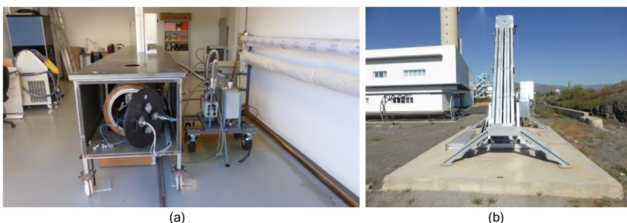
Figure 64. View of the HEATREC test chamber to measure heat losses in solar receiver tubes (a) and RESOL test bench to measure receiver's optical efficiency (b).
