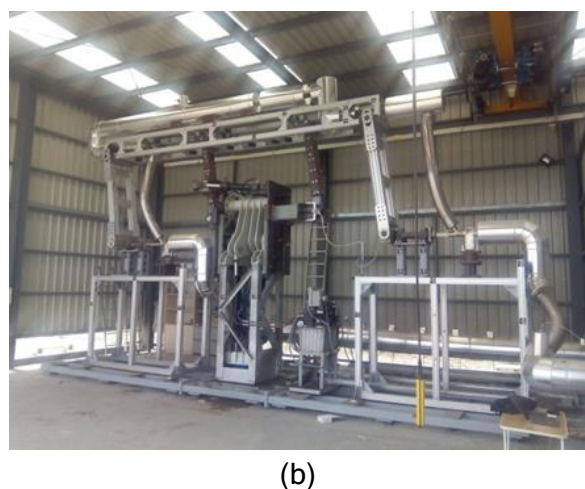
Figure 16. Schematic diagram of the REPA test loop at PSA (a) and north view of the test facility with two flex-hoses mounted for testing (b).
