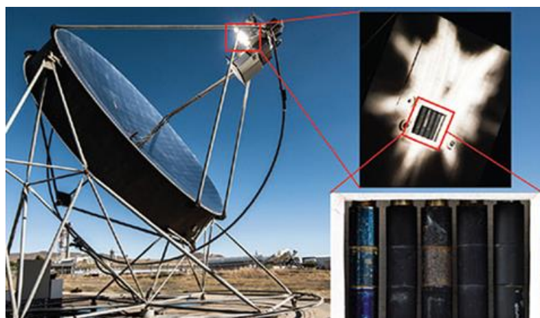
Figure 23. Accelerated aging tests of steel samples at a parabolic-dish DISTAL- II
