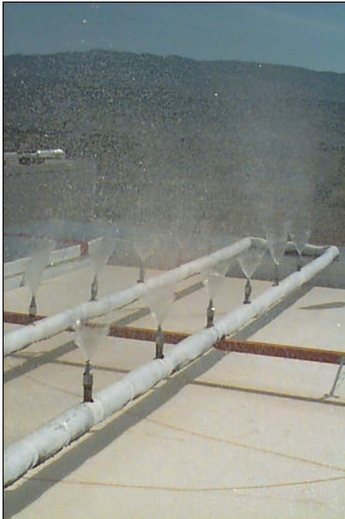
Fig 2.1.5 Evaporative roof with water sprinkler tested in the PASSYS I test cell.
