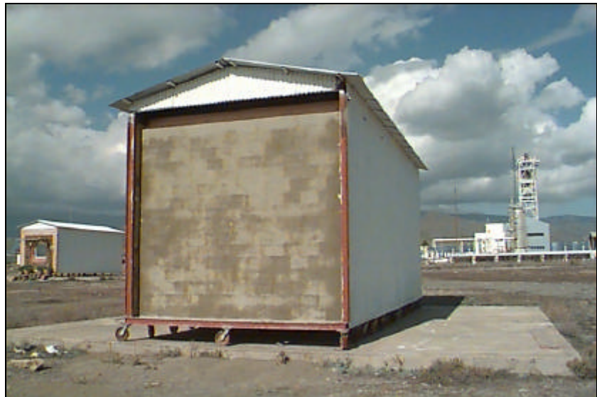
Fig. 2.1.6 Vertical component made with special bricks installed for testing in a CESPAs test cell
