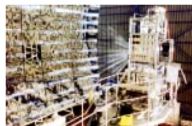
Fig. 2.4.5 The Falling-Particle-Receiver in the Solar Furnace
