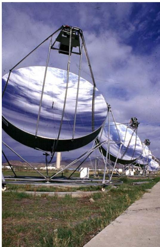
**Figure 4.2.** High concentration solar collector. Parabolic dish solar reactor (PSA, Spain)
