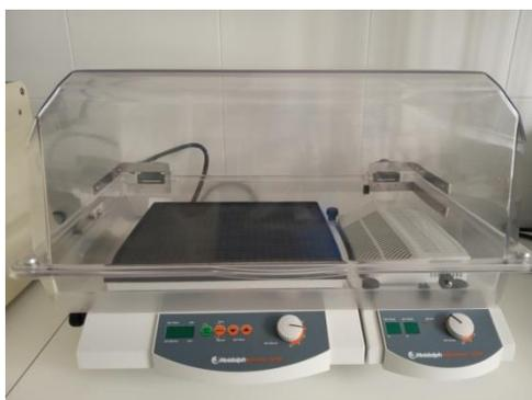
Figure 3.2. Rotary shaking incubator.
