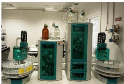
**Figure 3.18.** Photograph of ion chromatographs.
