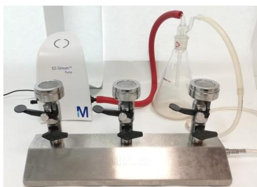
**Figure 3.4.** Microfil® filtration system.
