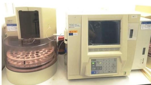
**Figure 3.19.** Photograph of TOC-analyzer.
