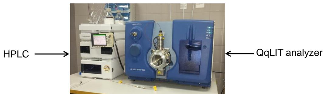
**Figure 3.9.** Photograph of HPLC-QqLIT-MS/MS equipment.
