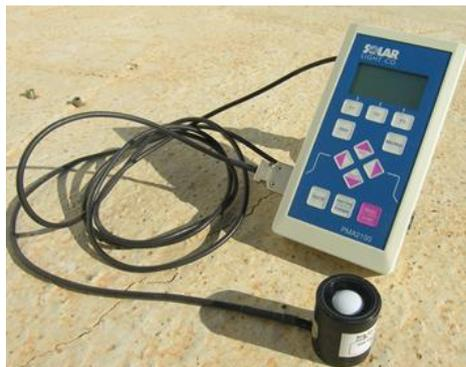
**Figure 3.16.** Portable UV-A radiometer.
