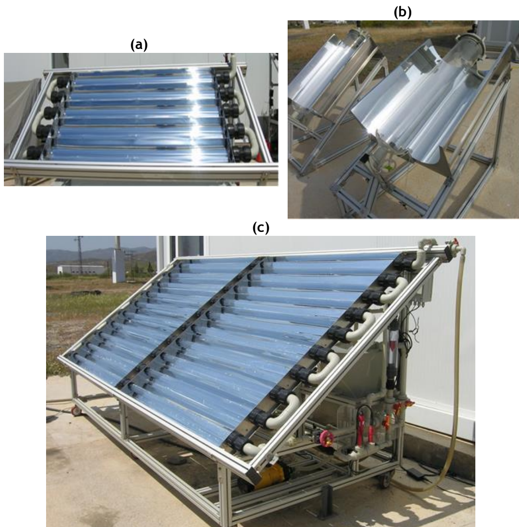
Figure 2.37. New CPC photo-reactors installed in 2010 for solar water disinfection applications: (a) CPC25, (b) CPC-SODIS and (c) FITOSOL-2.
