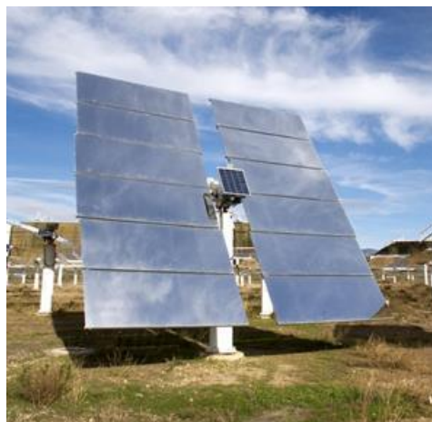
Figure 2.4. An autonomous heliostat in the CRS field
