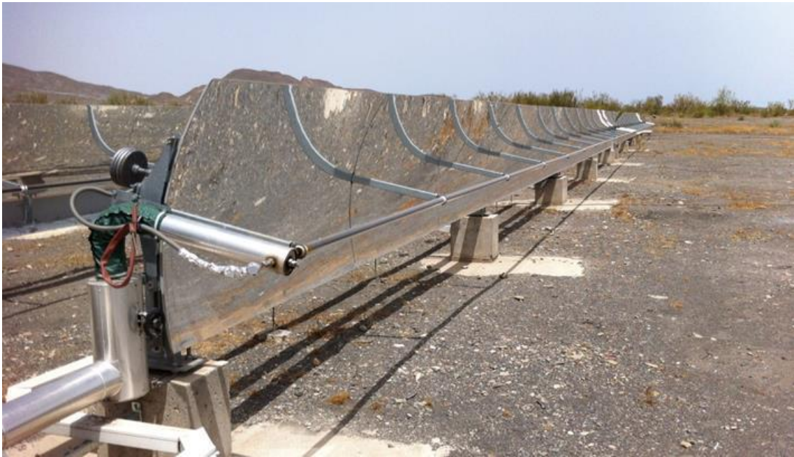
Figure 4.6: NEP PolyTrough 1200 solar collector for process heat applications up to 220 °C
