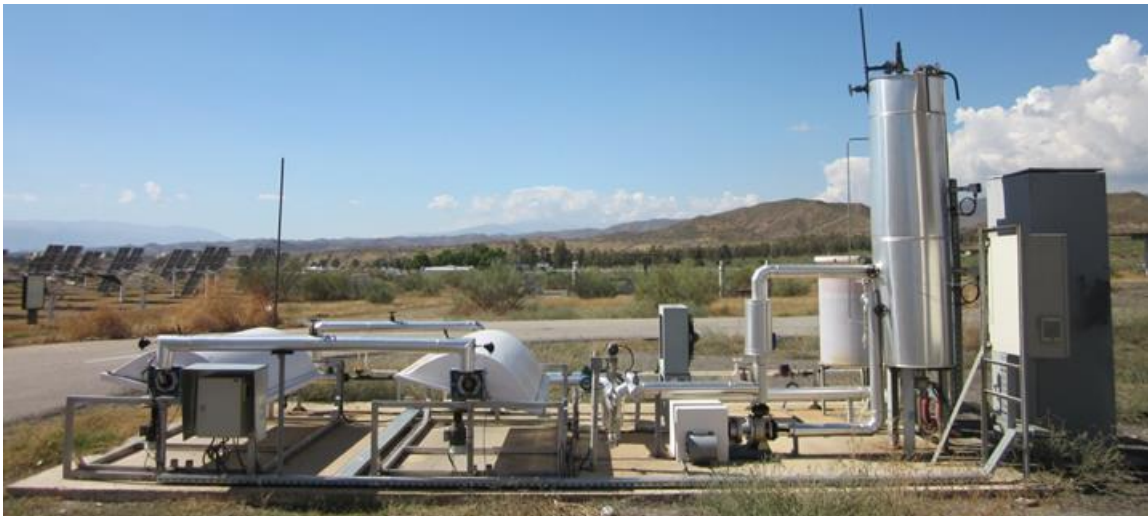
Figure 2.11. CAPSOL solar thermal test facility for small-size parabolic-trough collectors.
