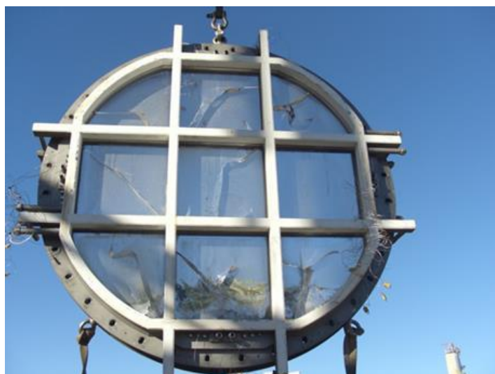
Figure 3.16. Photograph showing the reactor window after experimental tests.
