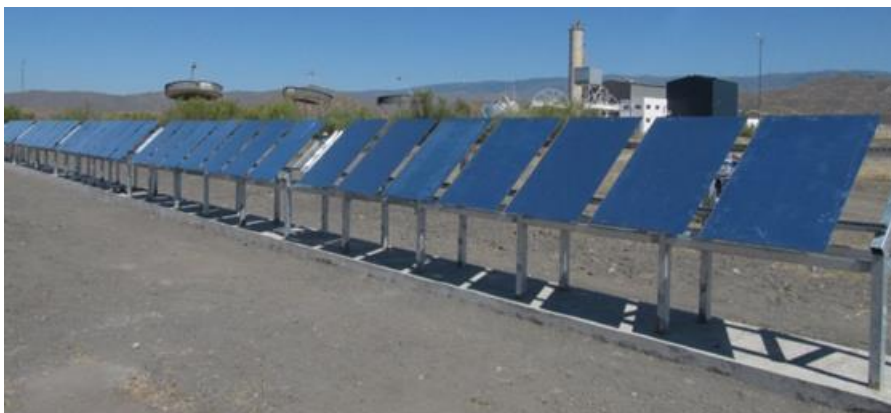
Figure 3.3. Outdoor test stand with reflector samples at PSA in Tabernas, Spain.
