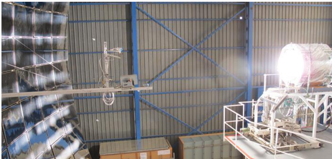
Figure 3.20. Experimental test of cylindrical volumetric solar receiver system prototype at PSA Solar Furnace
