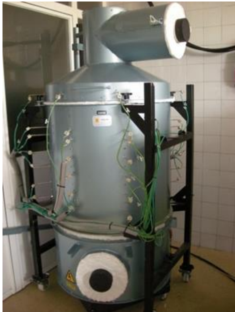
Figure 2.27. Front view of the lab-scale regenerative storage system in static arrangement
