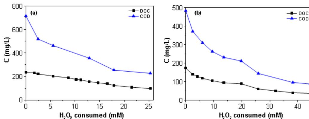
Figure 4.11. Elimination of DOC and COD during Photo-Fenton treatment of: (a) Dump lixivate pretreated in an SBBGR and (b) dump lixivate pretreated by SBBGR and ozonization.
