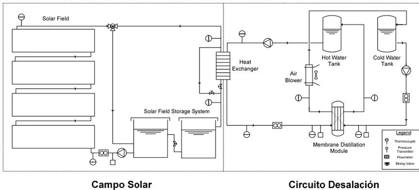
Figure 2.47. DM plant flow diagram
