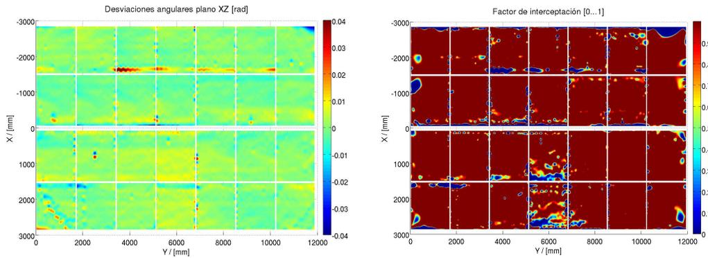
Figure 2.30. Angular deviations (left) and intercept factor of a parabolic-trough collector module analyzed by photogrammetry.
