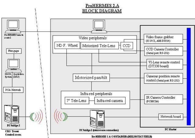
Figure 3.10. Block diagram of the ProHERMES 2.A
