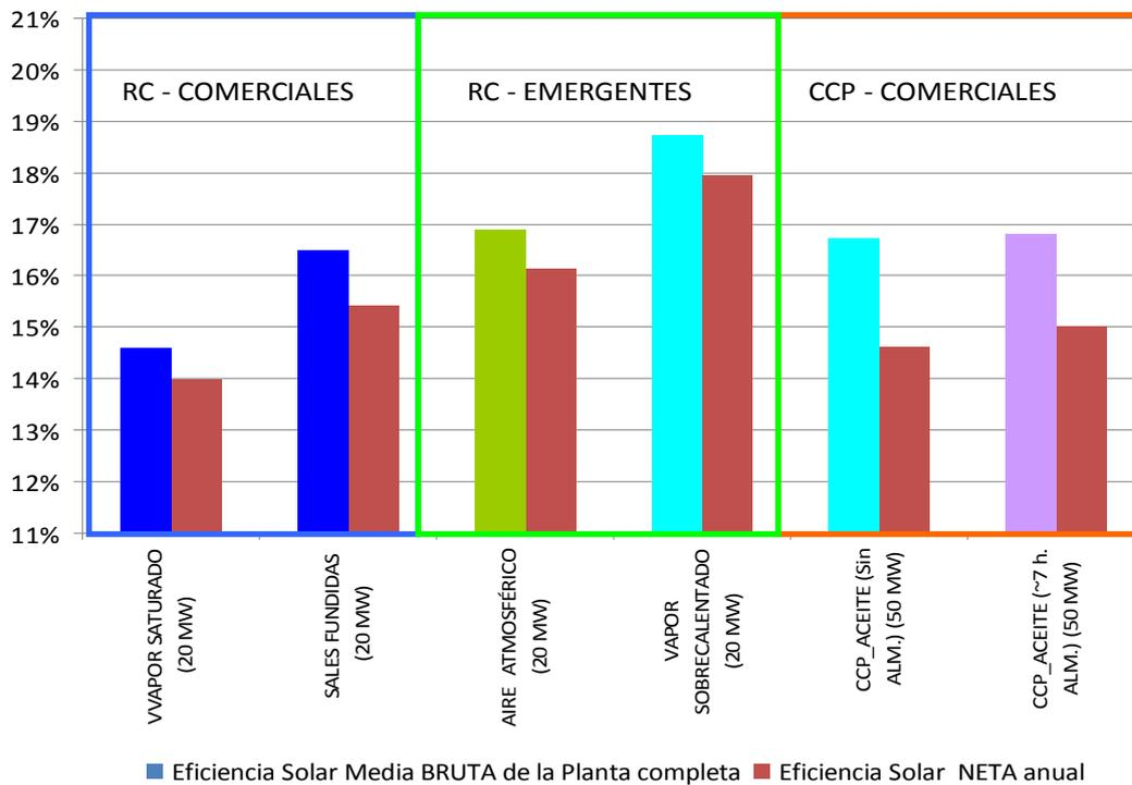
Figure 3.16. (Example) Comparative estimation of global solar-to-electric conversion efficiencies for several different technologies..
