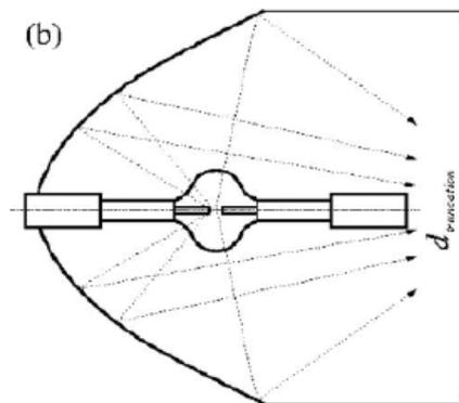
Figure 2.32. Xenon lamp used in the solar Simulator and configuration of the lamp and concentrator.
