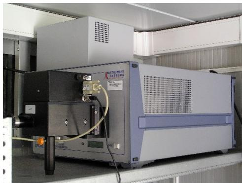
Figure 2.58. Spectroradiometer detector with three-probe connector switch
