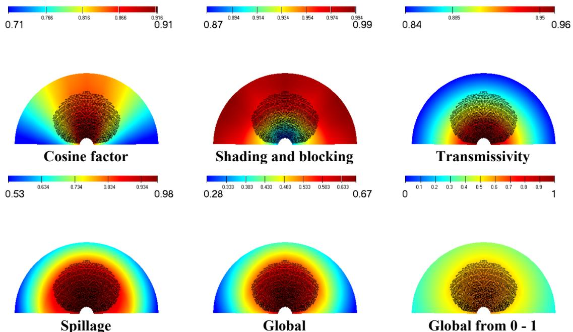
Figure 3.15. Example. Optical performance of the 50 MWe plant generated by WD along with the heliostat field proposed.
