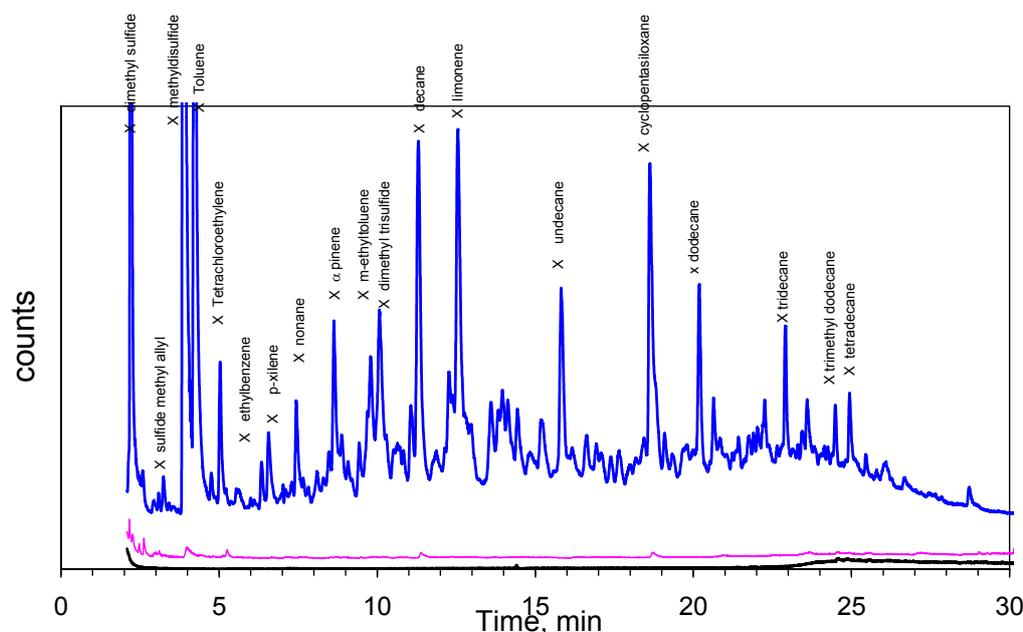
Figure 4.21. Photocatalytic treatment of real air from primary sludge in a WWTP. Chromatograms from air samples taken at the reactor inlet (blue line), and reactor outlet (pink line) and control (black line).
