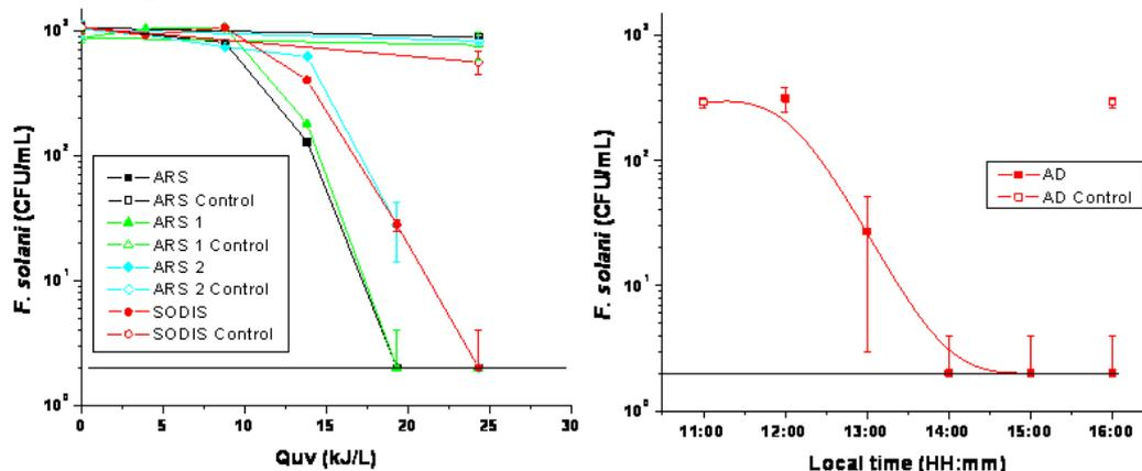
Figure 4.12. Inactivation of *F. solani* by photo-Fenton and solar radiation in : (a) lab-scale, in SWW and glass jars and (b) in DW and pilot CPC solar photoreactor plant.
