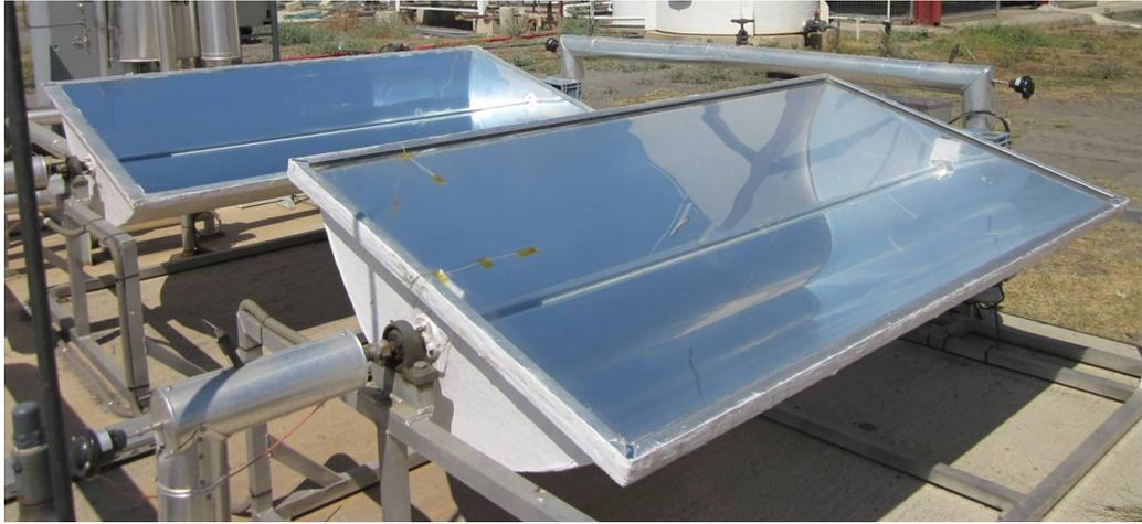
Figure 3.4. CAPSOL-02 parabolic-trough solar collector prototypes.
