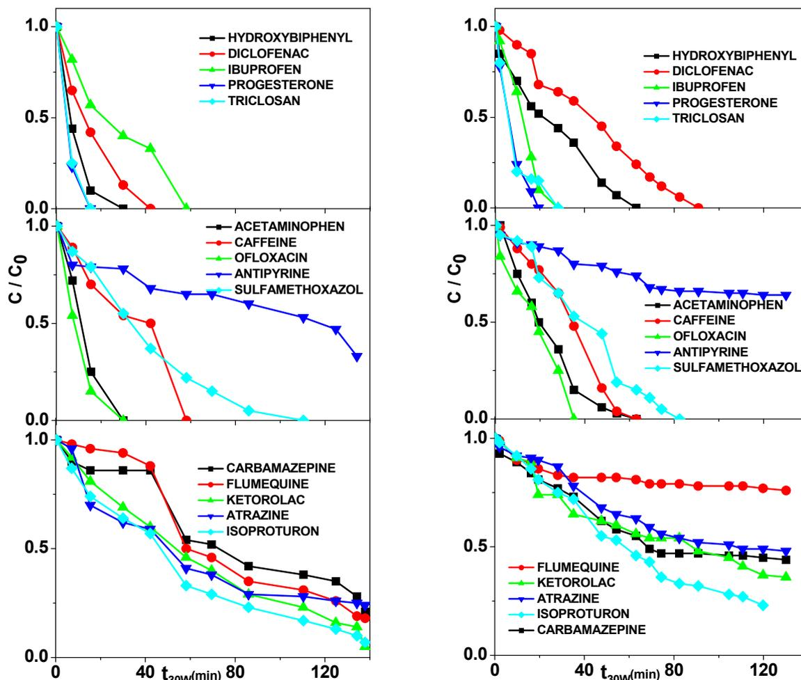
Figure 4.22. Degradation of the 15 selected compounds in real water after the 1<sup>st</sup> cycle (left) and after the 5<sup>th</sup> cycle (right).
