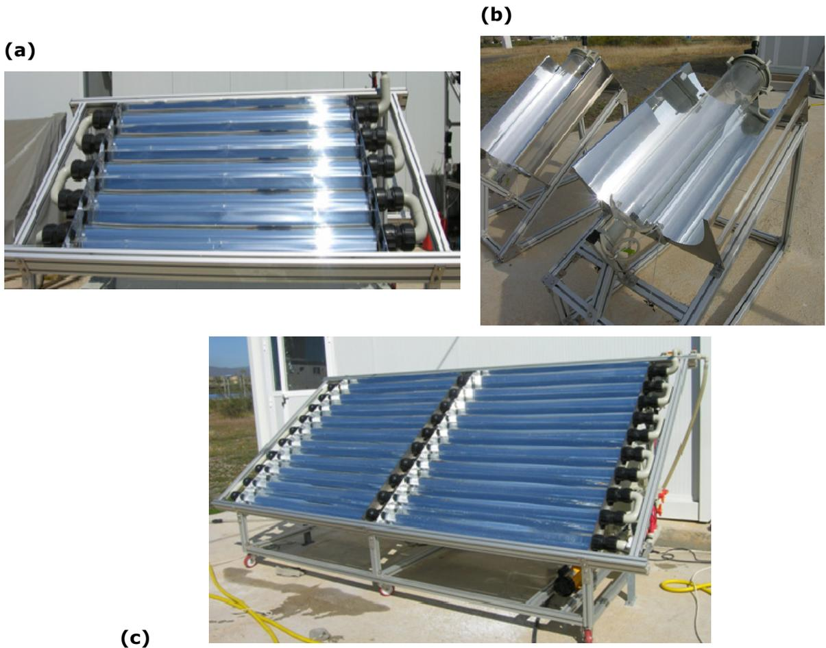
Figure 2.35. Photos of the new CPC photoreactors installed in 2010 for solar water disinfection applications: (a) CPC25, (b) CPC-SODIS and (c) FOTOSOL 2.
