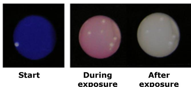
Figure 4.13. Change in color observed during exposure to sunlight of the resazurin SODIS sensor.
