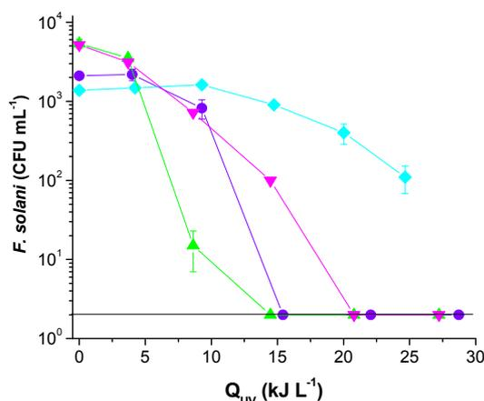
Figure 4.9. Viable *F. solani* spores over  $Q_{UV}$  under natural sunlight in the presence of 5 mg/L  $\text{H}_2\text{O}_2$  ( $\bullet$ ), 2.5 mg/L iron ( $\blacktriangledown$ ), and photo-Fenton: 2.5 mg/L iron and 5 mg/L peroxide ( $\blacktriangle$ ) concentrations compared to SODIS treatment ( $\blacklozenge$ ) (solar-only control).
