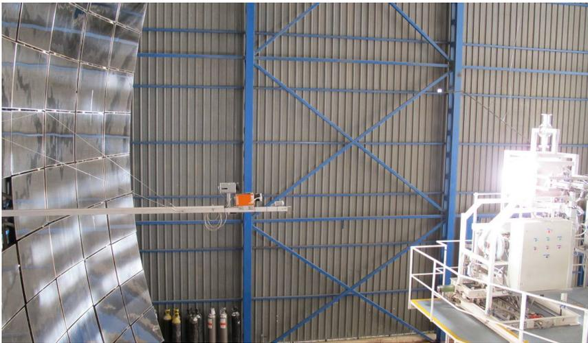
Figure 3.27. SolarPRO Project solar reactor prototype in operation in the PSA Solar Furnace.
