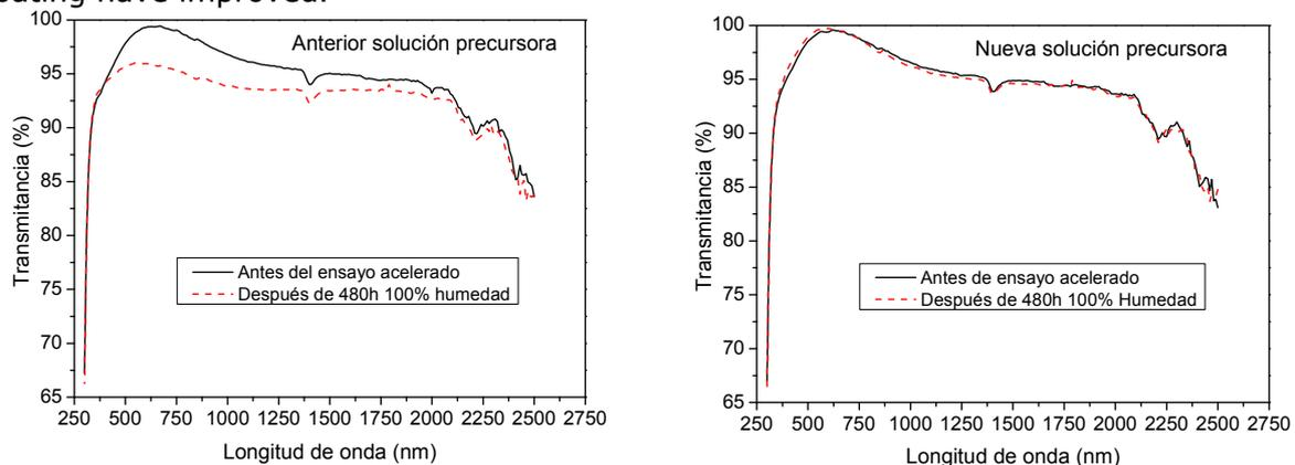
Figure 3.2. Transmittance spectra of borosilicate glass with antireflective coating prepared from the previous solution and the new solution, before and after accelerated testing according to UNE-EN-1096-2.
