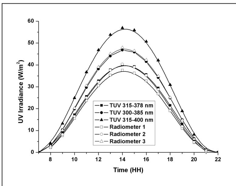
Figure 4.17. Comparison of measurements by radiometers 1 2, 3 and prediction of the TUV 4.1 model on a clear day in August 2010 at the Plataforma Solar de Almeria
