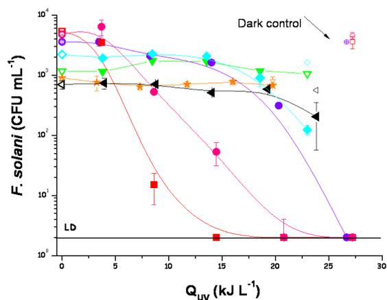
Figure 4.8. Disinfection of *solani* over  $Q_{UV}$  under natural sunlight in the presence of  $\text{Fe}^{3+}$  and  $\text{H}_2\text{O}_2$  concentrations (photo-Fenton system) of 1 mg/L and 2.5 mg/L ( $\bullet$ ); 2.5 mg/L and 5 mg/L ( $\blacksquare$ ); 5 mg/L and 10 mg/L ( $\bullet$ ); 10 mg/L and 10 mg/L ( $\blacktriangleleft$ ); and 50 mg/L and 10 mg/L, respectively ( $\blacktriangledown$ ), compared to SODIS treatment ( $\blacklozenge$ ) (solar-only control).
