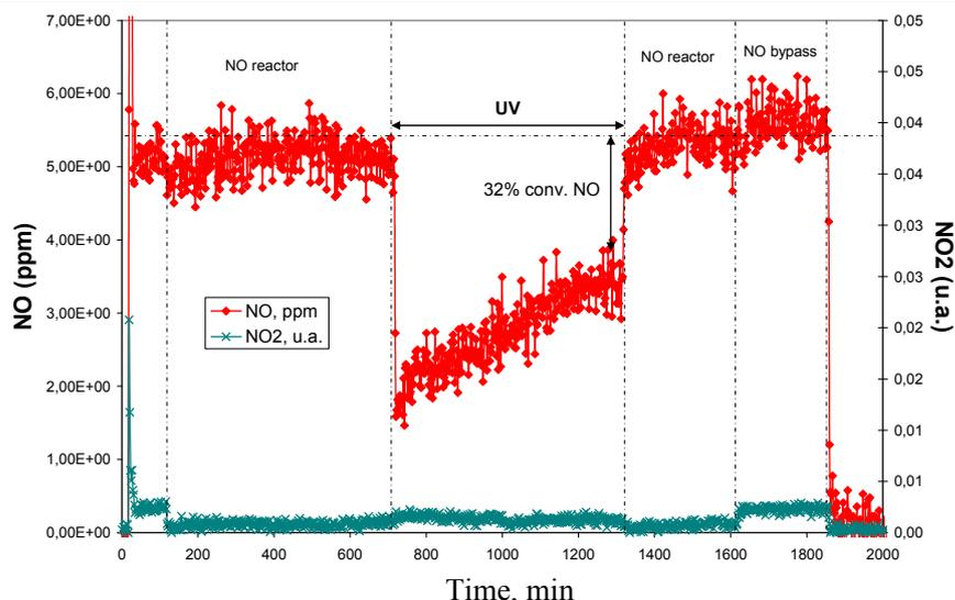
Figure 4.20. Variation in concentration of NO and NO<sub>2</sub> during photocatalytic degradation of NO for one of the photocatalytic asphalts tested.
