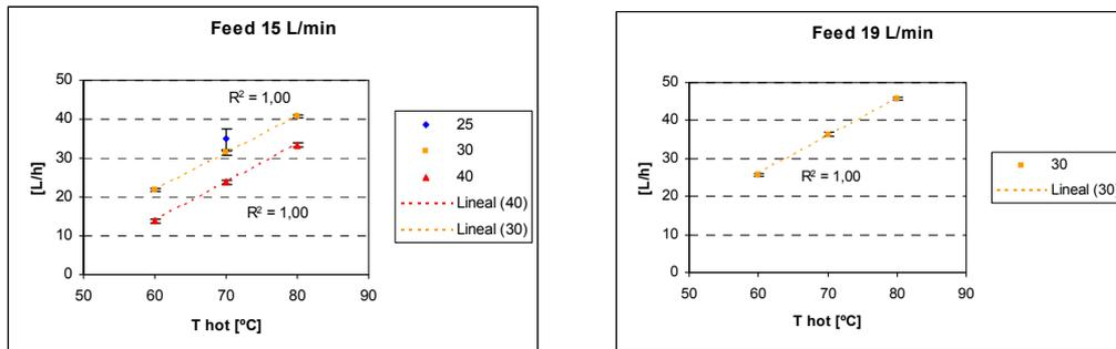
Figure 4.26. Production of permeate as a function of feedwater temperature at different flow rates. Three modules operating in series.
