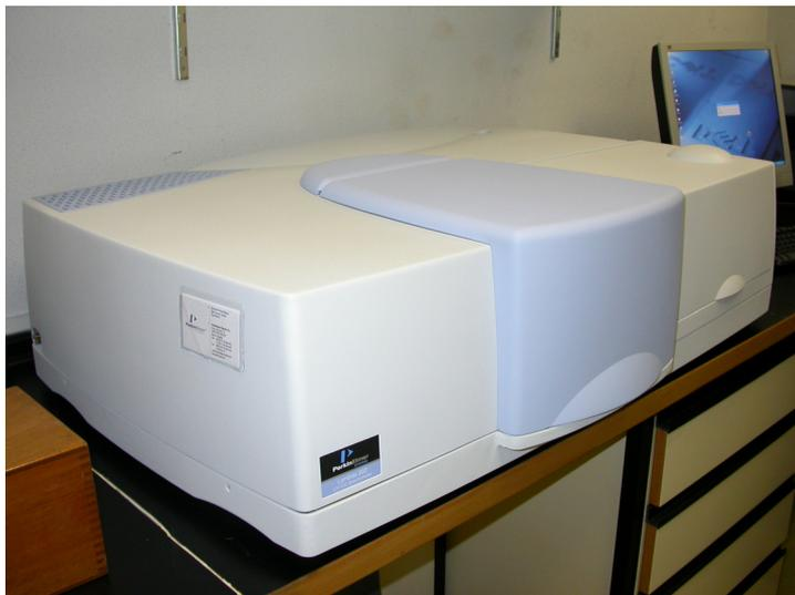
Figure 2.21. . Perkin Elmer Lambda 950 Spectrophotometer
