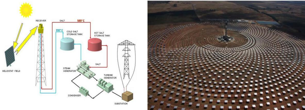
Figure 3.7. Flow diagram of the GEMASOLAR plant and construction site in 2010.
