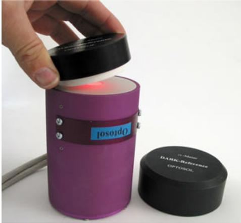
Figure 2.23. Optosol integrating sphere for measuring solar absorptance
