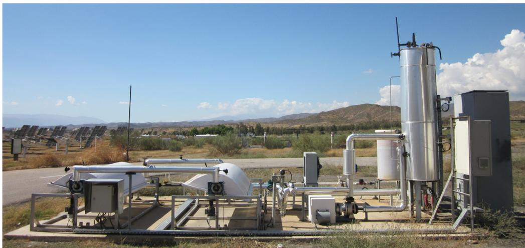
Figure 2.11. CAPSOL solar thermal test facility for small-size parabolic-trough collectors.
