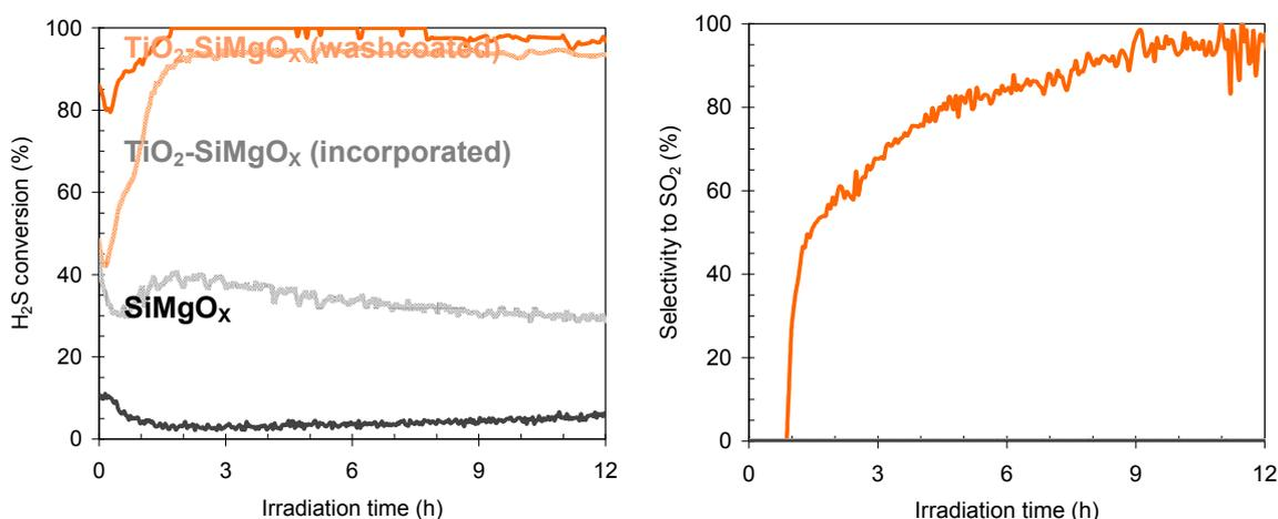
Figure 4.23. Conversion (left) and selectivity (right) during photocatalytic oxidation of  $\text{H}_2\text{S}$  with pure  $\text{SiMgO}_x$  and P25- $\text{TiO}_2$  or hybrid  $\text{TiO}_2$ - $\text{SiMgO}_x$  incorporated and coated, all treated at  $500^\circ\text{C}$ .
