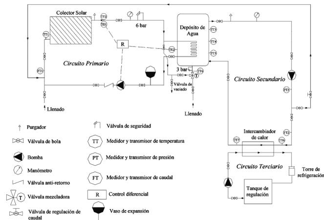
Figure 2.51. General layout of the stationary solar collector test platform
