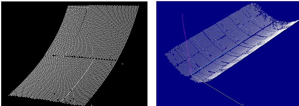
Figure 2.29. Three-dimensional models of a parabolic-trough facet (left) and a complete module found by photogrammetry.
