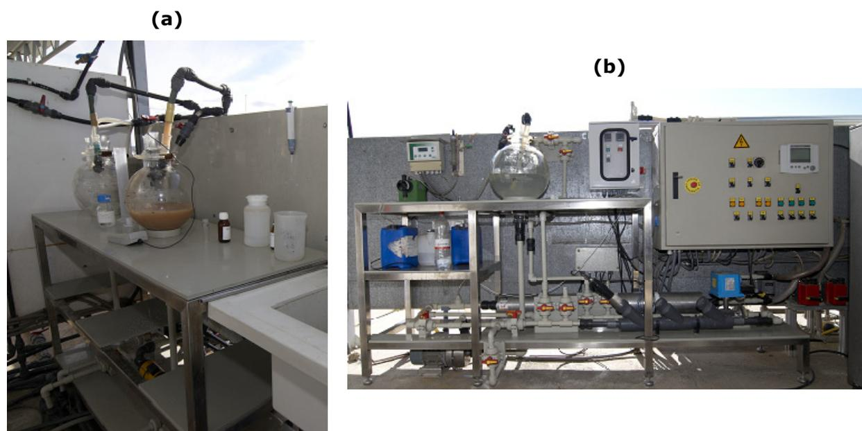
Figure 2.34. Photos of the auxiliary facilities and instrumentation remodelled in the CPC photoreactors (a) SOLEX and (b) CADOX.
