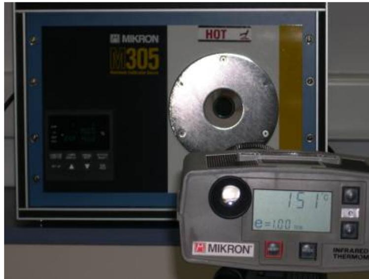
Figure 3.17. Calibration of IR detector in laboratory.
