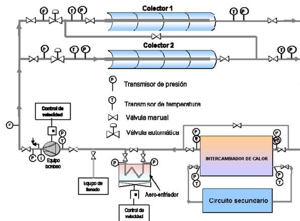
Figure 2.9. Simplified system diagram of the innovative fluids experimental facility.
