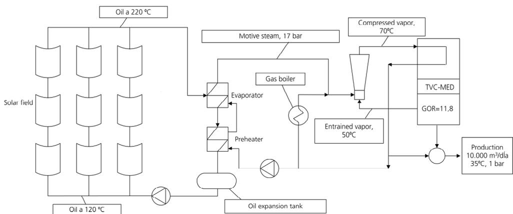
Figure 4.29. Diagram of the system made up of a TVC-MED plant connected to a PTC solar field.
