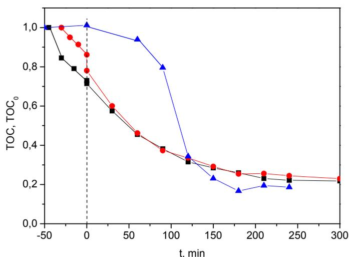
Figure 4.14. Elimination of TOC in the mixture of compounds in water at a concentration of 10 ppm using the sunlight/TiO<sub>2</sub> with and without the preliminary treatment. Symbols: ● elimination of compounds by ozonation; ▲ without preliminary ozonation.
