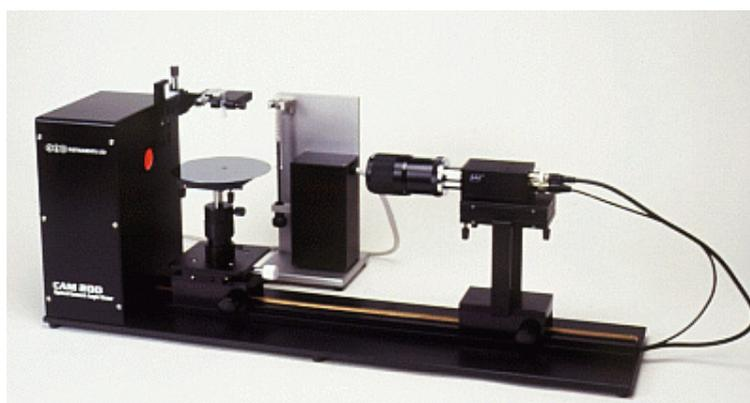
Figure 2.27. Goniometer for measuring contact angles
