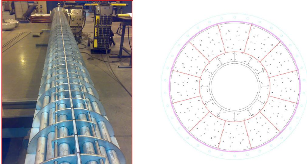
Figure 3.22. View of the exchanger located at the output of the SYNPET reactor and configuration in the brick-shaped receiver aperture.
