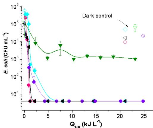
Figure 4.6. *E. coli* over time of exposure to sunlight in the presence of 1 mg/L ( $\bullet$ ), 5 mg/L ( $\circ$ ), 10 mg/L ( $\blacktriangleleft$ ) and 50 mg/L ( $\blacktriangledown$ )  $Fe^{3+}$  concentrations compared to SODIS treatment ( $\blacklozenge$ ) (solar-only control).
