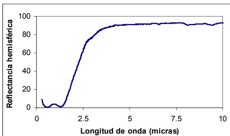
Figure 3.3. Complete spectrum of the selective absorber developed at CIEMAT
