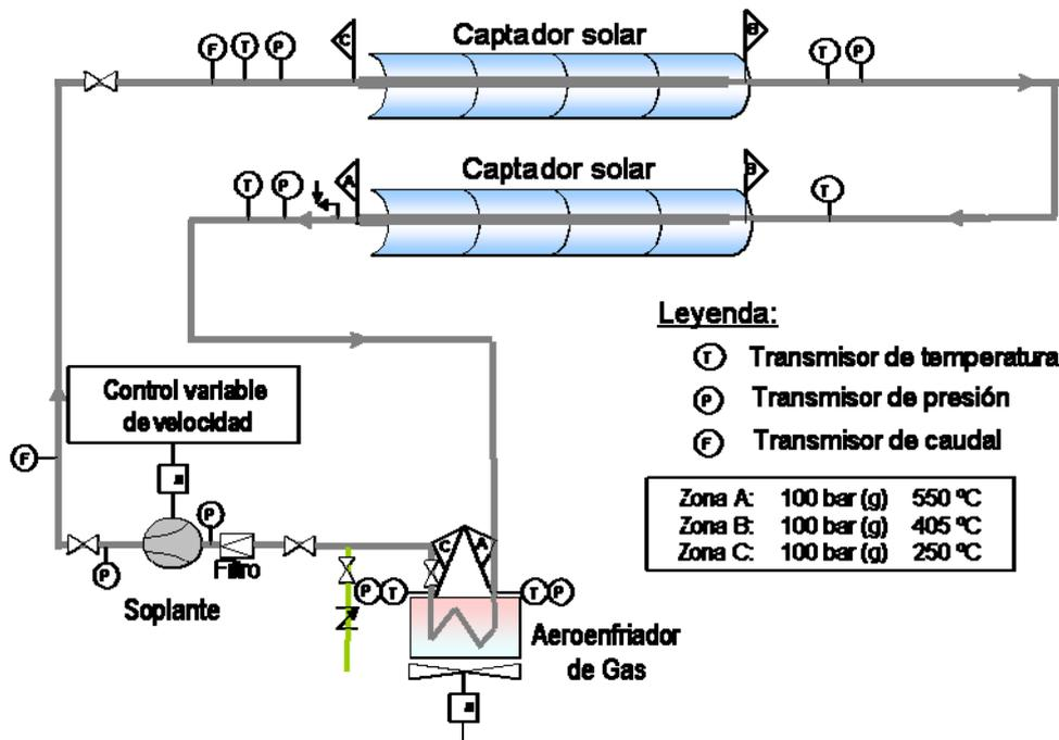
Figure 3.5. Diagram of the new configuration of the test loop installed at the PSA for the experimental study of pressurized gas as the working fluid in parabolic-trough collectors.
