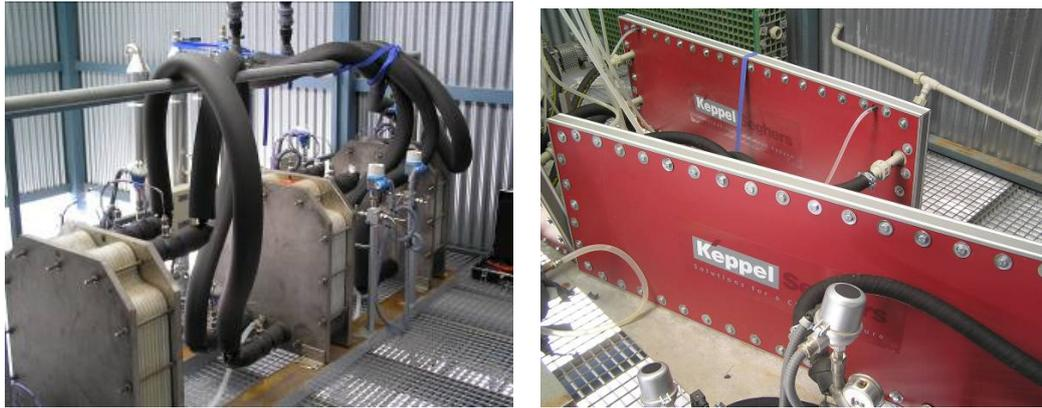
Figure 2.48. Characterized membrane distillation modules in the plant; at the left: Scarab AB module; at the right: Keppel Seghers module.
