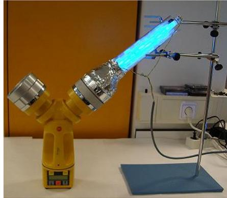
Figure 2.43. Air impactor for biological sampling connected to a photocatalytic disinfection reactor
