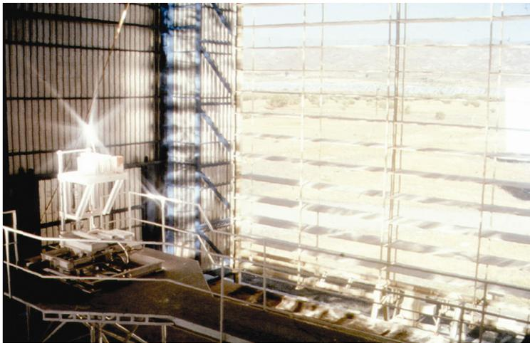
Figure 2.19. The focus and the test table, on the left. On the right, the completely open shutter allows the rays from the heliostats outside to come in.
