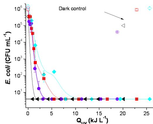
Figure 4.7. Disinfection of *E. coli* over QUV under natural sunlight in the presence of 2.5 mg/L ( $\blacksquare$ ), 5 mg/L ( $\bullet$ ) and 10 mg/L ( $\blacktriangleleft$ )  $H_2O_2$  concentrations compared to SODIS ( $\blacklozenge$ ) (solar-only control).
