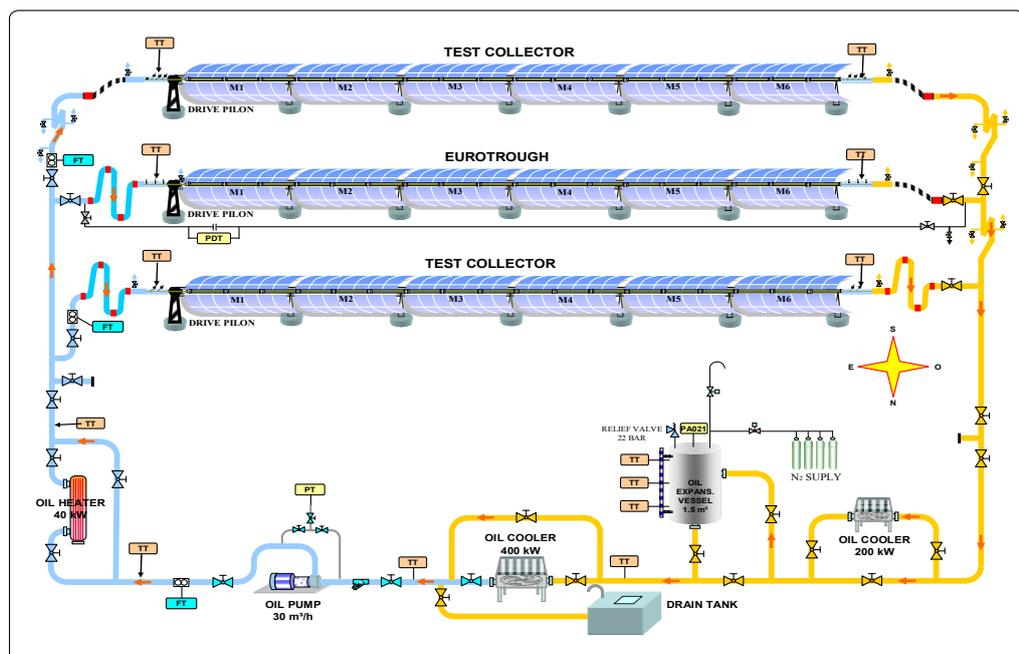
Figure 2.5. Diagram of the “HTF Loop” parabolic-trough solar collector test loop facility
