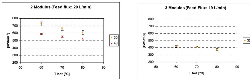
Figure 4.27. Specific thermal energy consumption [kWh<sub>t</sub> m<sup>-3</sup>]. Results operating with 2 and 3 DM modules in series.
