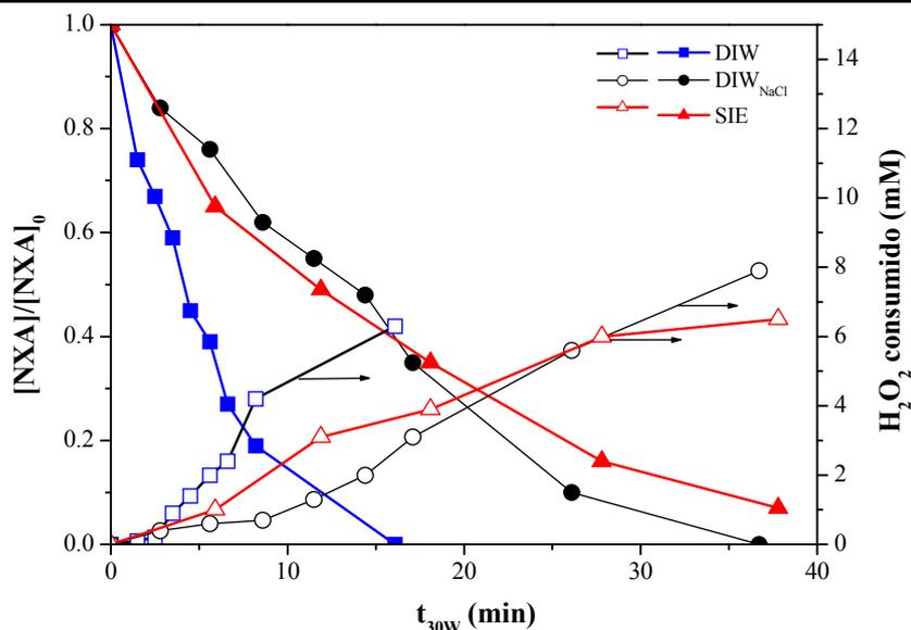
Figure 4.4. Degradation of nalidixic acid (NXA) and hydrogen peroxide consumption during photo-Fenton treatment in waste water with different salt content: deionized water (DIW), natural water (SIE) and water with 5 g/L of NaCl (DIW<sub>NaCl</sub>)
