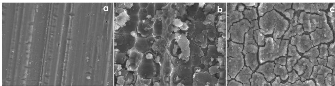
Figure 4.24. SEM images. A) Washed aluminum b) Pretreated aluminum c) Pretreated aluminum coated with TiO<sub>2</sub>.
