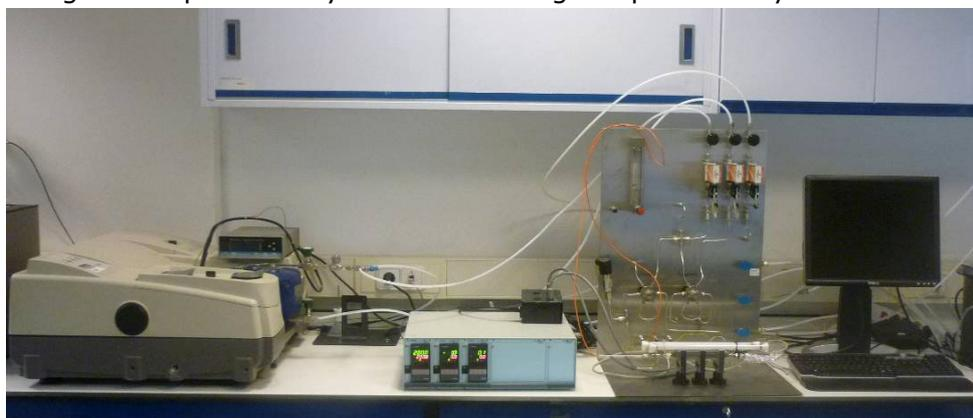
Figure 2.40. Automatic photocatalysis test bed with UV radiation connected to an FT-IR system for analysis of re
