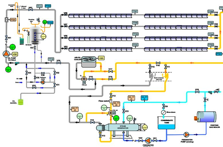
Figure 2.54. Polygeneration facility layout
