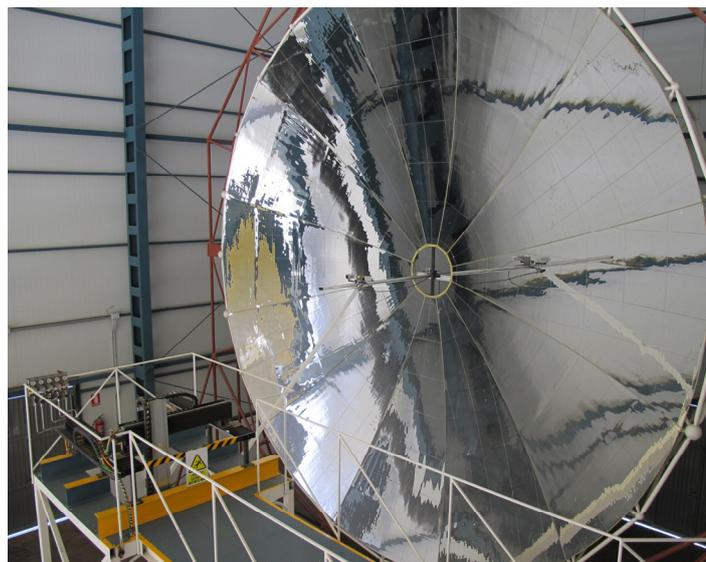
Figure 2.17. Interior of the SF40 solar furnace in its final stage of construction
