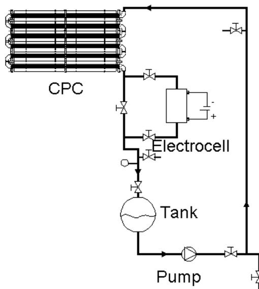
Figure 4.3. Drawing of the new photoelectrochemical reactor installed at the PSA.
