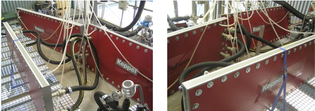
Figure 4.25. Second membrane distillation prototype (Keppel-Seghers, Singapore) tested at the PSA facility.
