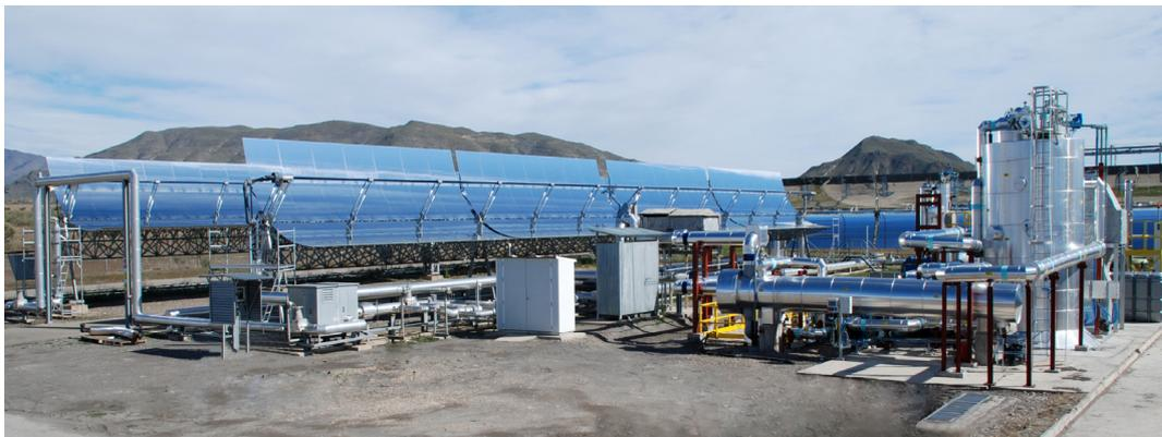
Figure 2.8. View of the pressurized gas test loop connected to a molten salt thermal storage system.
