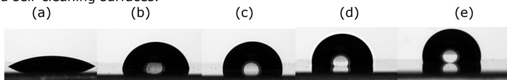
Figure 2.26. Photos showing how the angle of contact varies as a function of the hydrophobicity of the substrate.
