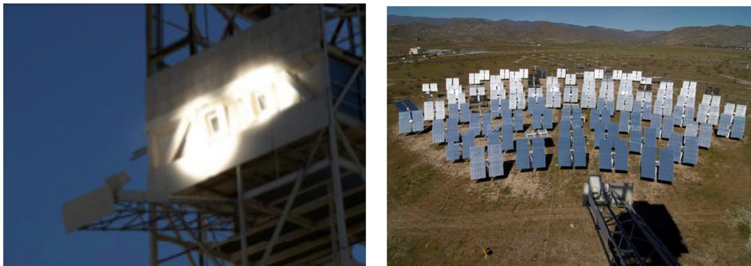
Figure 3.25. Left: Detail of the two HYDROSOL-II reactor apertures in operation. Right: View of the SSPS heliostat field as seen from one of the HYDROSOL-II reactor apertures
