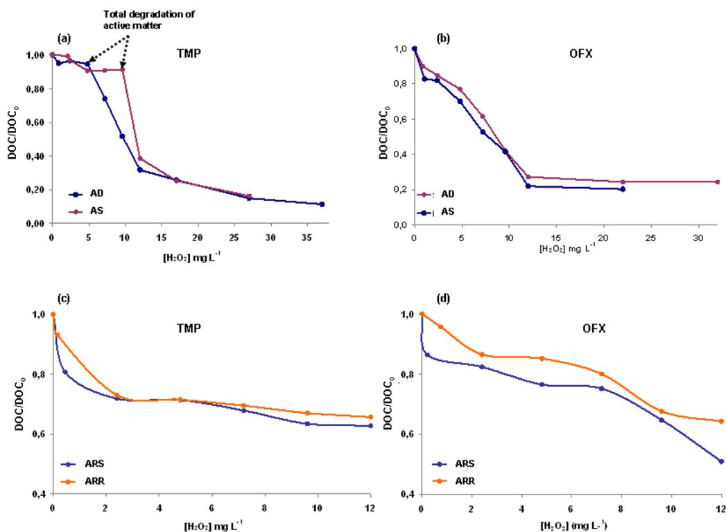
Figure 4.10. Degradation trimetroprin (TMP) and ofloxacin (OFX) by photo-Fenton for each type of matrix used: (a) TMP: DW and SW; (b) OFX: DW and SW; (c) TMP: SWW and RWW; (d) OFX: SWW and RWW.
