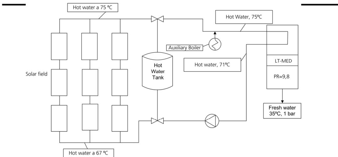
Figure 4.28. Diagram of the system made up of an LT-MED plant connected to a field of ETCs.
