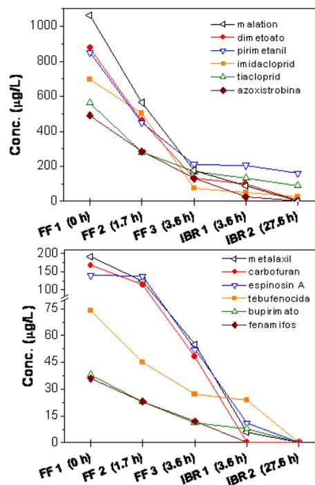
Figure 4.5. Evolution of the concentration of pesticides contained in real water during the combined Photo-Fenton/biological treatment ( $\text{COD}_0$ : 480 mg/L). Treatment times of each sample are included.
