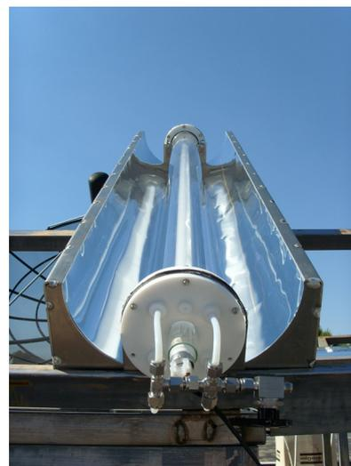
Figure 2.39. Hybrid solar/lamp photoreactor/with compound parabolic-trough collector (CPC)
