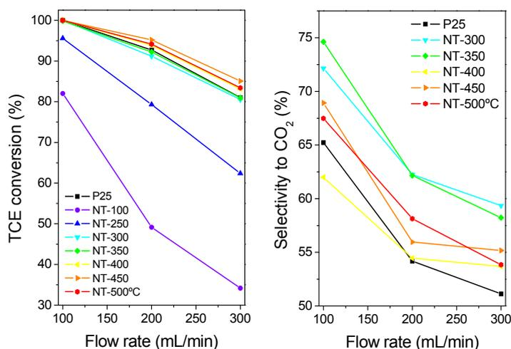
Figure 4.19. Effect of calcination temperature on TCE conversion and  $\text{CO}_2$ -selectivity of one of the sample nanotubes synthesized.
