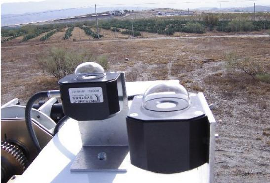
Figure 2.57. Spectroradiometer probes for measuring global and diffuse radiation installed in the solar tracker
