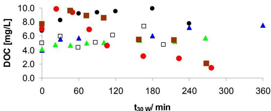
Figure 4.15. Mineralization of progesterone solutions treated under different conditions. Sunlight-only (□), Anodic oxidation (AO) at 10 A (▲), AO+sunlight at 10 A (▲), electroFenton (EF) at 10 A (●), and photo-electro-Fenton (FEF) at 10 A (●) and at 15 A (■).
