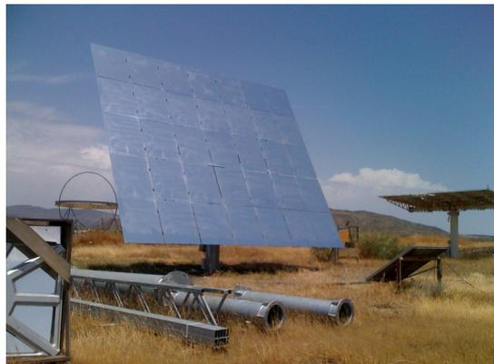
Figure 3.9. Front view of the SATOHE heliostat in normal tracking
