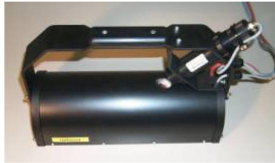
Figure 2.24. Accessory for thermal emissivity measurement at 70°C.
