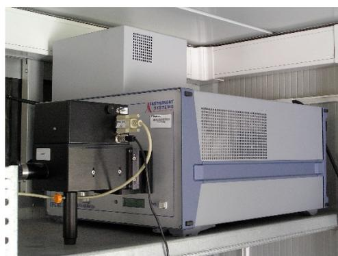
Figure 2.34. Spectroradiometer detector with three-probe connector switch
