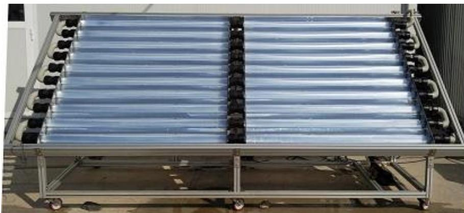
Figure 2.18. Disinfection CPC photoreactors installed in November 2008.
