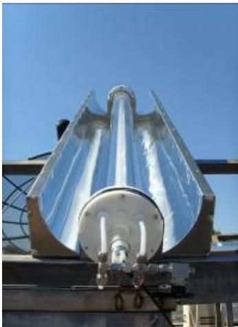
Figure 4.18. Hybrid photoreactor for continuous treatment of gas emissions
