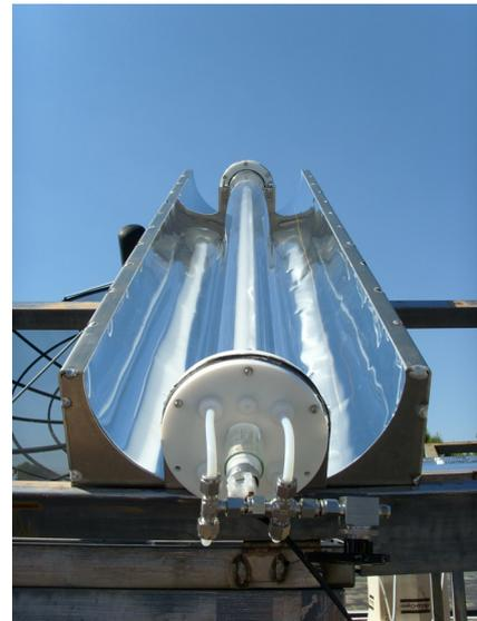
Figure 2.26. Hybrid solar/lamp reactor with CPC
