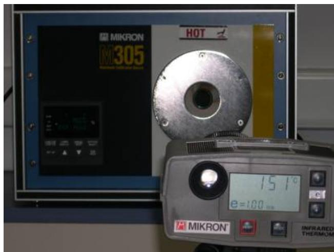
Figure 3.22 Calibration of an IR detector in the laboratory
