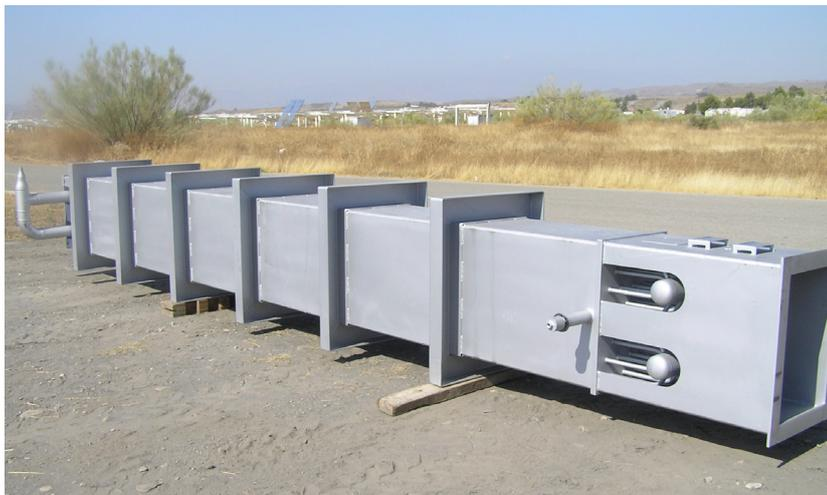
Figure 3.1 General view of the new PCM storage module to be installed and tested at the PSA in 2010.
