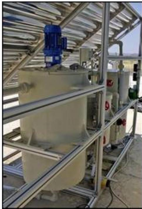
Figure 2.17. Biological system underneath one of the CPC photoreactors
