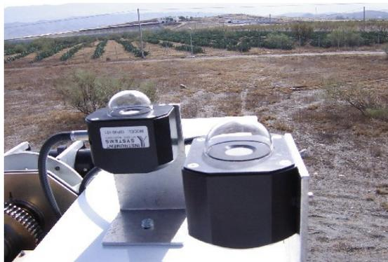
Figure 2.33. Spectroradiometer probes for measuring global and diffuse radiation installed in the solar tracker
