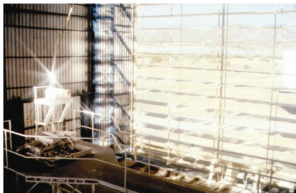
Figure 2.15. The focus and the test table, on the left. On the right, the completely open shutter allows the rays from the heliostats outside to come in.
