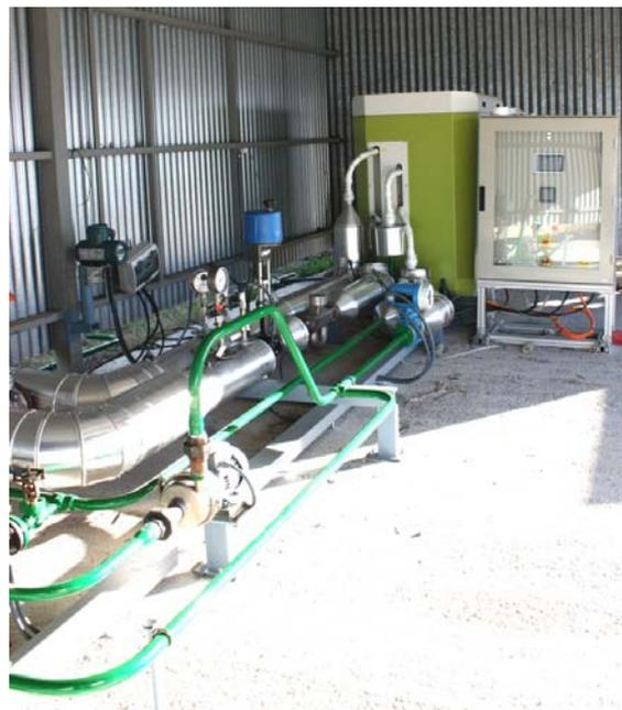
Figure 4.25. PSA organic Rankine cycle test bed
