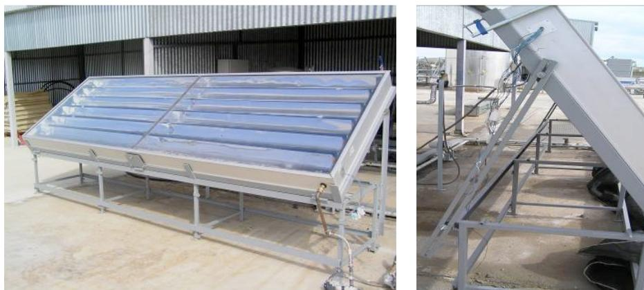
Figure 4.24. Experimental evaluation of the CPC 1.5x collector prototype
