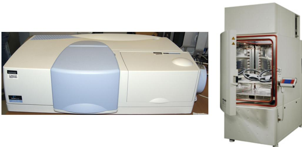
Figure 3.11 Perkin Elmer Lambda 1050 spectrophotometer (left) and Atlas SC340 weathering chamber (right) in the solar reflector materials lab.
