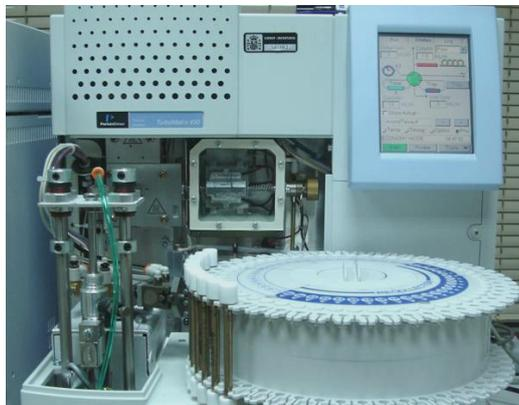
Figure 2.27. ATD-GC-MS for analysis of air in interiors
