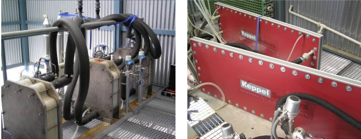
Figure 2.21. Characterized membrane distillation modules in the plant; at the left: Scarab AB module; at the right: Keppel Seghers module.
