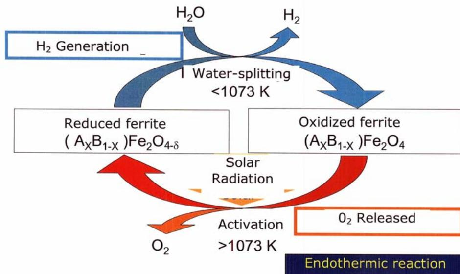
Figure 3.24 Schematic diagram of the ferrite cycle for H<sub>2</sub> production selected in the SOLTER project.
