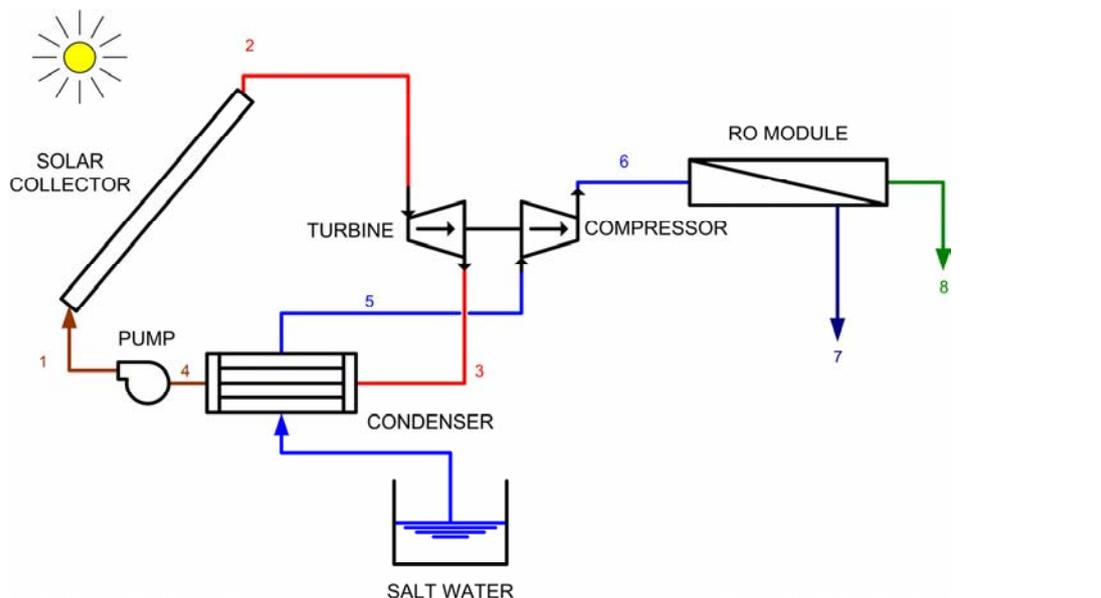
Figure 4.16 Generic reverse osmosis system hooked up to a solar driver
