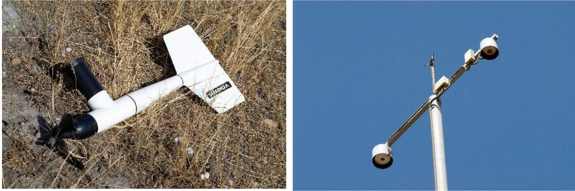
Figure 4.18 Damage by lightning. The anemometer at the top of the mast was knocked off
