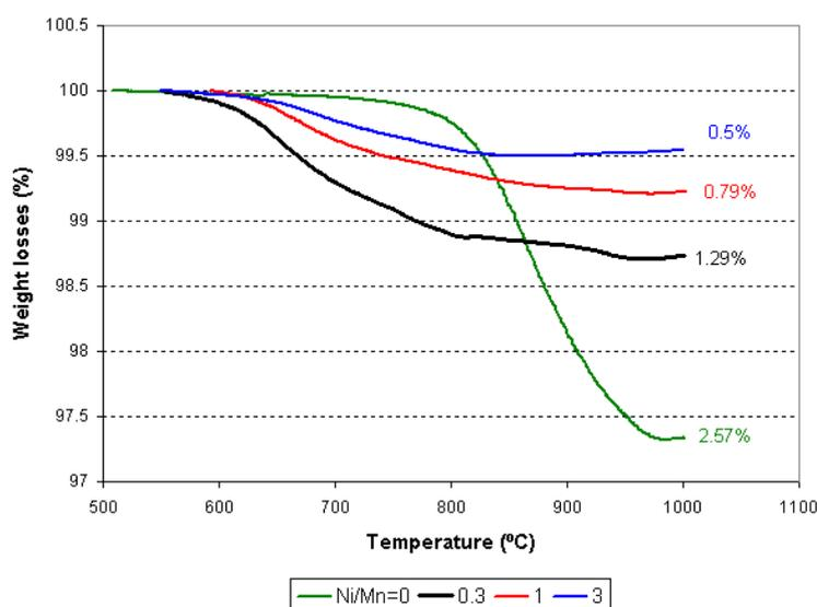
Figure 3.25 Activation stage weight loss testing done in the thermogravimetric balance, with weightloss over temperature for mixed ferrite Ni<sub>x</sub>Mn<sub>1-x</sub>Fe<sub>2</sub>O<sub>4</sub> samples (with nitrogen carrier and heat ramp of 20°C/min)
