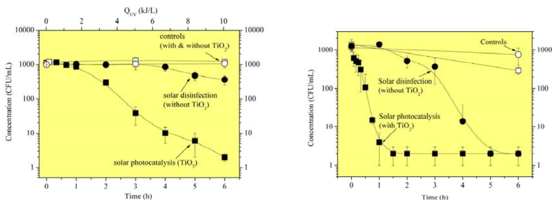
Figure 4.7 Degradation of *Fusarium equiseti* spores (left) and *Fusarium verticillioides* (right) by solar irradiation and solar photocatalysis with TiO<sub>2</sub> in suspension (35 mg/L) under natural solar radiation at the Plataforma Solar de Almería (right [4.5]).
