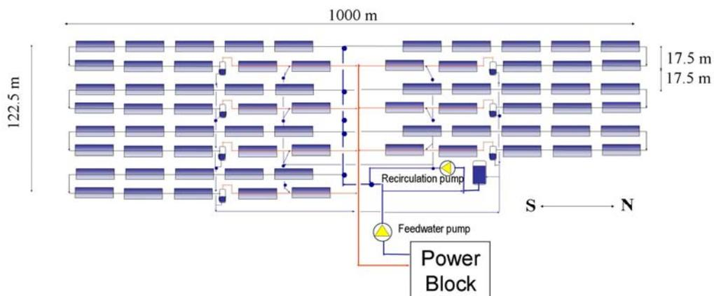
Figure 3.2 Schematic diagram of the 3 MW<sub>e</sub> Almería DSG plant.
