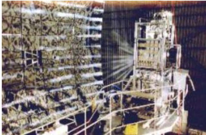
Figure 2.12 Solar Furnace: Concentrator (left) and receiver in operation at the focus (right).
