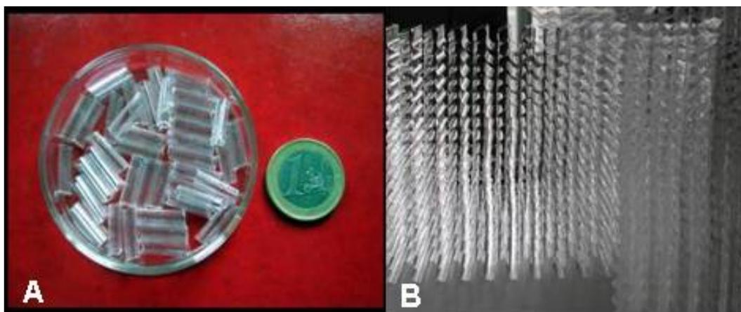
Figure 4.11 Some examples of the supports used to deposit  $\text{TiO}_2$  on A) borosilicate glass tubes; B) polymeric monoliths
