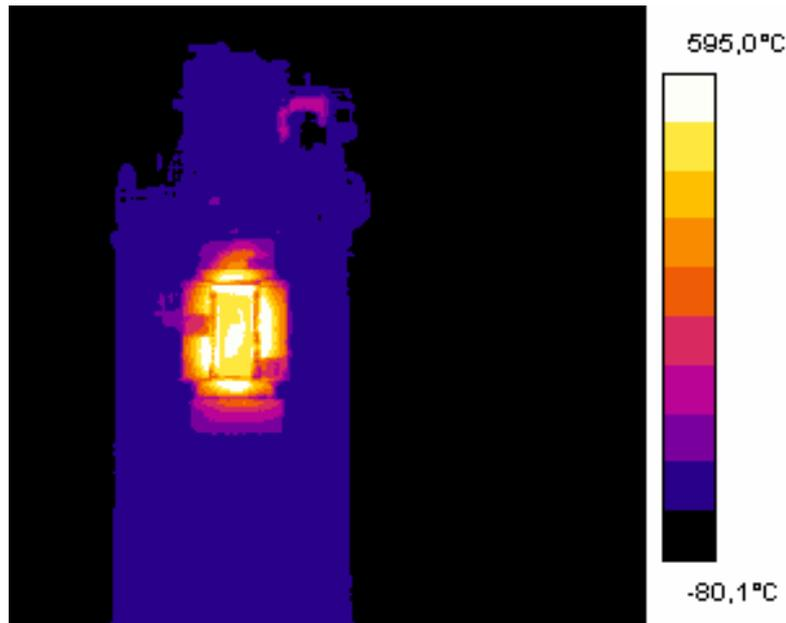
Figure 3.10 Infrared image of first salt receiver panel tests in the CESA-1 tower.
