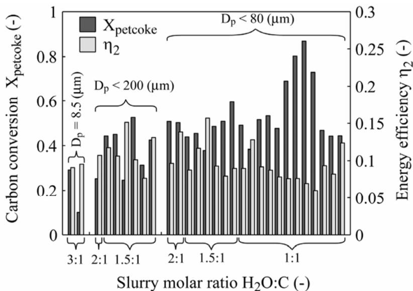
Figure 3.23 Chemical conversion of petcoke and energy efficiency of the conversion in solar tests in order by particle size and stoichiometry of the slurry.
