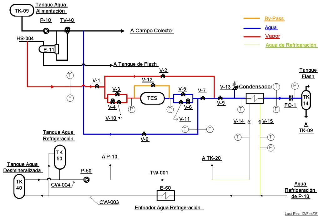
Figure 3.1 Schematic of the interface designed to connect the DISTOR storage module to the PSA DISS experimental plant.
