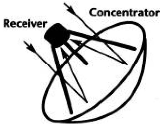
Figure 2.8 Schematic diagram of a parabolic dish with Stirling motor at the focus
