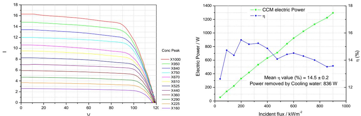
Figure 3.13 IV curves for the CCM tested at different concentrations in the solar furnace; delivered electric potential and efficiency curves.
