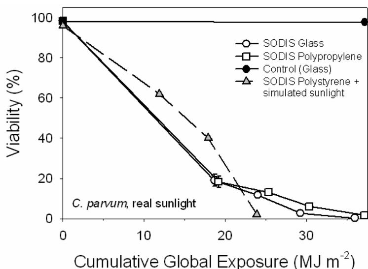
Figure 4.9 Comparison of solar inactivation of *C. parvum* oocyst suspensions in borosilicate glass and polypropilene bottles exposed to real sunlight
