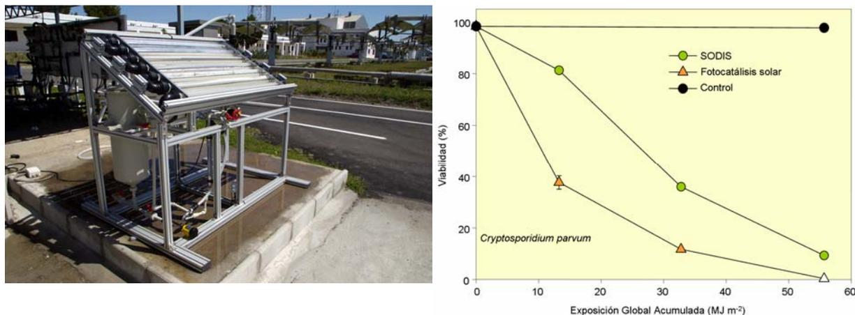
Figure 4.6 Solar photoreactor prototype for water disinfection (left). Degradation of *Cryptosporidium parvum* oocysts by SODIS and solar photocatalysis with supported TiO<sub>2</sub> under natural solar radiation at the Plataforma Solar de Almería (right, [4.4])
