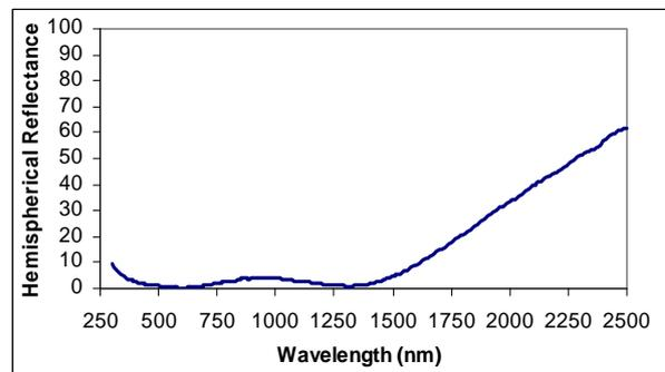
Figure 3.4 Hemispherical reflectance of the high-temperature absorbers
