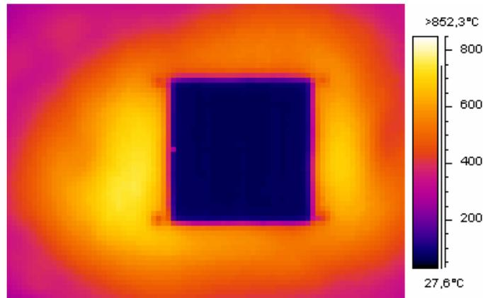
Figure 3.14 Thermogram of CCM surface temperature at 1 MW/m<sup>2</sup> concentration
