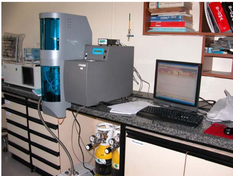
Figure 3.16 Thermogravimetry analysis system for analysis of materials subjected to the combined action of high temperatures and cycles in controlled atmosphere.
