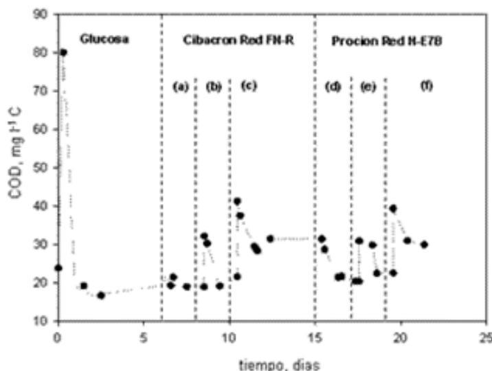
Figure 4.10 Operation of the bioreactor after photo-Fenton pretreatment. 250 mg l<sup>-1</sup> Cibacron Red FN-R with different H<sub>2</sub>O<sub>2</sub> doses (a) 250 mg l<sup>-1</sup>, (b) 225 mg l<sup>-1</sup>, (c) 200 mg l<sup>-1</sup>. 250 mg l<sup>-1</sup> Procion Red H-E7B with different H<sub>2</sub>O<sub>2</sub> doses (d) 80 mg l<sup>-1</sup> (e) 65 mg l<sup>-1</sup> (f) 50 mg l<sup>-1</sup>
