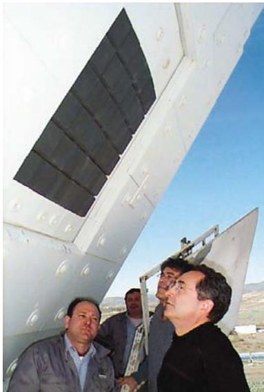
Figure 2.4 Front view of the 200-350-kW volumetric receiver test bed in the CRS tower
