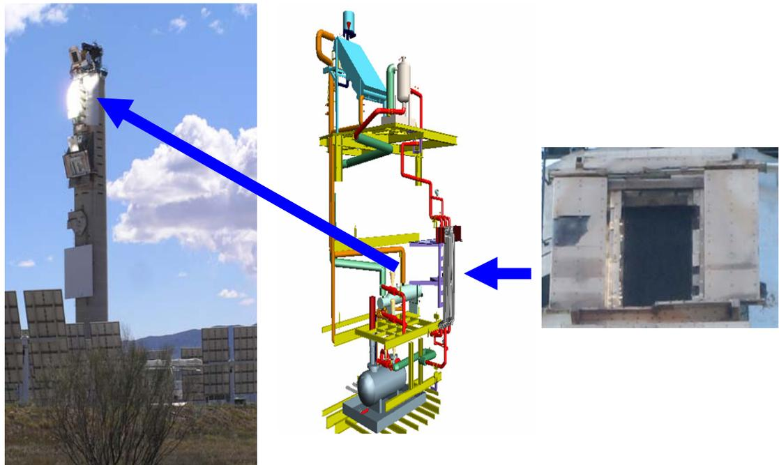
Figure 3.9 Salt Receiver Panel during testing at the 70-m level of the CESA-1 tower; diagram of the experimental device and front view of the receiver panel with side shielding.
