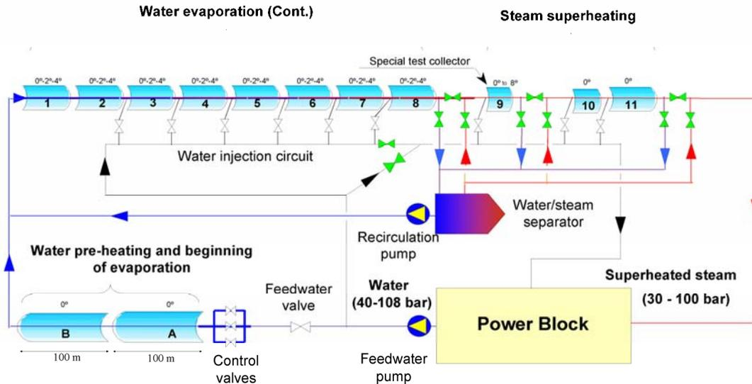
Figure 2.6 Simplified diagram of the PSA DISS plant
