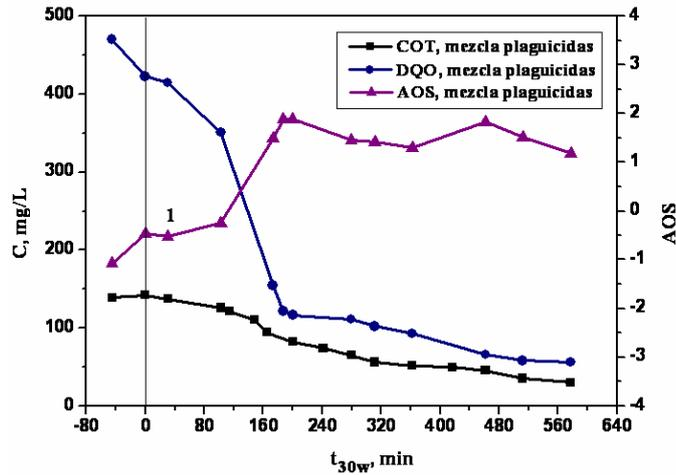
Figure 4.1 Degradation of a pesticide mixture (50 mg/L each) by foto-Fenton at 20 mg/L Fe<sub>2</sub><sup>+</sup>
