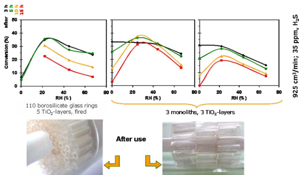
Figure 4.13 Conversion as a function of relative humidity, using glass rings and polymeric monoliths as  $TiO_2$  catalyst supports.
