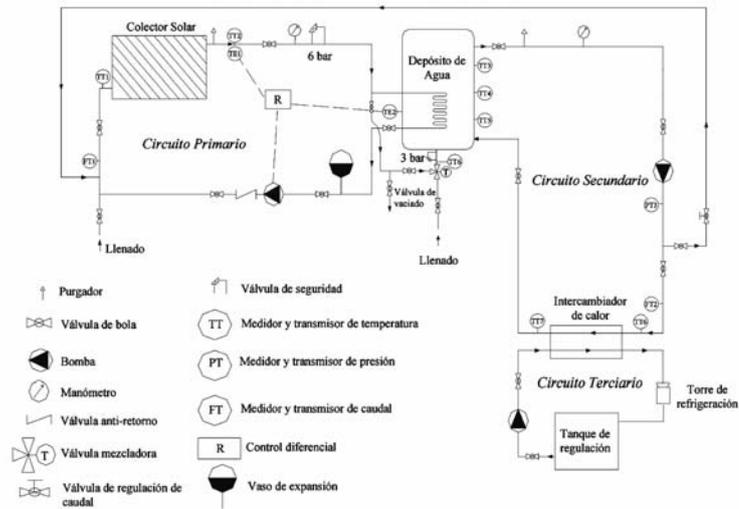
Figure 2.2 General diagram of the stationary solar collector test platform
