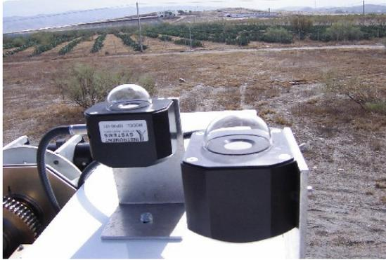
Figure 2.4 Spectroradiometer probes for measuring global and diffuse radiation installed in the solar tracker
