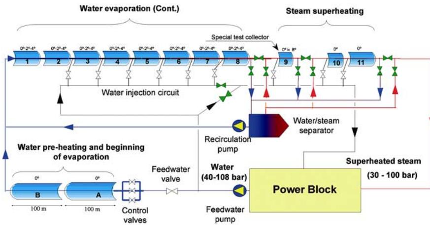
Figure 48. Schematic drawing of the DISS plant solar field after improvement of the solar field
