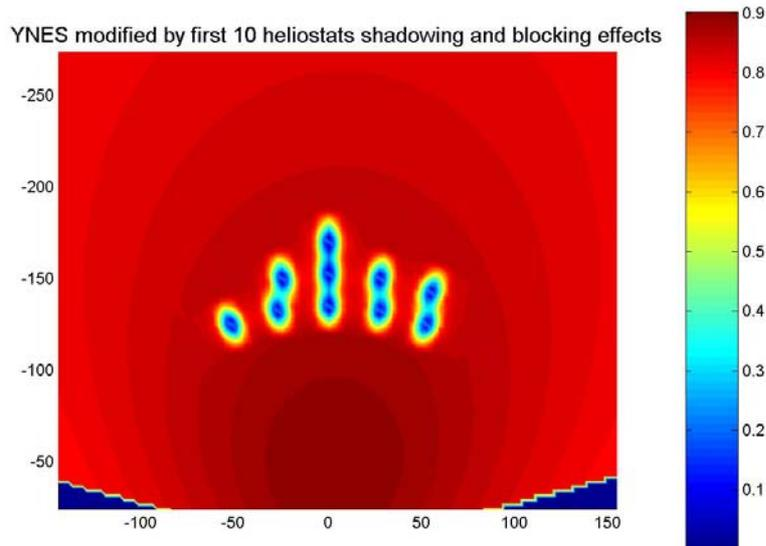
**Figure 44. Example of an YNES after being modified with the distribution of the first 10 heliostats. The blue spots represent shading and blocking caused. The coordinates are expressed in meters from the tower (0.0).**
