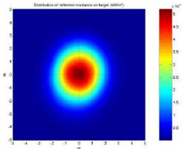
**Figure 35. Projection of the sun on the CESA-1 target by the Sanlúcar 120 heliostat (Day: 01/08/2003; Time: 12:30 UT)**
