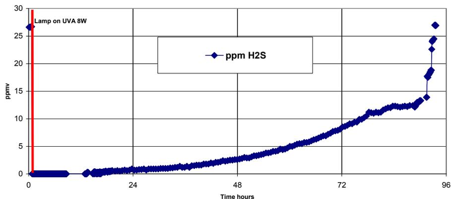
Figure 62. Destruction of 27 ppm<sub>v</sub> of H<sub>2</sub>S and its evolution over time
