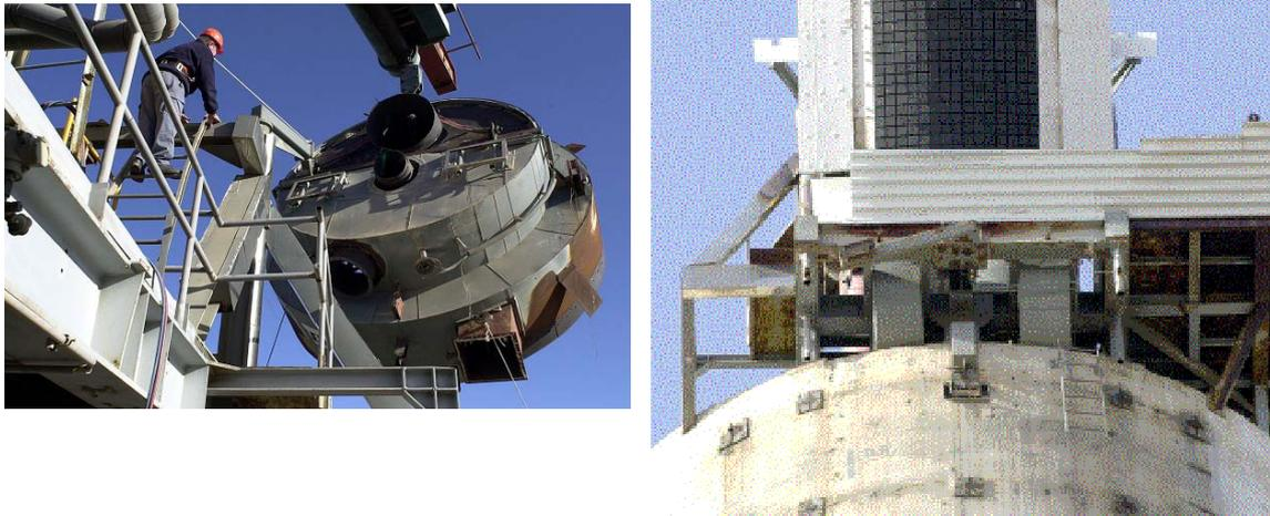
**Figure 40.** The metal absorber TSA receiver being lowered from the tower in March 2003 (left) and front view of the new Solair-3000 receiver in the CESA-I tower.
