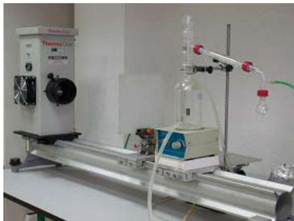
**Figure 26. Solar Chemistry Project test bed**
