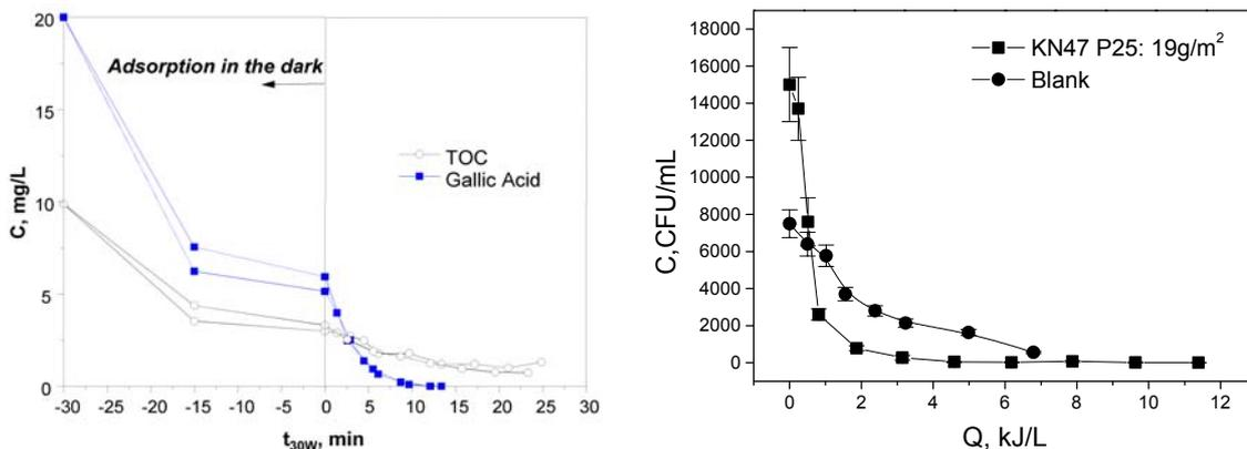
Figure 66. Left: Photocatalytic degradation of gallic acid with TiO<sub>2</sub> deposited on Ahlstrom type NW-10 paper (C<sub>0</sub>= 20 mg/L). Right: Deactivation of *E. Coli* con TiO<sub>2</sub> deposited on Ahlstrom type KN-47 paper (C<sub>0</sub>= 10<sup>4</sup> CFU/mL). Both carried out in a CPC solar reactor.
