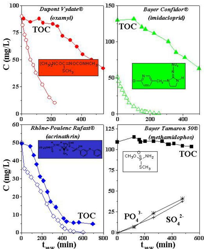
Figure 58. Photocatalytic degradation of four commercial pesticides widely used in greenhouse agriculture.
