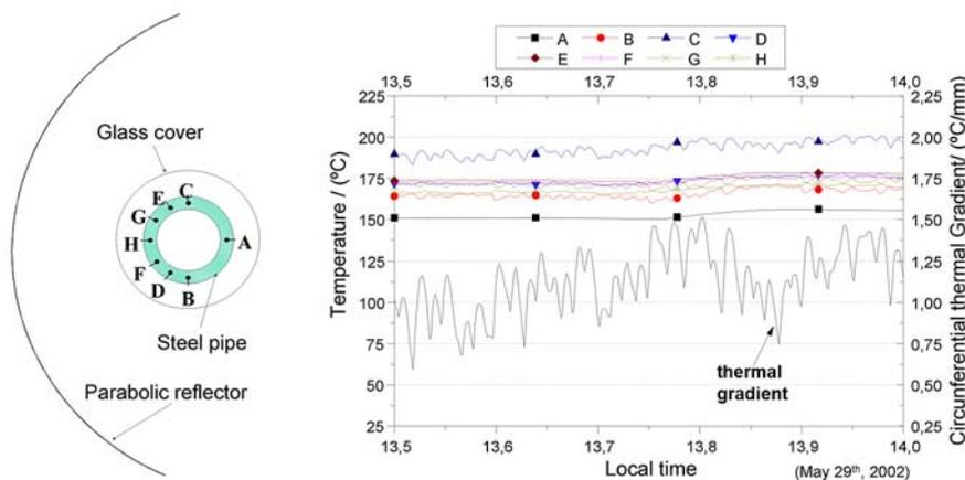
**Figure 52. Temperature profile and thermal gradient in the most unfavorable case found in the water pre-heat zone.**
