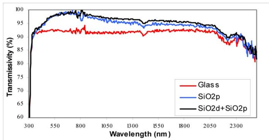
**Figure 51. Solar transmittance of borosilicate glass with no coating, with porous silica coating and with a dense silica and another porous layer.**
