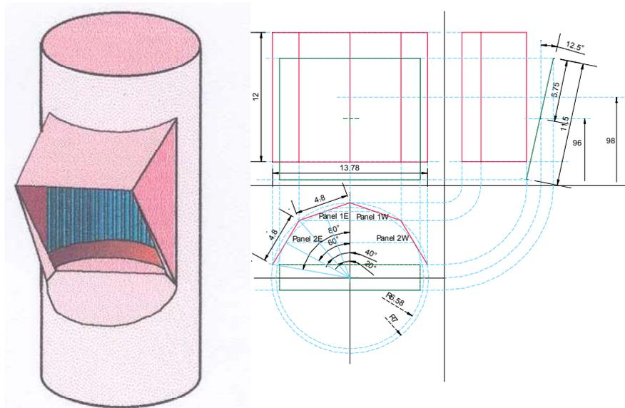
**Figure 34. Design of the cavity receiver with saturated steam**
