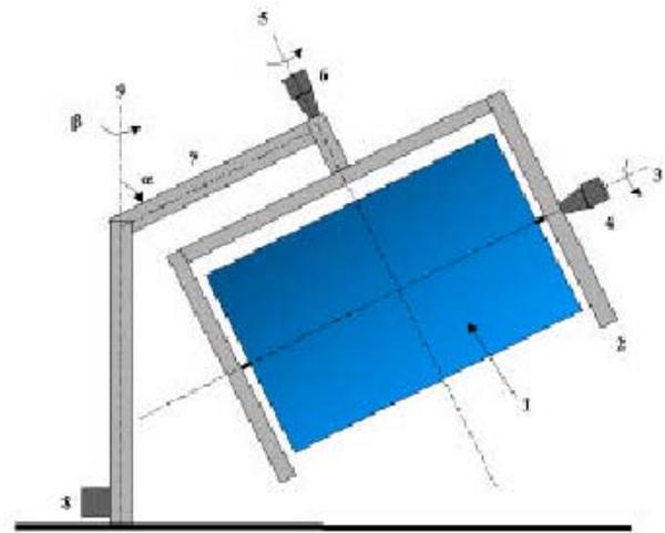
**Figure 37. Confined line-focusing cylindrical heliostat**
