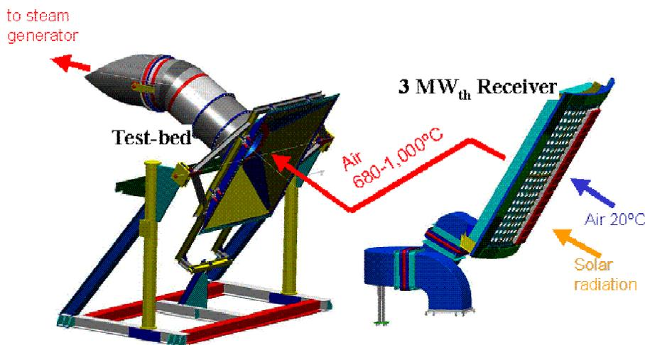
**Figure 41.** SOLAIR 3000 Test bed component parts showing solar radiation flux input
