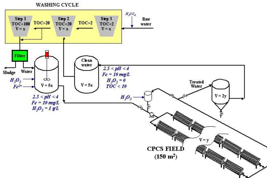
Figure 59. Schematic diagram of the container washing and photocatalytic water treatment plant concept
