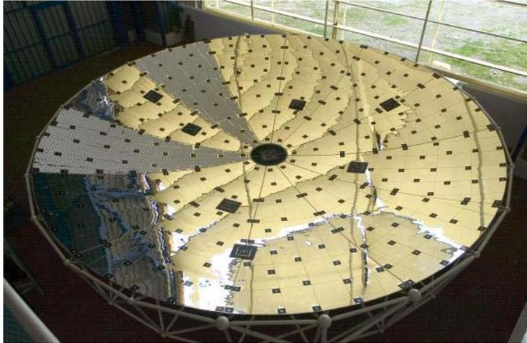
**Figure 23. New EUROdish parabolic concentrator**
