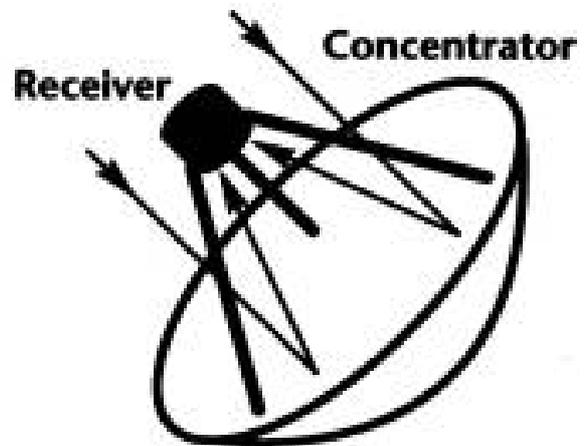
Figure 15. Schematic diagram of a parabolic dish with Stirling motor at the focus
