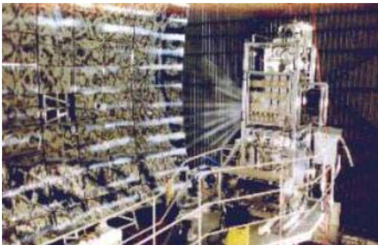
Figure 20. Solar Furnace: Concentrator (left) and receiver in operation at the focus (right).
