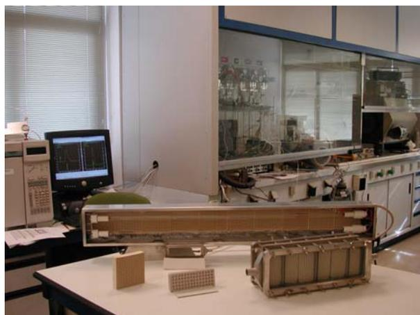
**Figure 27. Different types and configurations of reactors and catalysts—flat, monolithic, tubular—tested in gas phase.**
