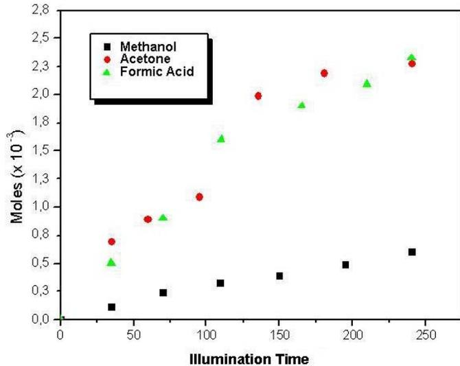
Figure 74. Formation of methanol, acetone and formic acid during the CO<sub>2</sub> reduction process. Experimental conditions: 100 ml/min CO<sub>2</sub>; pH = 1; TiO<sub>2</sub>-Ru (0.1%).
