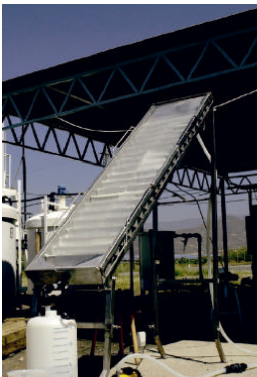
Cascade Photoreactor used to test titanium deposited on a fiber support prepared by the AHLSTROM PAPER company
