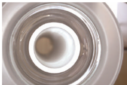
Tubular catalyst impregnated with \text{TiO}_2 and placed in the interior of a parabolic trough collector absorber tube. System configuration allows solar radiation to be used on the outside while UV lamps simultaneously irradiate the inner surface of the catalyst
