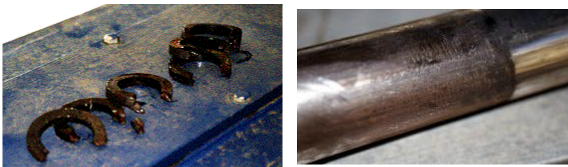
Recirculation pump packing and plunger after one of the frequent failures
