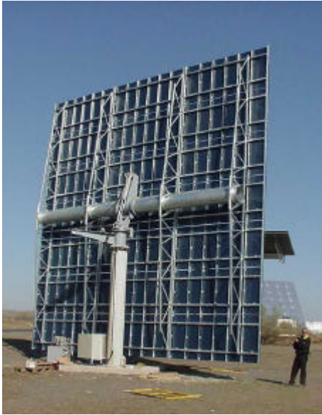
Rear view of the Sanlúcar heliostat with hydraulic driver installed at the PSA and flux distribution obtained at 380 m on a 12 x 12 m Lambertian target
