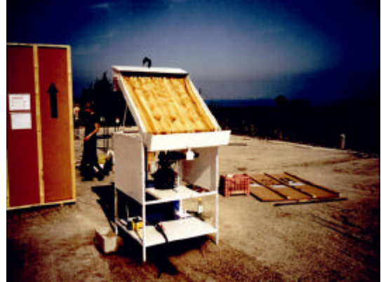
"Combined" photoreactor based on CPC collectors and UV lamps installed in a Portuguese olive mill (left) and "flat collector"-based photoreactor installed in a Greek olive mill (right)
