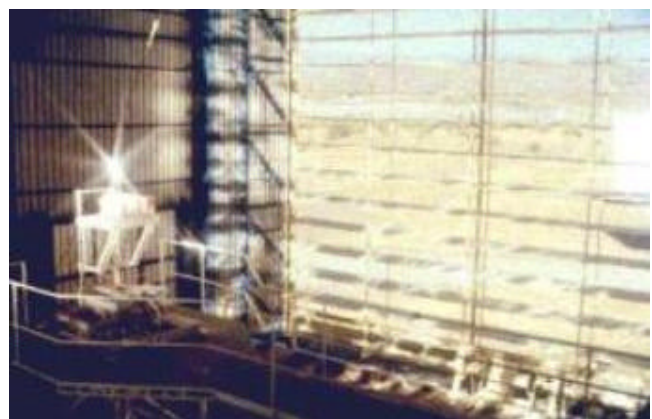
The focus and the test table on the left. On the right, the attenuator, completely open, allows the rays from the heliostats outside to enter.
