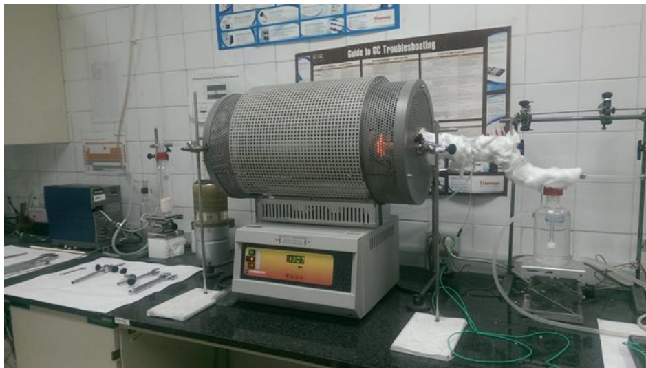
Figure 58. Indoor Solar Simulation Loop for evaluation of materials for thermochemical cycles.
