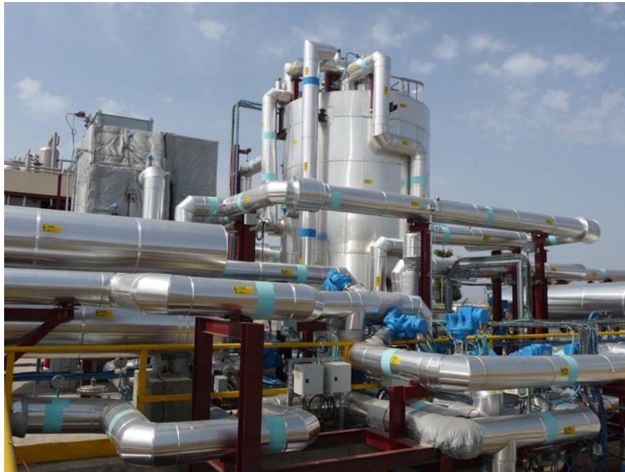
Figure 26. Molten Salt Test Loop (MOSA) for Thermal Energy Systems.
