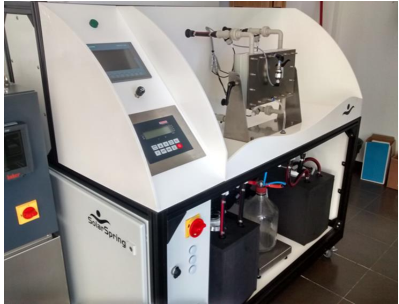
Figure 33. Bench-scale unit for testing MD with flat-sheet membranes.
