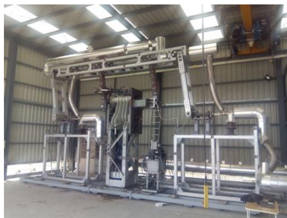
Figure 13. Schematic diagram of the REPA test loop at PSA (a) and north view of the test facility (b).
