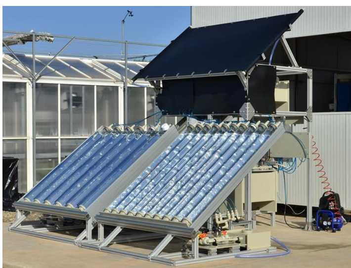
Figure 37. View of new CPC and U-type photoreactors (NOVA 75 V 1.0).
