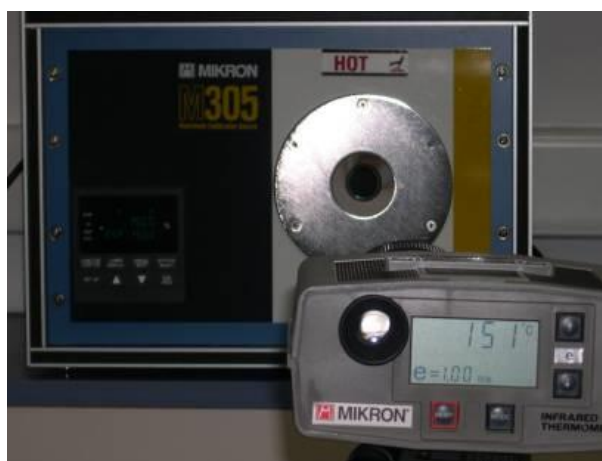
Figure 48. IR sensor calibration using a black body.
