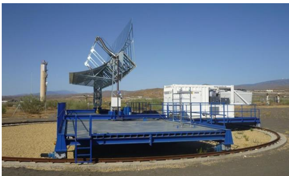
Figure 12. Side view of KONTAS test bench and the heating cooling unit.
