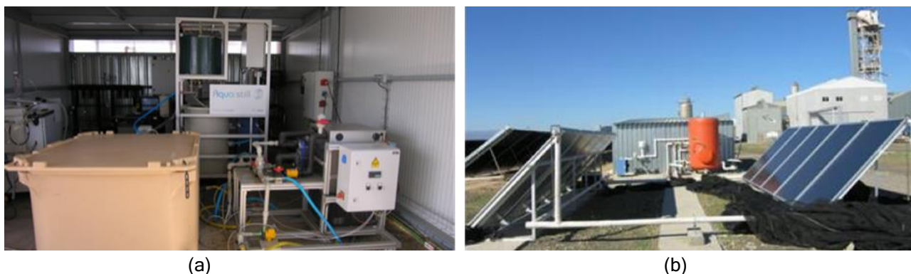
Figure 31. Internal (a) and external (b) views of the Membrane Distillation experimental test bed within the PSA low-temperature solar thermal desalination facility.
