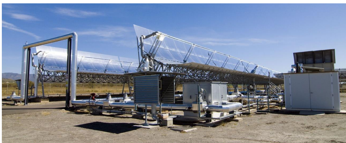
Figure 10. View of the IFL experimental facility (with parabolic-troughs) using compressed gas as heat transfer fluid.
