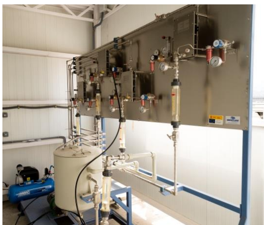
Figure 36. Electro-Fenton pilot plant coupled with a 2 m 2 CPC (ELECTROX).
