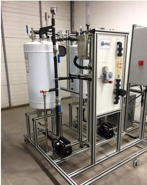
Figure 32. Bench-scale unit for testing membranes on isobaric MD.
