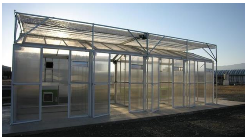
Figure 42. Cultivation chamber for wastewater crops irrigation reuse at PSA facilities.
